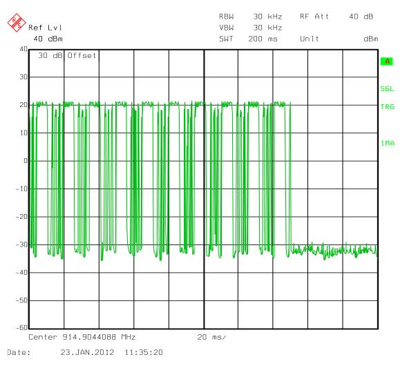
30 Short pulses @ 0.841 ms 10 Long pulses @ 6.9 ms Time per hop = 0.58 seconds
