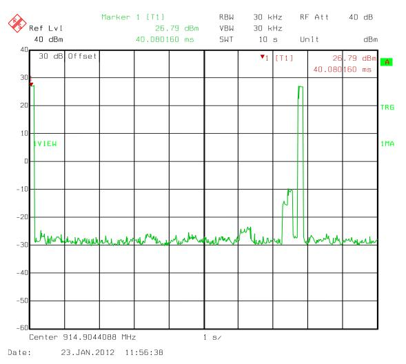
Hopping on 51 Channels Total ON time =116 ms in 10 seconds
