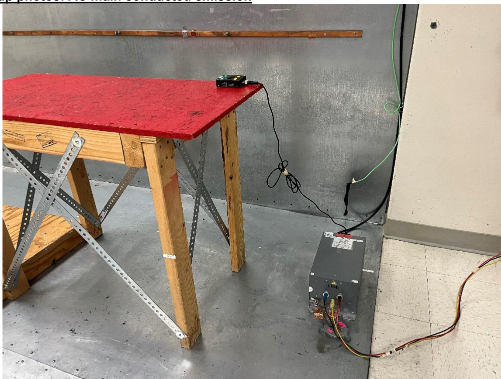
Photo 11: Test setup for AC main conducted emission
