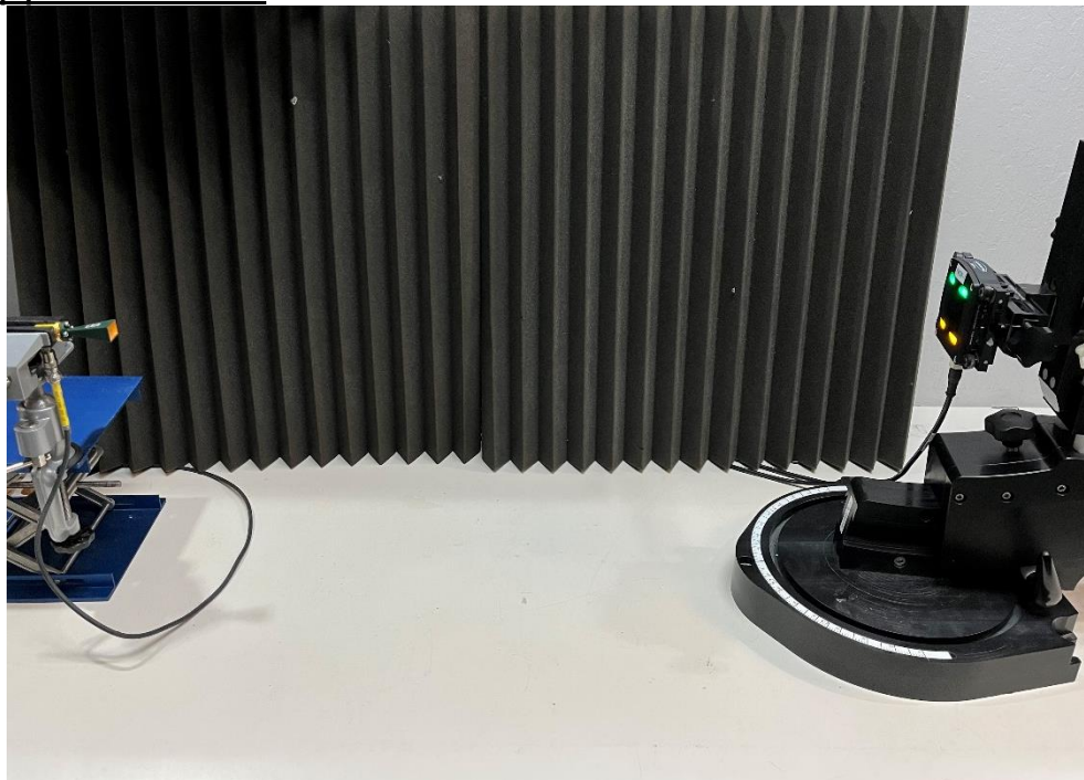
Photo 7: Test setup for step 1: measuring the main beam of the EUT with RF detector and DSO.
