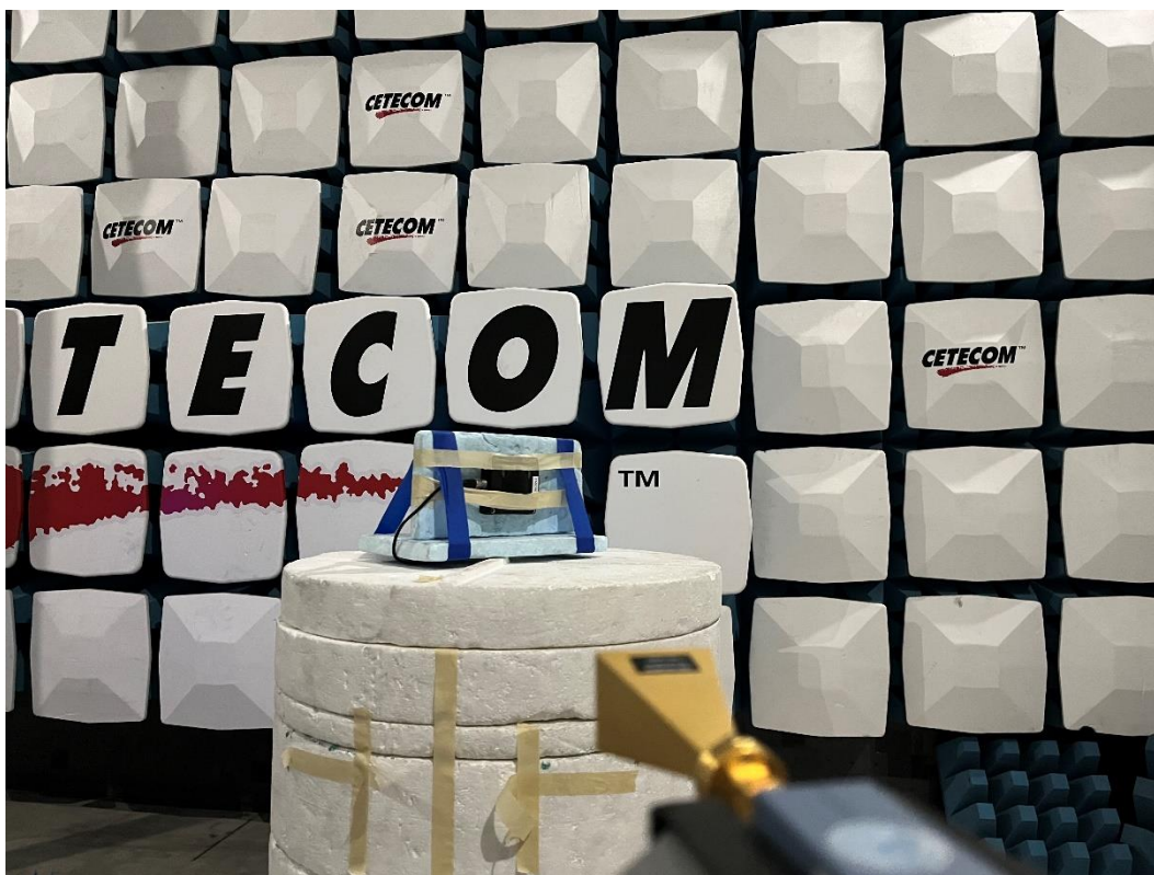
Photo 6: Emissions in frequency range 50-75 GHz (for other frequency ranges above 40 GHz, other external mixer and antenna are applied)
