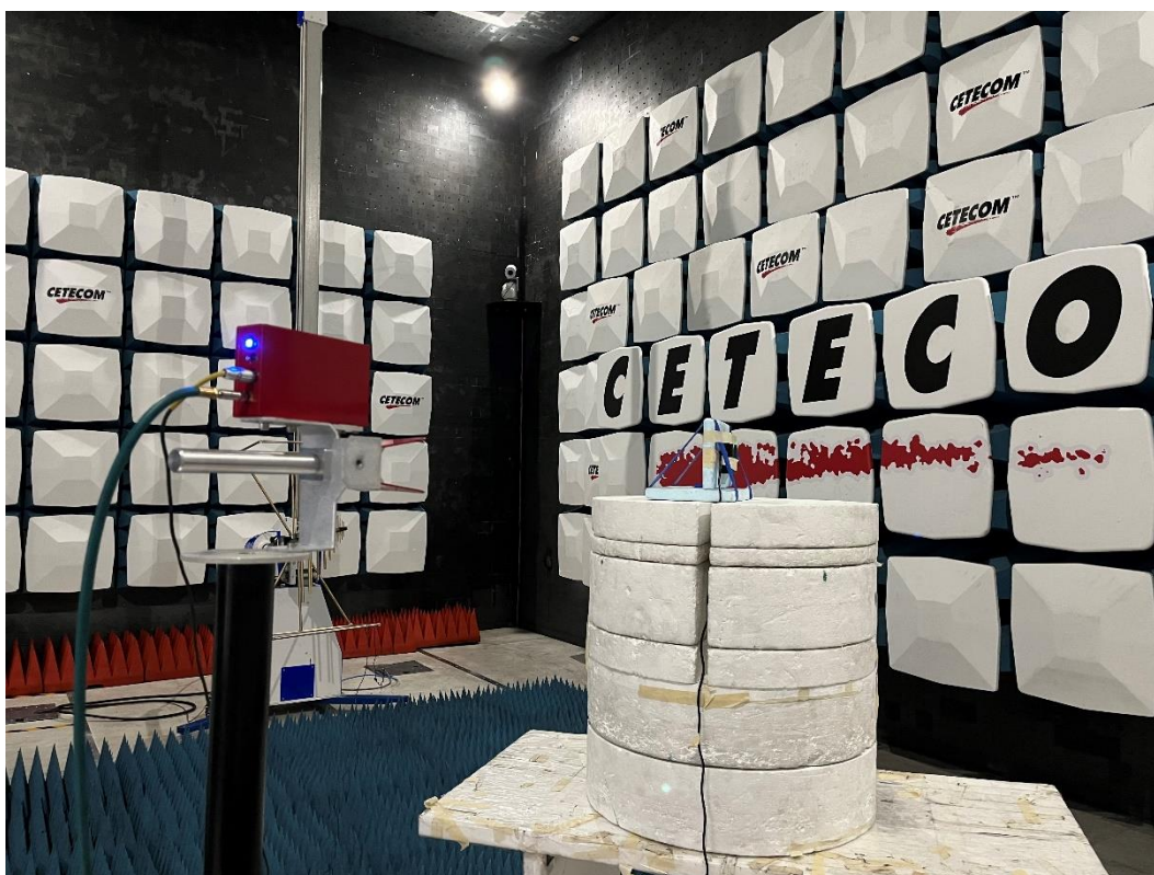
Photo 5: Emissions in frequency range 18-40 GHz
