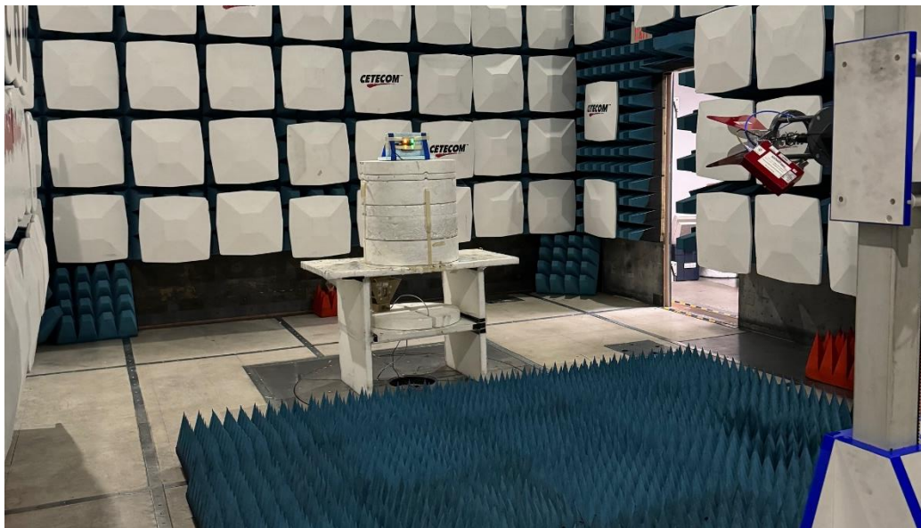
Photo 4: Emissions in frequency range 3-18 GHz
