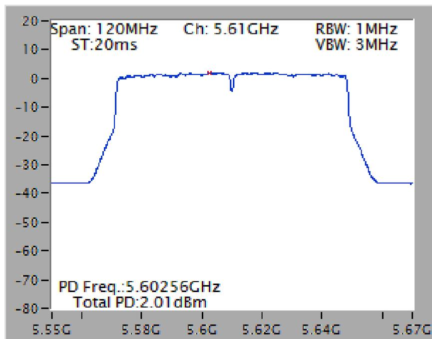
Power Density Plot on Configuration IEEE 802.11ac MCS0/Nss3 VHT20 / Chain 1 + Chain 2 + Chain 3 + Chain 4 / 5260 MHz
