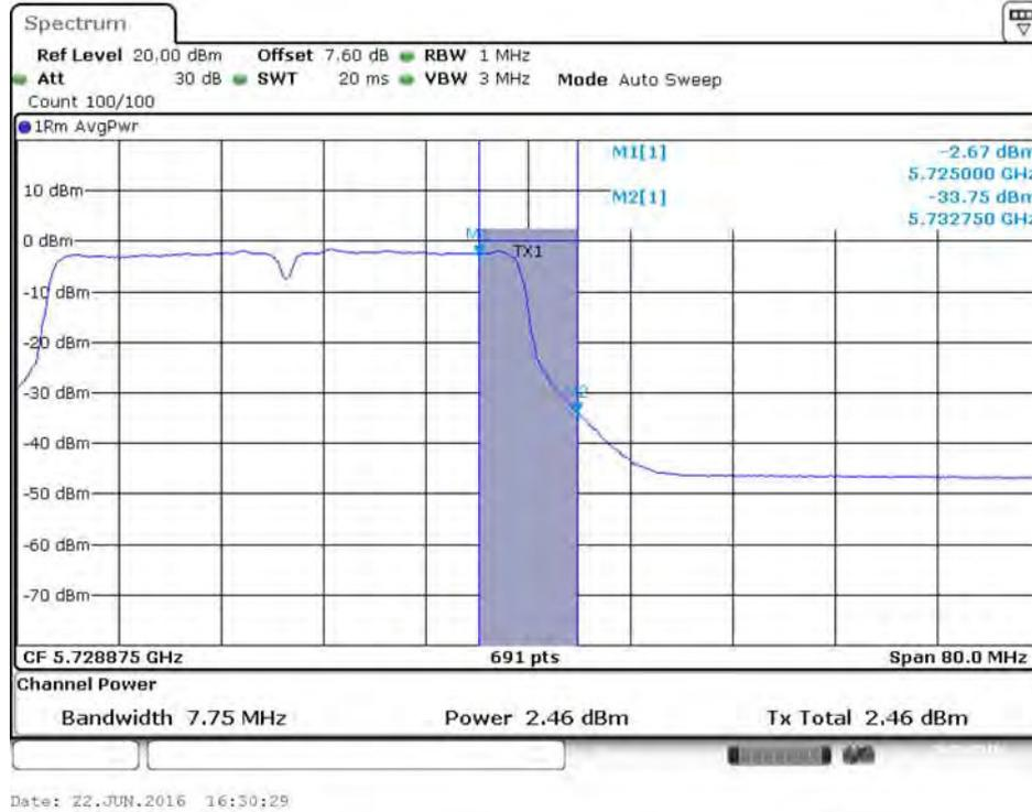
**Conducted Output Power Plot on Configuration IEEE 802.11ac MCS0/Nss3 VHT40 / Chain 2 / 5710 MHz (UNII 3)**
