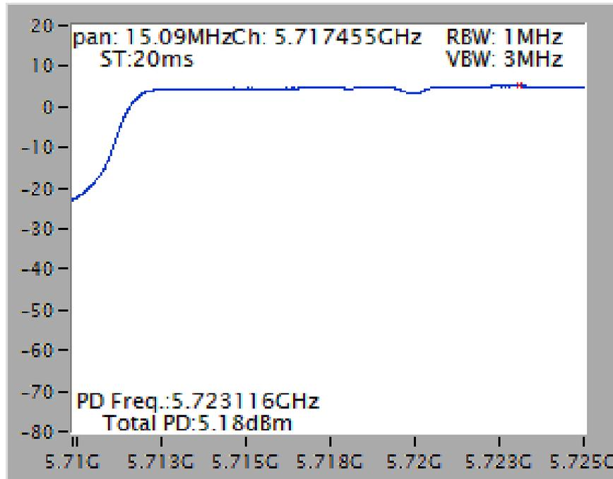
Power Density Plot on Configuration IEEE 802.11a / Chain 1 + Chain 2 + Chain 3 + Chain 4 / 5720 MHz
