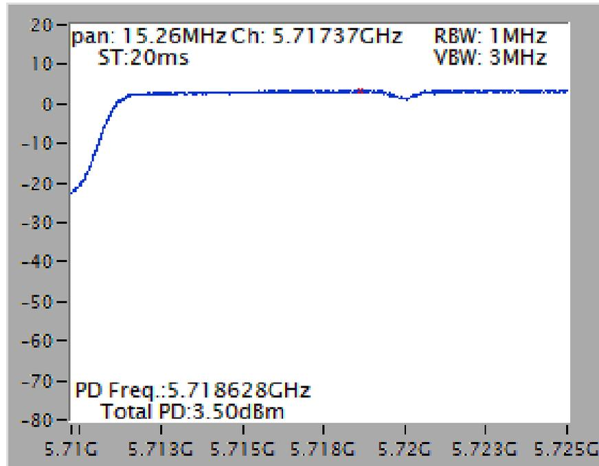
Power Density Plot on Configuration IEEE 802.11ac MCS0/Nss2 VHT20 / Chain 1 + Chain 2 + Chain 3 + Chain 4 / 5720 MHz (UNII 3)
