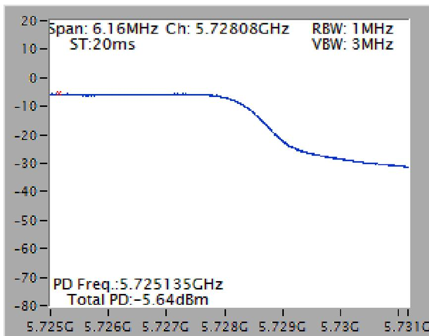
Power Density Plot on Configuration IEEE 802.11ac MCS0/Nss2 VHT20 / Chain 1 + Chain 2 + Chain 3 + Chain 4 / 5720 MHz (UNII 2C)
