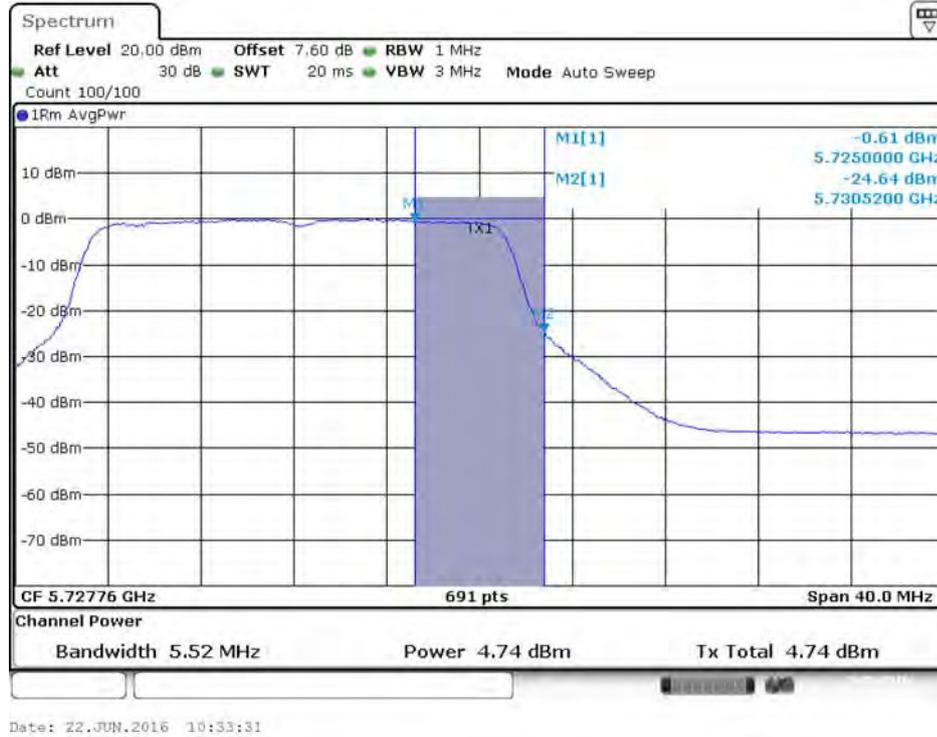
**Conducted Output Power Plot on Configuration IEEE 802.11ac MCS0/Nss3 VHT20 / Chain 2 / 5720 MHz (UNII 3)**
