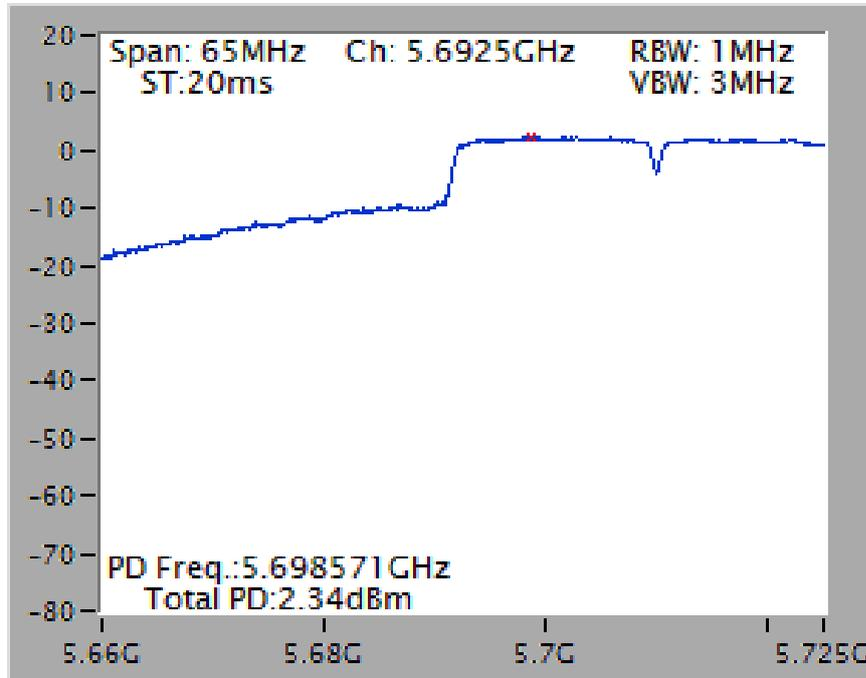
Power Density Plot on Configuration IEEE 802.11ac MCS0/Nss1 VHT40 / Chain 5 / 5710 MHz (UNII 3)
