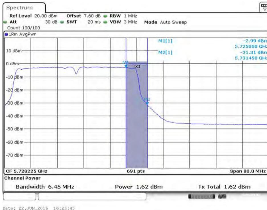
**Conducted Output Power Plot on Configuration IEEE 802.11ac MCS0/Nss3 VHT80 / Chain 1 / 5690 MHz (UNII 2C)**
