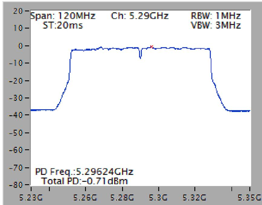
Power Density Plot on Configuration IEEE 802.11ac MCS0/Nss1 VHT80 / Chain 1 + Chain 2 + Chain 3 + Chain 4 / 5530 MHz
