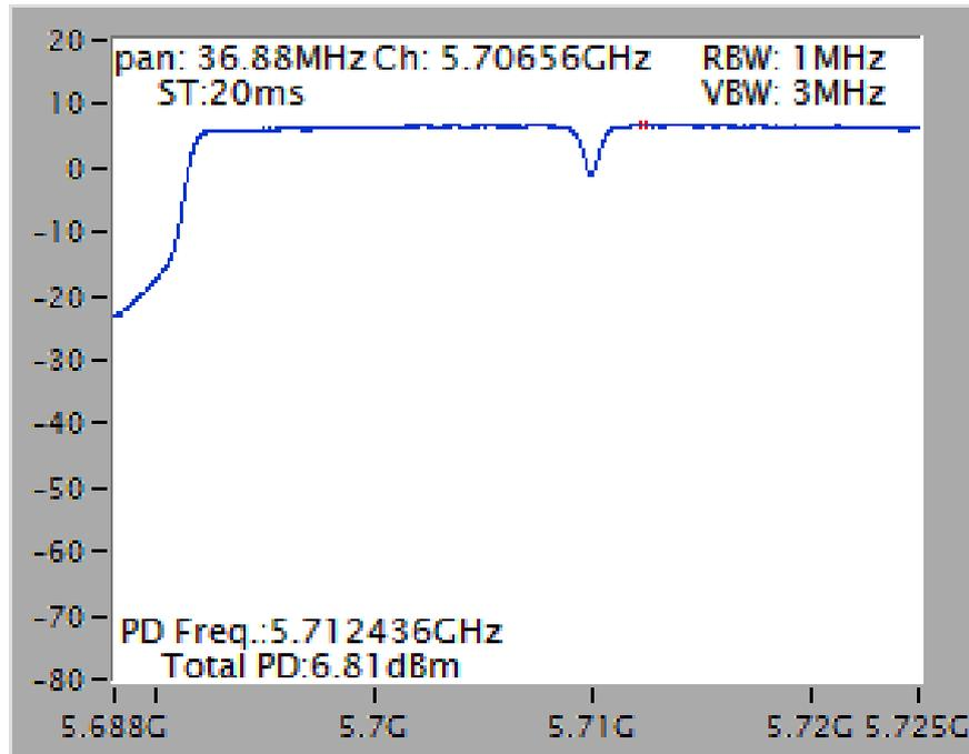
Power Density Plot on Configuration IEEE 802.11ac MCS0/Nss3 VHT40 / Chain 1 + Chain 2 + Chain 3 + Chain 4 / 5710 MHz (UNII 3)
