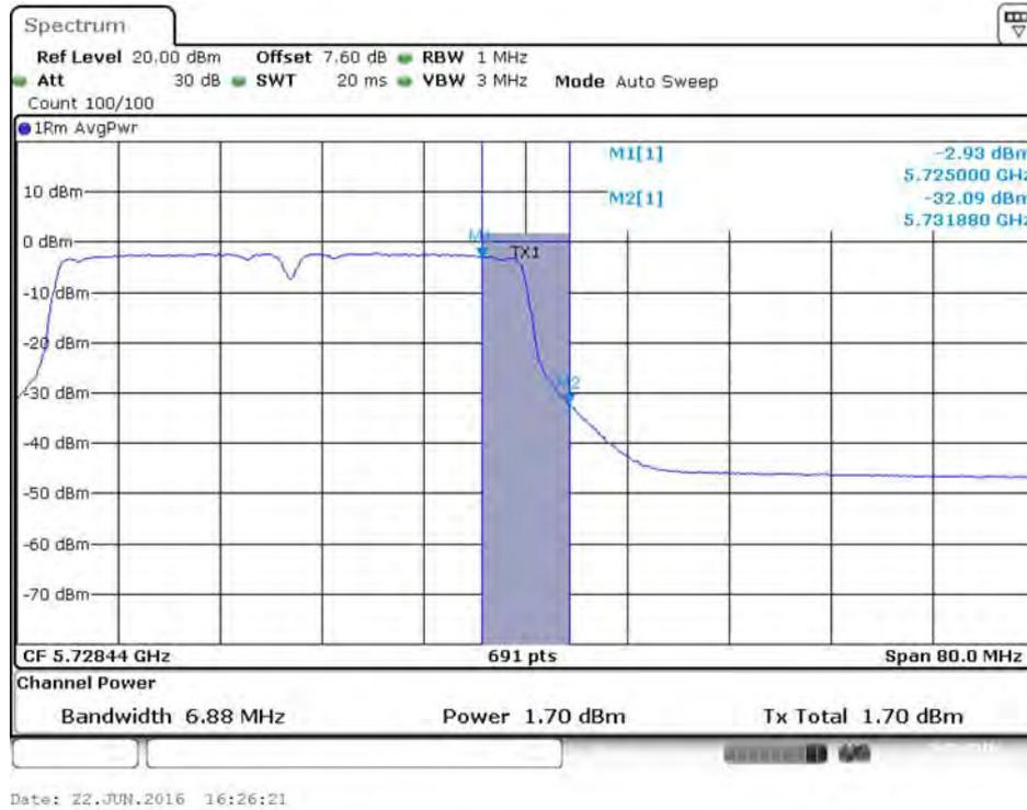
**Conducted Output Power Plot on Configuration IEEE 802.11ac MCS0/Nss3 VHT40 / Chain 4 / 5710 MHz (UNII 3)**
