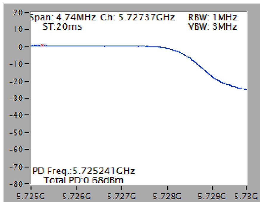
Power Density Plot on Configuration IEEE 802.11ac MCS0/Nss1 VHT20 / Chain 1 + Chain 2 + Chain 3 + Chain 4 / 5720 MHz (UNII 2C)
