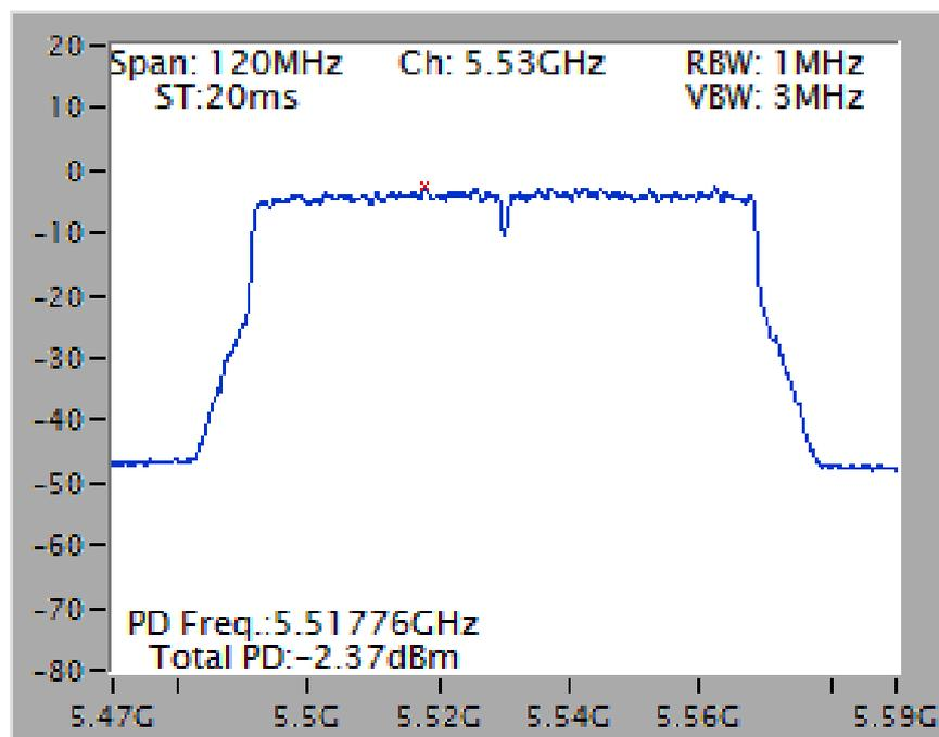
Power Density Plot on Configuration IEEE 802.11ac MCS0/Nss3 VHT20 / Chain 1 + Chain 2 + Chain 3 + Chain 4 / 5300 MHz
