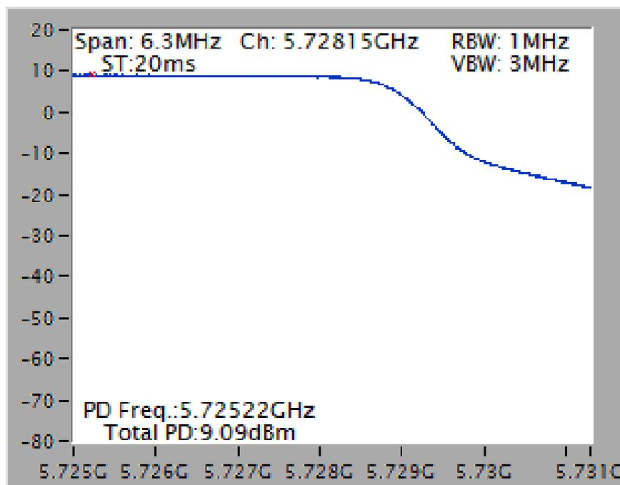
Power Density Plot on Configuration IEEE 802.11ac MCS0/Nss3 VHT40 / Chain 1 + Chain 2 + Chain 3 + Chain 4 / 5710 MHz (UNII 2C)
