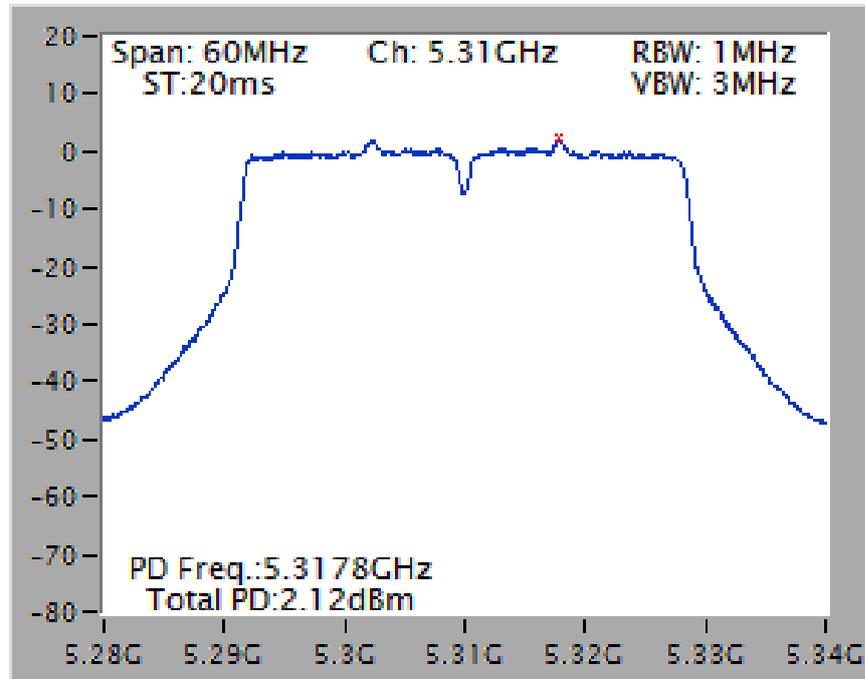
Power Density Plot on Configuration IEEE 802.11ac MCS0/Nss3 VHT40 / Chain 1 + Chain 2 + Chain 3 + Chain 4 / 5550 MHz
