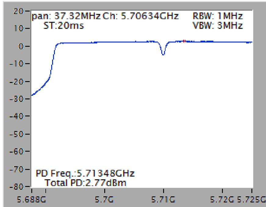
Power Density Plot on Configuration IEEE 802.11ac MCS0/Nss4 VHT40 / Chain 1 + Chain 2 + Chain 3 + Chain 4 / 5710 MHz (UNII 3)
