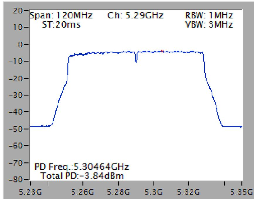
Power Density Plot on Chain 3 + Chain 4 / 5530 MHz
