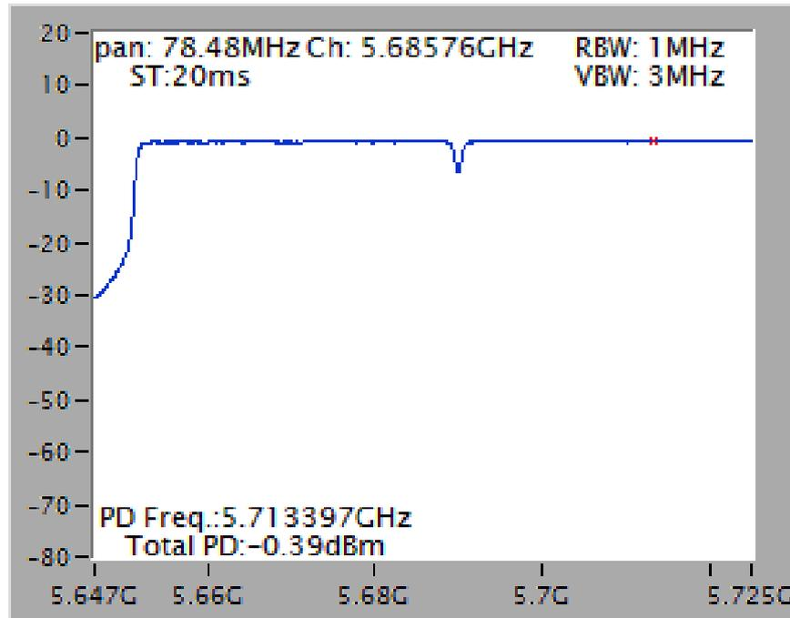
Power Density Plot on Configuration IEEE 802.11ac MCS0/Nss4 VHT80 / Chain 1 + Chain 2 + Chain 3 + Chain 4 / 5690 MHz (UNII 3)
