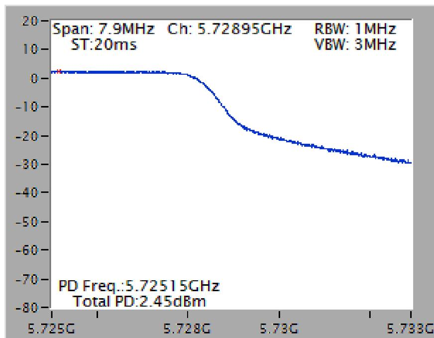
Power Density Plot on Configuration IEEE 802.11ac MCS0/Nss4 VHT80 / Chain 1 + Chain 2 + Chain 3 + Chain 4 / 5690 MHz (UNII 2C)
