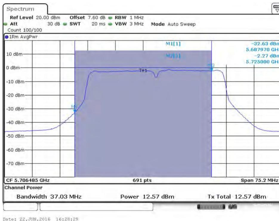
**Conducted Output Power Plot on Configuration IEEE 802.11ac MCS0/Nss3 VHT40 / Chain 3 / 5710 MHz (UNII 2C)**
