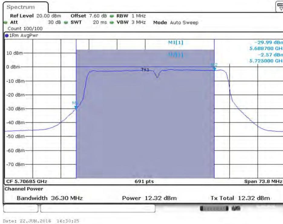
**Conducted Output Power Plot on Configuration IEEE 802.11ac MCS0/Nss3 VHT40 / Chain 2 / 5710 MHz (UNII 2C)**
