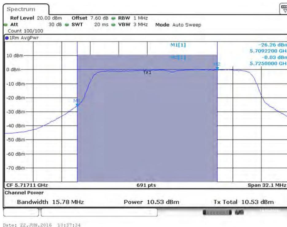
**Conducted Output Power Plot on Configuration IEEE 802.11ac MCS0/Nss3 VHT20 / Chain 3 / 5720 MHz (UNII 2C)**
