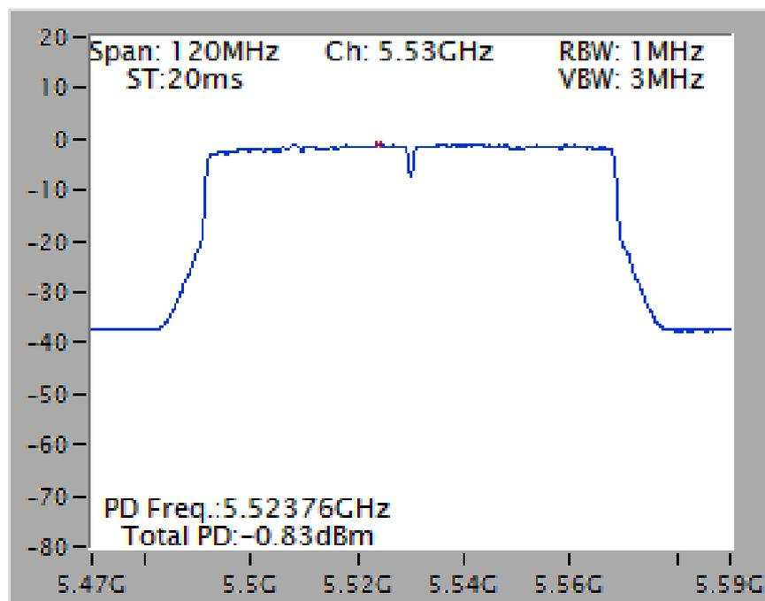
Power Density Plot on Configuration IEEE 802.11ac MCS0/Nss2 VHT20 / Chain 1 + Chain 2 + Chain 3 + Chain 4 / 5300 MHz
