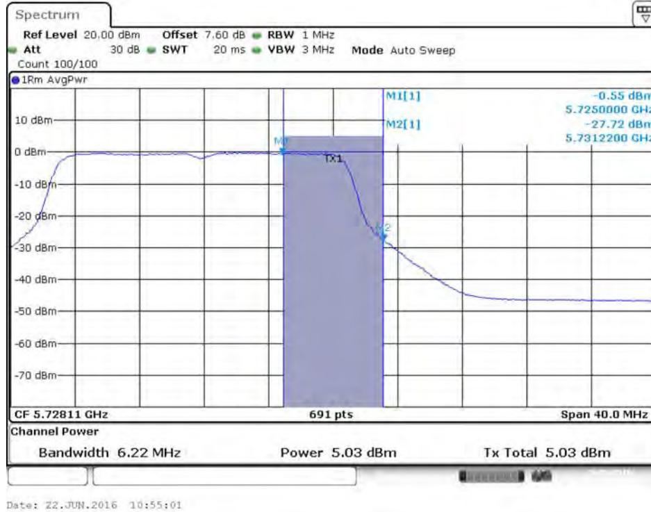
**Conducted Output Power Plot on Configuration IEEE 802.11ac MCS0/Nss3 VHT20 / Chain 4 / 5720 MHz (UNII 3)**
