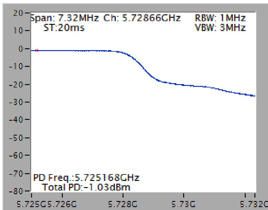
Power Density Plot on Configuration IEEE 802.11ac MCS0/Nss4 VHT20 / Chain 1 + Chain 2 + Chain 3 + Chain 4 / 5720 MHz (UNII 2C)
