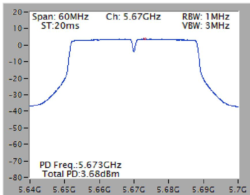
Power Density Plot on Configuration IEEE 802.11ac MCS0/Nss4 VHT80 / Chain 1 + Chain 2 + Chain 3 + Chain 4 / 5290 MHz
