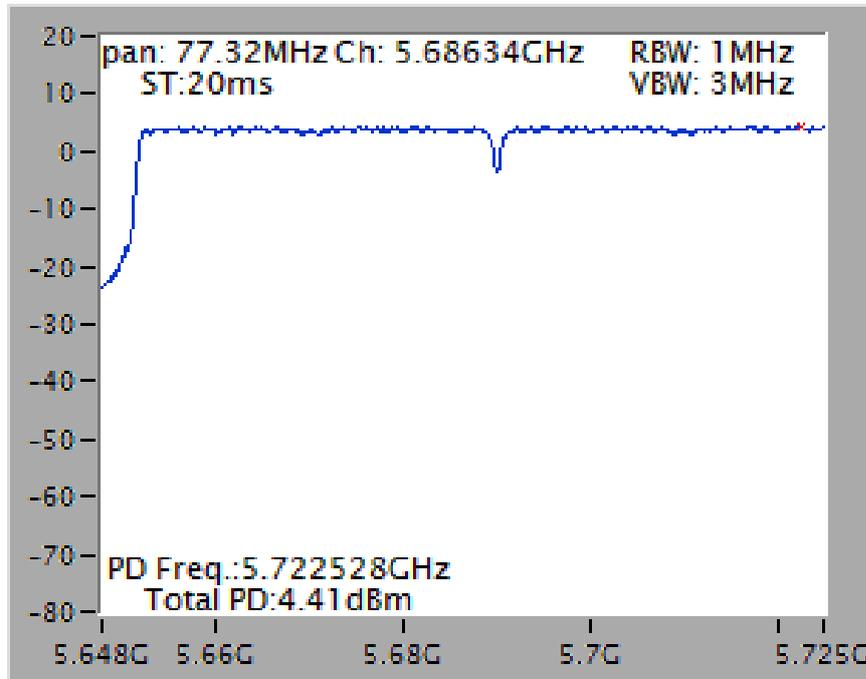
Power Density Plot on Configuration IEEE 802.11ac MCS0/Nss3 VHT80 / Chain 1 + Chain 2 + Chain 3 + Chain 4 / 5690 MHz (UNII 3)
