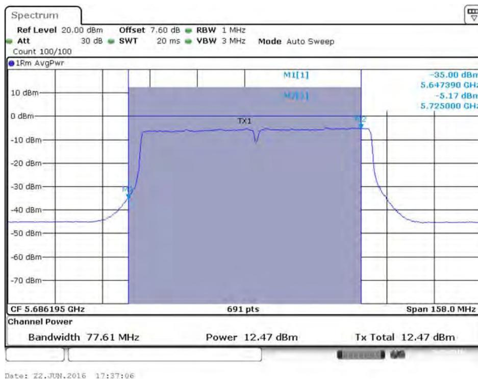
**Conducted Output Power Plot on Configuration IEEE 802.11ac MCS0/Nss3 VHT80 / Chain 3 / 5690 MHz (UNII 2C)**
