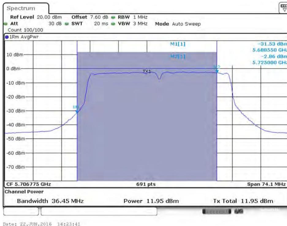
**Conducted Output Power Plot on Configuration IEEE 802.11ac MCS0/Nss3 VHT40 / Chain 1 / 5710 MHz (UNII 3)**
