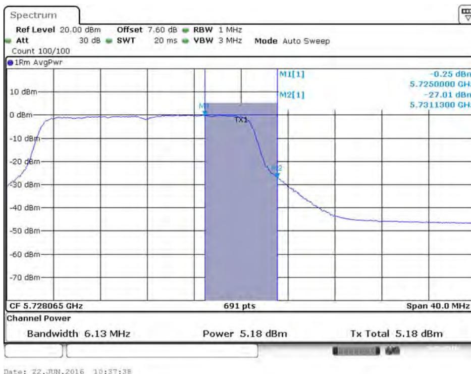
**Conducted Output Power Plot on Configuration IEEE 802.11ac MCS0/Nss3 VHT20 / Chain 3 / 5720 MHz (UNII 3)**
