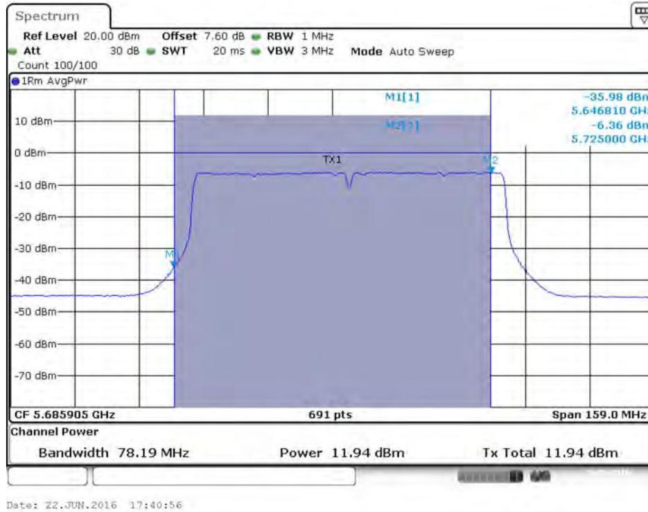
**Conducted Output Power Plot on Configuration IEEE 802.11ac MCS0/Nss3 VHT80 / Chain 4 / 5690 MHz (UNII 2C)**
