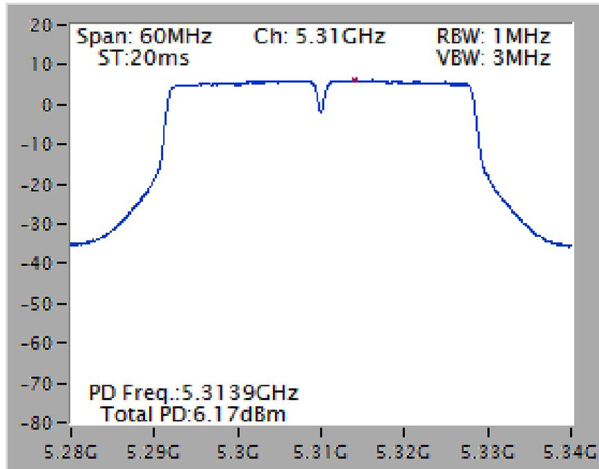
Power Density Plot on Configuration IEEE 802.11ac MCS0/Nss3 VHT40 / Chain 1 + Chain 2 + Chain 3 + Chain 4 / 5510 MHz
