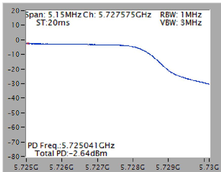
Power Density Plot on Configuration IEEE 802.11ac MCS0/Nss1 VHT80 / Chain 1 + Chain 2 + Chain 3 + Chain 4 / 5690 MHz (UNII 2C)
