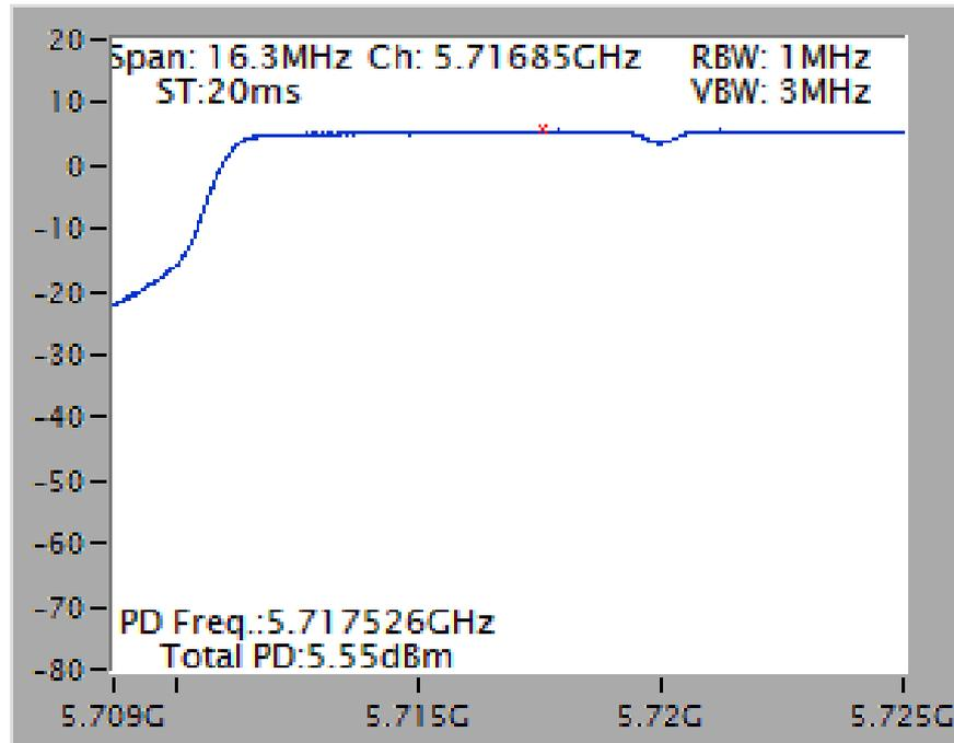
Power Density Plot on Configuration IEEE 802.11ac MCS0/Nss4 VHT20 / Chain 1 + Chain 2 + Chain 3 + Chain 4 / 5720 MHz (UNII 3)
