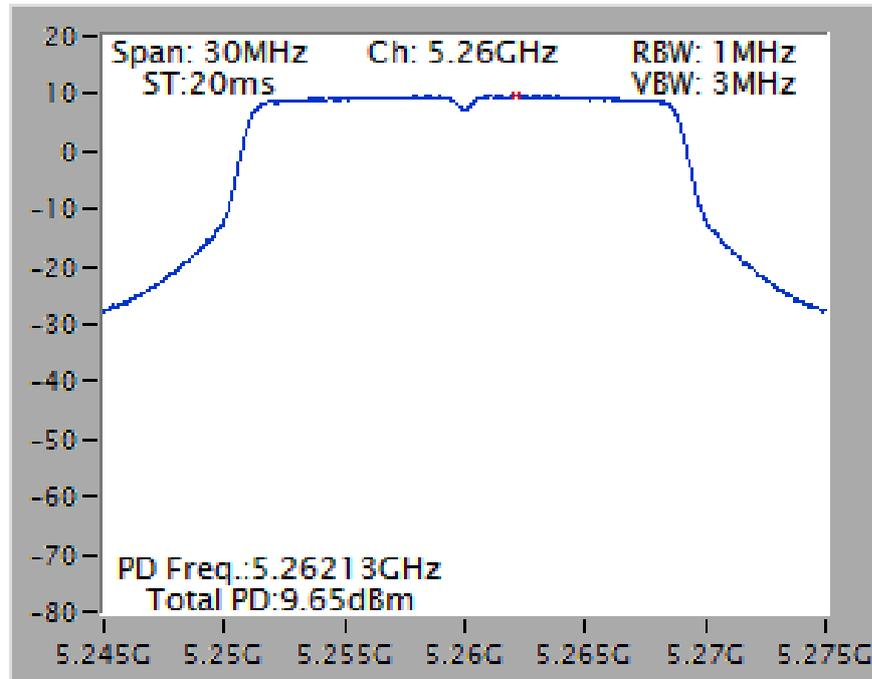
Power Density Plot on Configuration IEEE 802.11ac MCS0/Nss3 VHT20 / Chain 1 + Chain 2 + Chain 3 + Chain 4 / 5500 MHz
