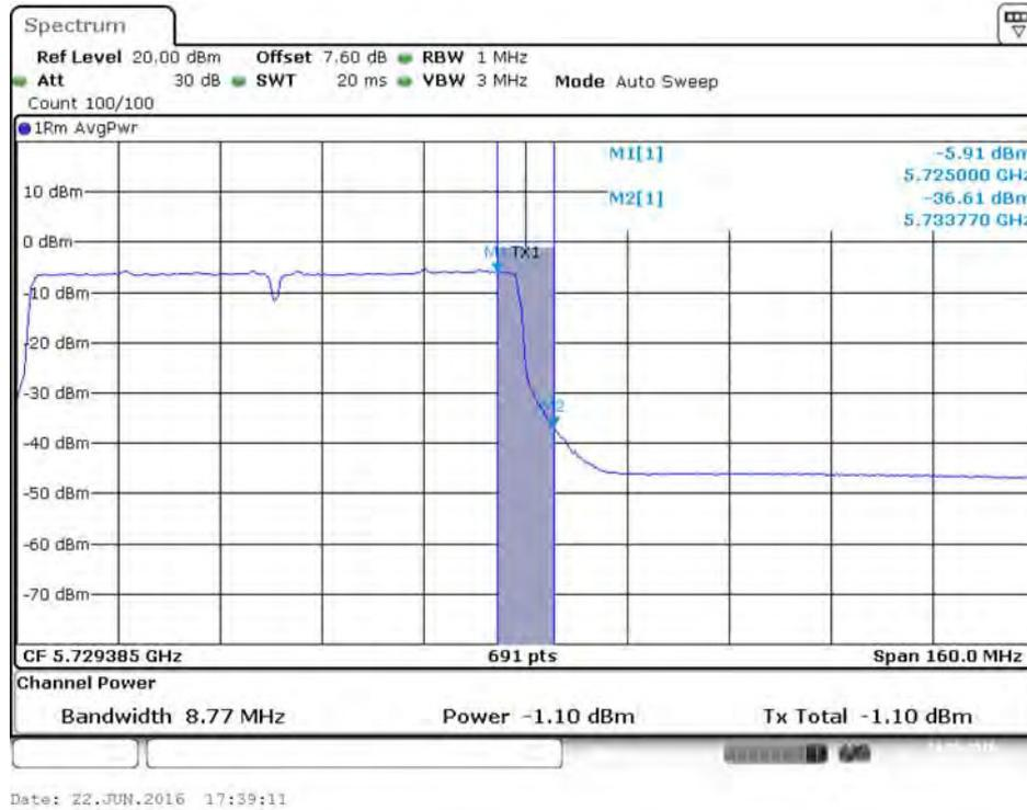
**Conducted Output Power Plot on Configuration IEEE 802.11ac MCS0/Nss3 VHT80 / Chain 2 / 5690 MHz (UNII 3)**
