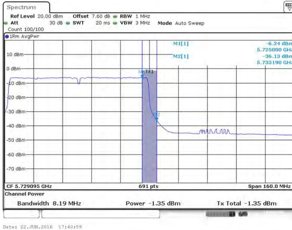
**Conducted Output Power Plot on Configuration IEEE 802.11ac MCS0/Nss3 VHT80 / Chain 4 / 5690 MHz (UNII 3)**
