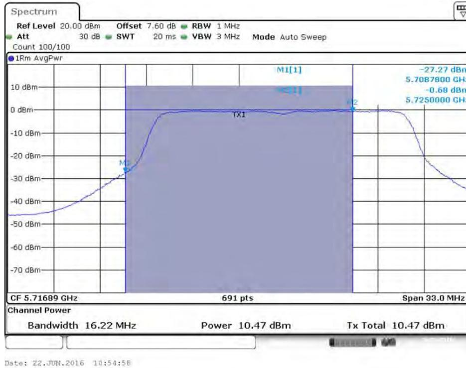
**Conducted Output Power Plot on Configuration IEEE 802.11ac MCS0/Nss3 VHT20 / Chain 4 / 5720 MHz (UNII 2C)**
