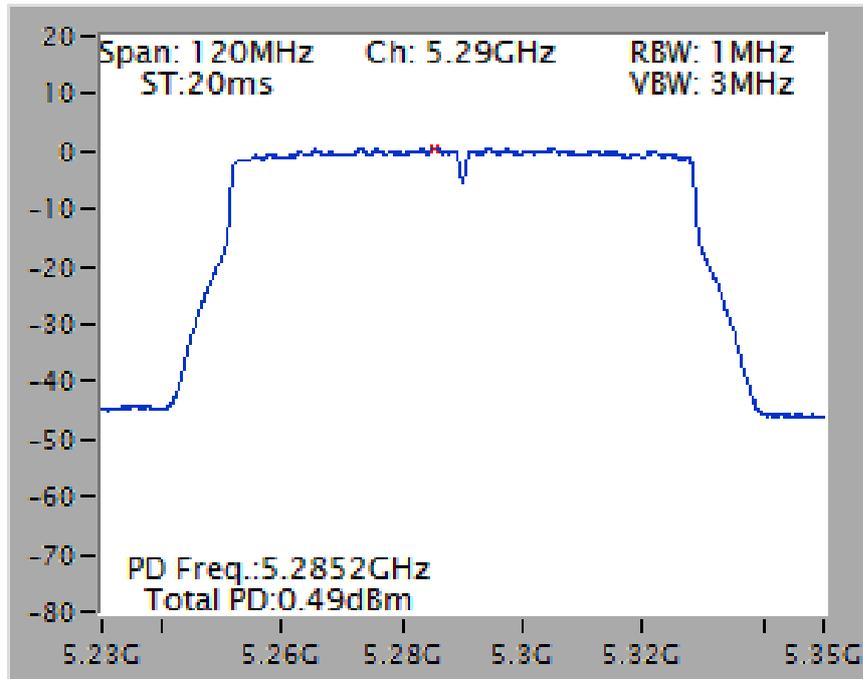
Power Density Plot on Chain 3 + Chain 4 / 5610 MHz
