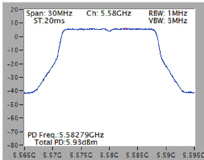
Power Density Plot on Configuration IEEE 802.11ac MCS0/Nss1 VHT20 / Chain 1 + Chain 2 + Chain 3 + Chain 4 / 5300 MHz
