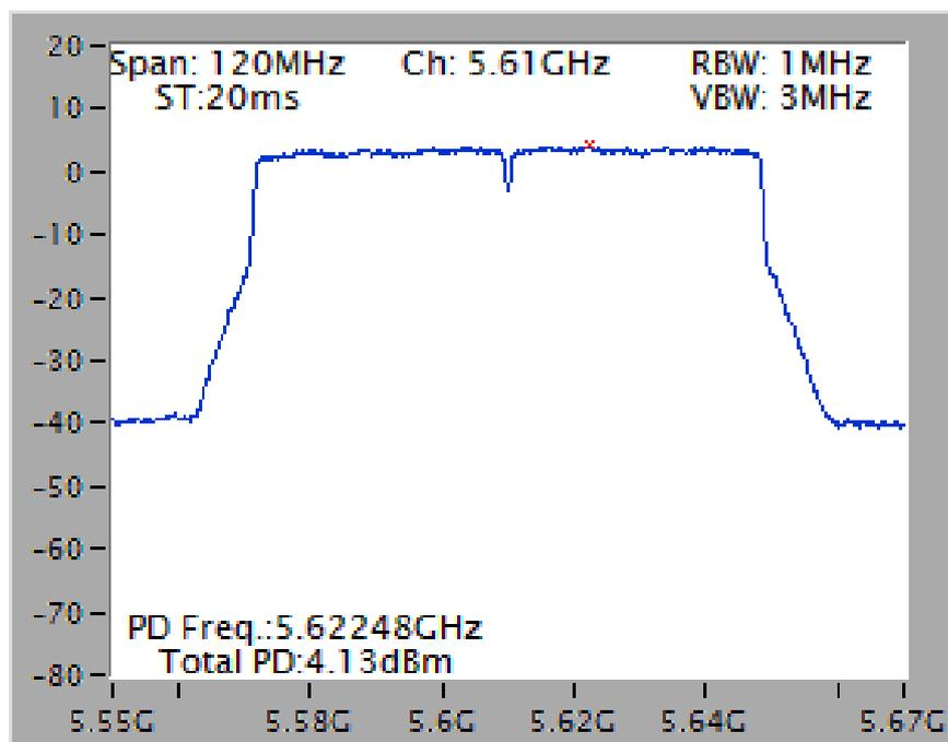
Power Density Plot on Configuration IEEE 802.11ac MCS0/Nss4 VHT20 / Chain 1 + Chain 2 + Chain 3 + Chain 4 / 5300 MHz
