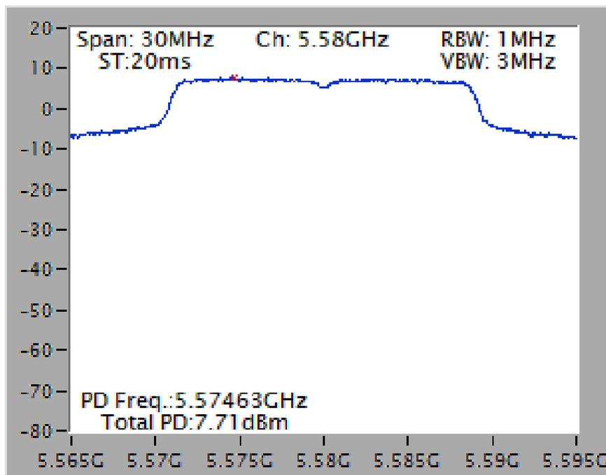
Power Density Plot on Configuration IEEE 802.11ac MCS0/Nss1 VHT40 / Chain 5 / 5270 MHz
