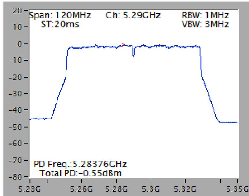
Power Density Plot on Configuration IEEE 802.11ac MCS0/Nss1 VHT80 / Chain 1 + Chain 2 + Chain 3 + Chain 4 / 5610 MHz
