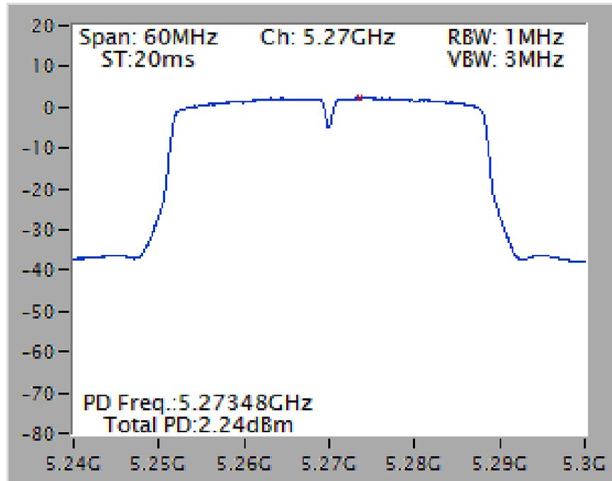
Power Density Plot on Configuration IEEE 802.11ac MCS0/Nss1 VHT40 / Chain 1 + Chain 2 + Chain 3 + Chain 4 / 5550 MHz
