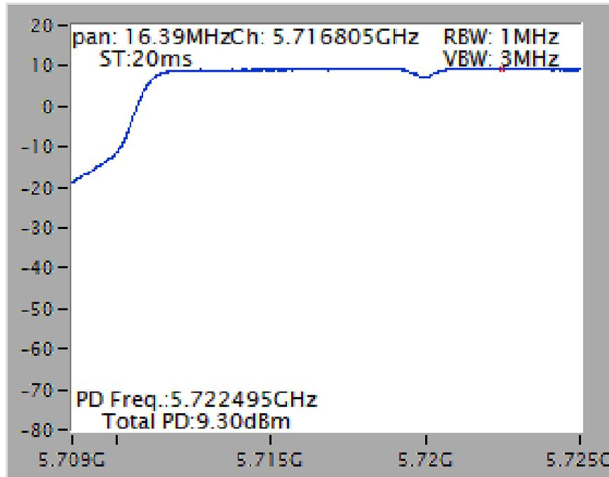
Power Density Plot on Configuration IEEE 802.11ac MCS0/Nss3 VHT20 / Chain 1 + Chain 2 + Chain 3 + Chain 4 / 5720 MHz (UNII 3)
