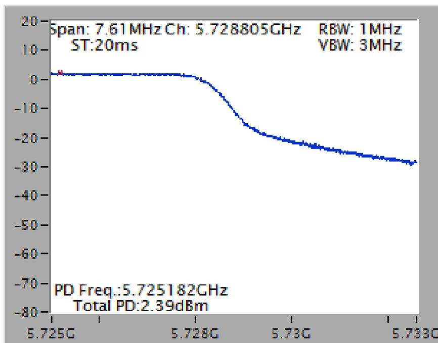
Power Density Plot on Configuration IEEE 802.11ac MCS0/Nss3 VHT80 / Chain 1 + Chain 2 + Chain 3 + Chain 4 / 5690 MHz (UNII 2C)
