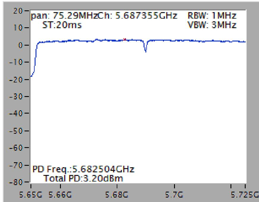
Power Density Plot on Configuration IEEE 802.11ac MCS0/Nss2 VHT80 / Chain 1 + Chain 2 + Chain 3 + Chain 4 / 5690 MHz (UNII 3)
