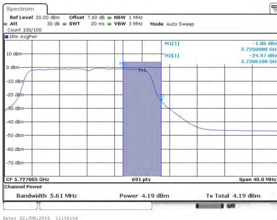
**Conducted Output Power Plot on Configuration IEEE 802.11ac MCS0/Nss3 VHT40 / Chain 1 / 5710 MHz (UNII 2C)**
