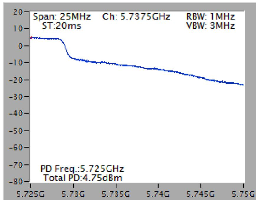
Power Density Plot on Configuration IEEE 802.11ac MCS0/Nss1 VHT40 / Chain 5 / 5710 MHz (UNII 2C)
