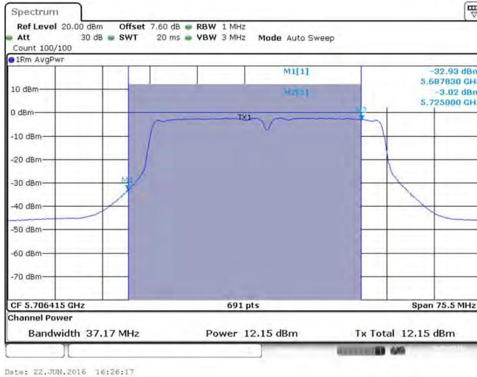
**Conducted Output Power Plot on Configuration IEEE 802.11ac MCS0/Nss3 VHT40 / Chain 4 / 5710 MHz (UNII 2C)**
