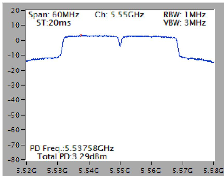
Power Density Plot on Configuration IEEE 802.11ac MCS0/Nss1 VHT80 / Chain 5 / 5290 MHz
