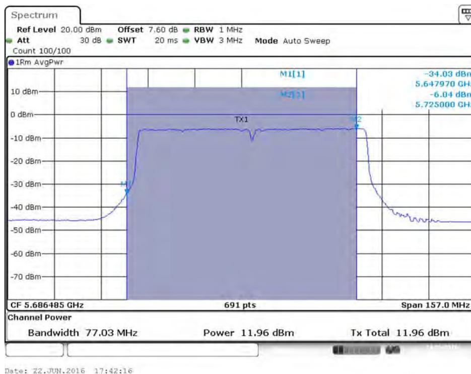
**Conducted Output Power Plot on Configuration IEEE 802.11ac MCS0/Nss3 VHT80 / Chain 1 / 5690 MHz (UNII 3)**
