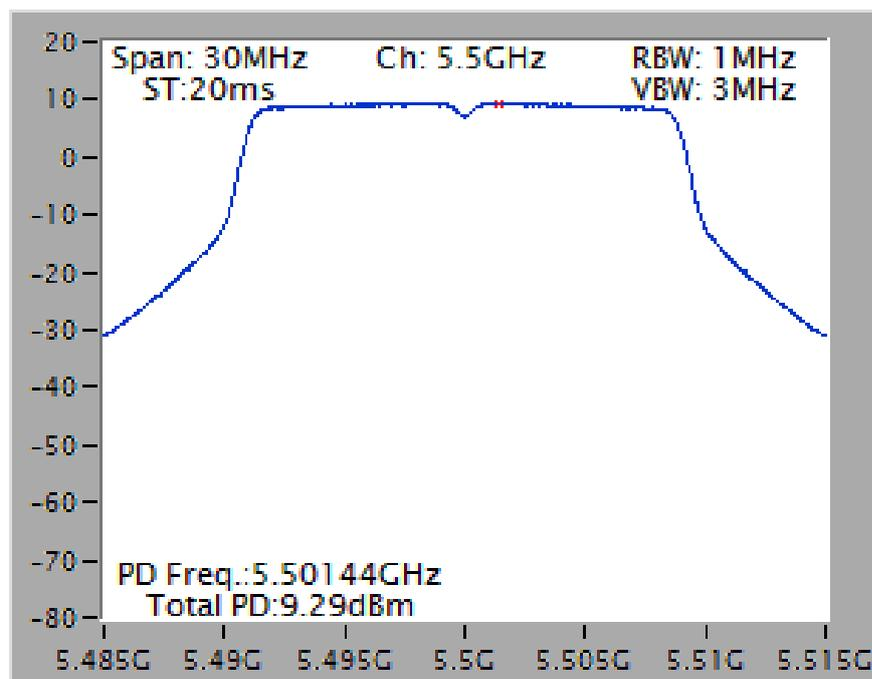
Power Density Plot on Configuration IEEE 802.11ac MCS0/Nss3 VHT40 / Chain 1 + Chain 2 + Chain 3 + Chain 4 / 5270 MHz
