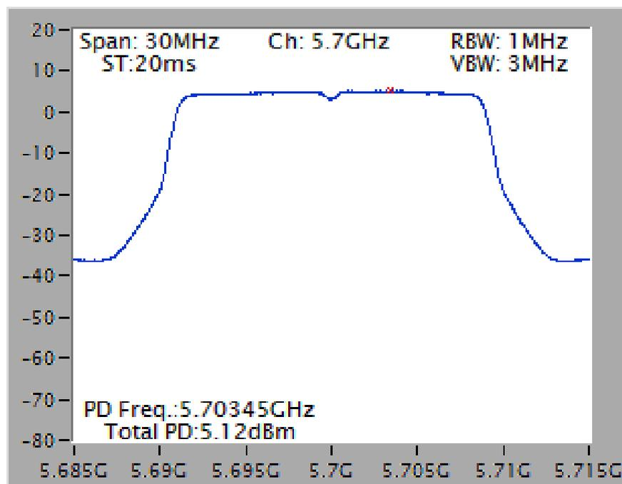
Power Density Plot on Configuration IEEE 802.11ac MCS0/Nss1 VHT40 / Chain 1 + Chain 2 + Chain 3 + Chain 4 / 5270 MHz
