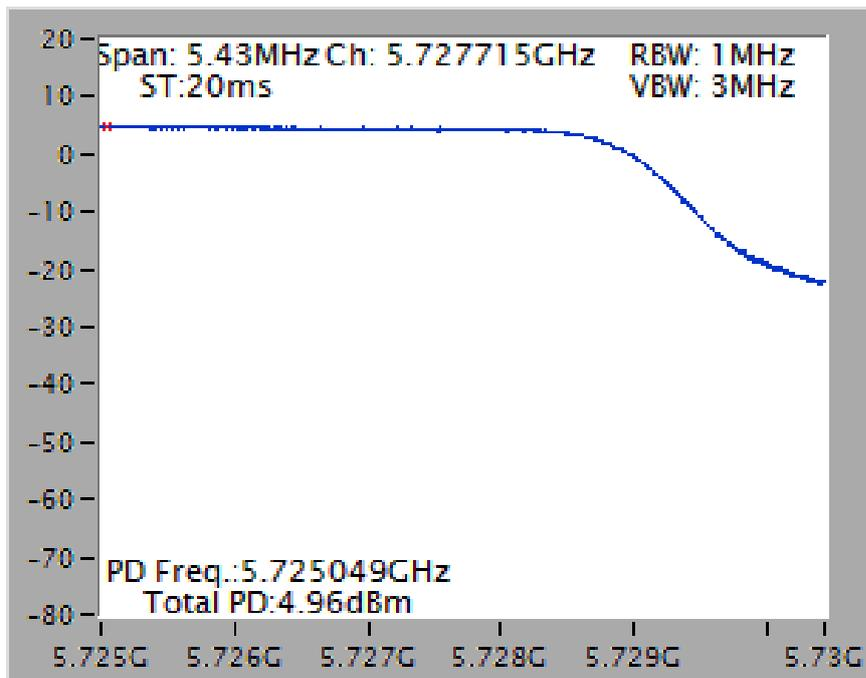
Power Density Plot on Configuration IEEE 802.11ac MCS0/Nss1 VHT40 / Chain 1 + Chain 2 + Chain 3 + Chain 4 / 5710 MHz (UNII 2C)
