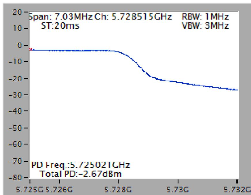
Power Density Plot on Configuration IEEE 802.11ac MCS0/Nss3 VHT20 / Chain 1 + Chain 2 + Chain 3 + Chain 4 / 5720 MHz (UNII 2C)
