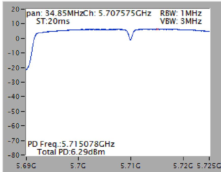
Power Density Plot on Configuration IEEE 802.11ac MCS0/Nss2 VHT40 / Chain 1 + Chain 2 + Chain 3 + Chain 4 / 5710 MHz (UNII 3)
