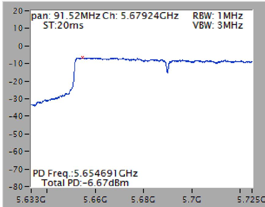
Power Density Plot on Configuration IEEE 802.11ac MCS0/Nss1 VHT80 / Chain 5 / 5690 MHz (UNII 3)
