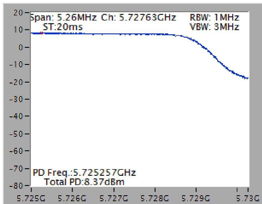
Power Density Plot on Configuration IEEE 802.11ac MCS0/Nss2 VHT40 / Chain 1 + Chain 2 + Chain 3 + Chain 4 / 5710 MHz (UNII 2C)
