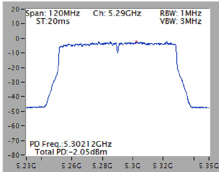
Power Density Plot on Configuration IEEE 802.11ac MCS0/Nss2 VHT80 / Chain 1 + Chain 2 + Chain 3 + Chain 4 / 5530 MHz
