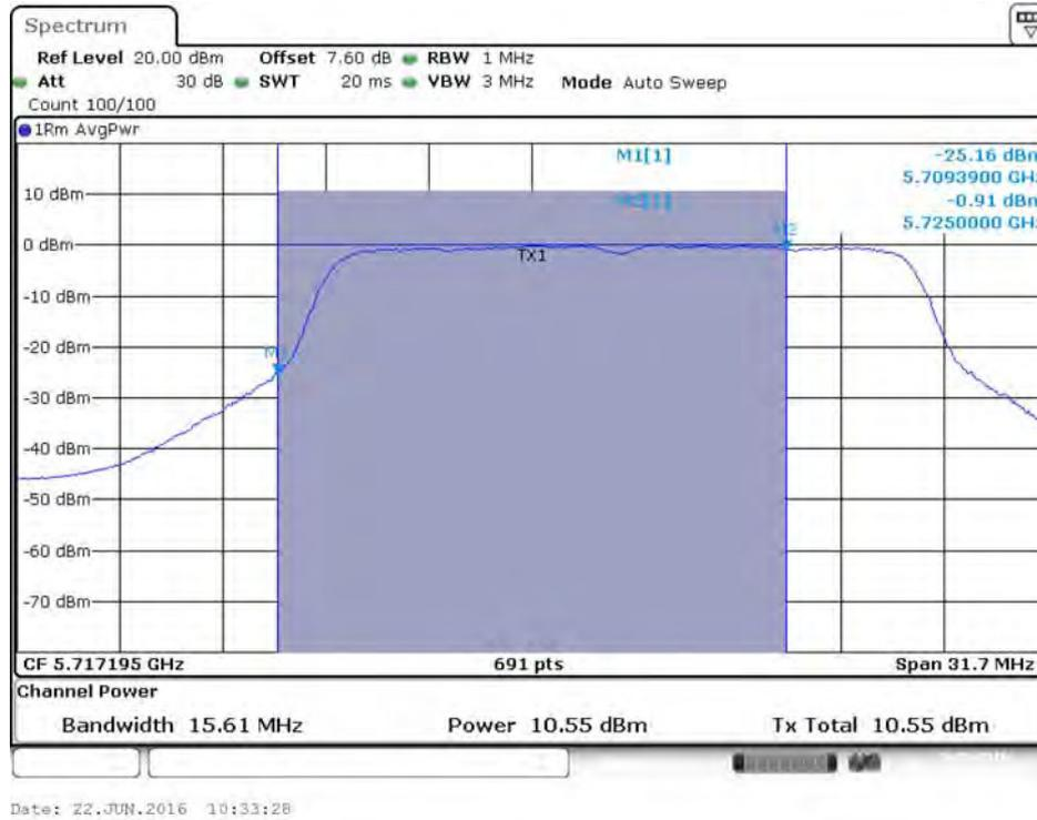
**Conducted Output Power Plot on Configuration IEEE 802.11ac MCS0/Nss3 VHT20 / Chain 2 / 5720 MHz (UNII 2C)**
