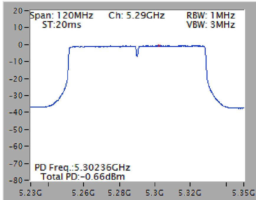
Power Density Plot on Configuration IEEE 802.11ac MCS0/Nss4 VHT80 / Chain 1 + Chain 2 + Chain 3 + Chain 4 / 5610 MHz
