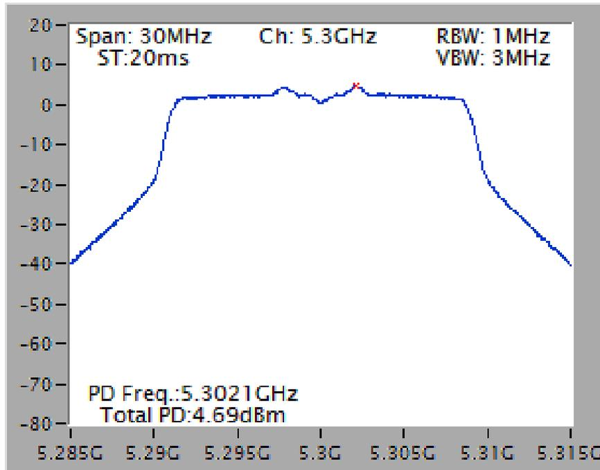
Power Density Plot on Configuration IEEE 802.11ac MCS0/Nss3 VHT20 / Chain 1 + Chain 2 + Chain 3 + Chain 4 / 5580 MHz
