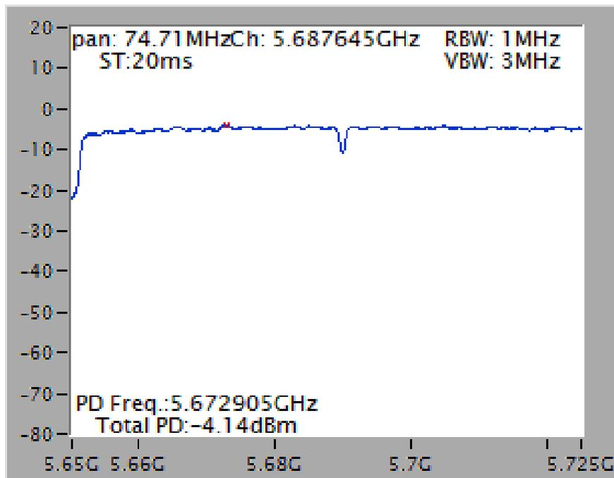
Power Density Plot on Chain 3 + Chain 4 / 5690 MHz (UNII 3)
