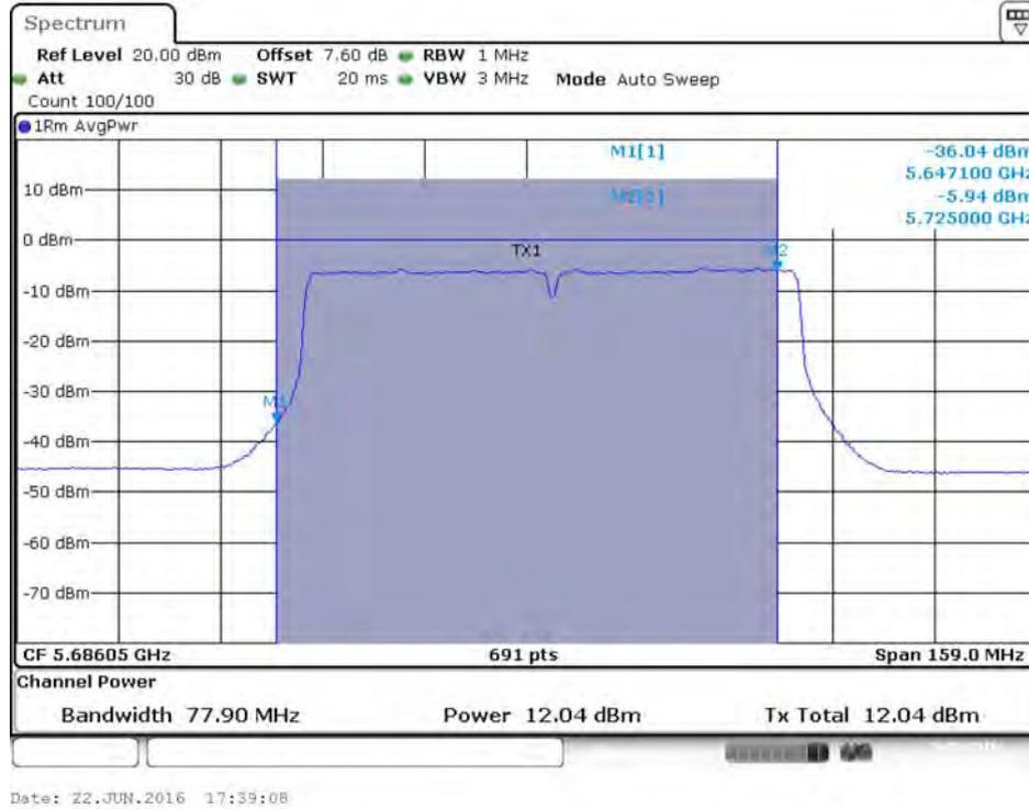
**Conducted Output Power Plot on Configuration IEEE 802.11ac MCS0/Nss3 VHT80 / Chain 2 / 5690 MHz (UNII 2C)**
