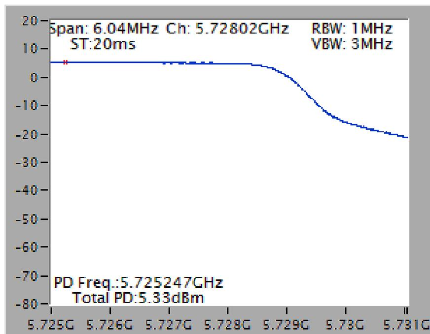
Power Density Plot on Configuration IEEE 802.11ac MCS0/Nss4 VHT40 / Chain 1 + Chain 2 + Chain 3 + Chain 4 / 5710 MHz (UNII 2C)
