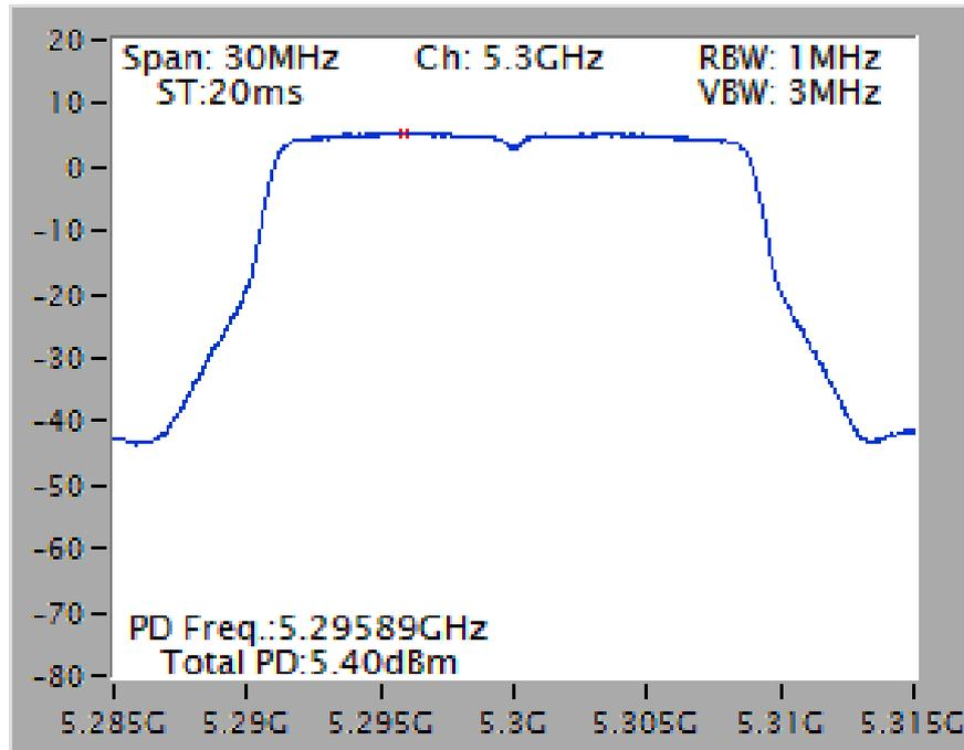
Power Density Plot on Configuration IEEE 802.11ac MCS0/Nss1 VHT20 / Chain 1 + Chain 2 + Chain 3 + Chain 4 / 5500 MHz
