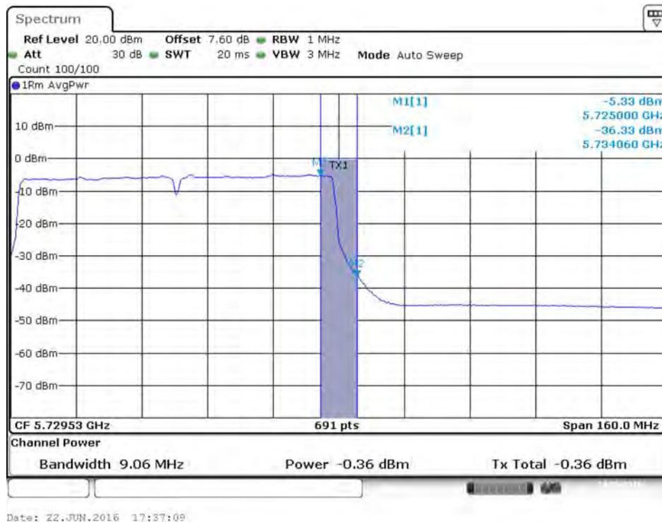
**Conducted Output Power Plot on Configuration IEEE 802.11ac MCS0/Nss3 VHT80 / Chain 3 / 5690 MHz (UNII 3)**
