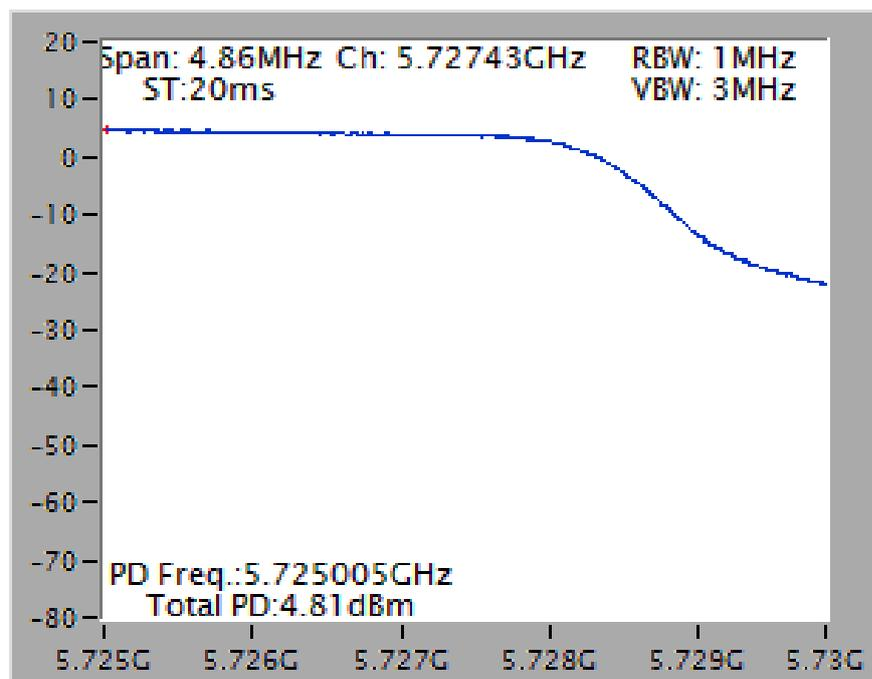
Power Density Plot on Configuration IEEE 802.11ac MCS0/Nss2 VHT80 / Chain 1 + Chain 2 + Chain 3 + Chain 4 / 5690 MHz (UNII 2C)
