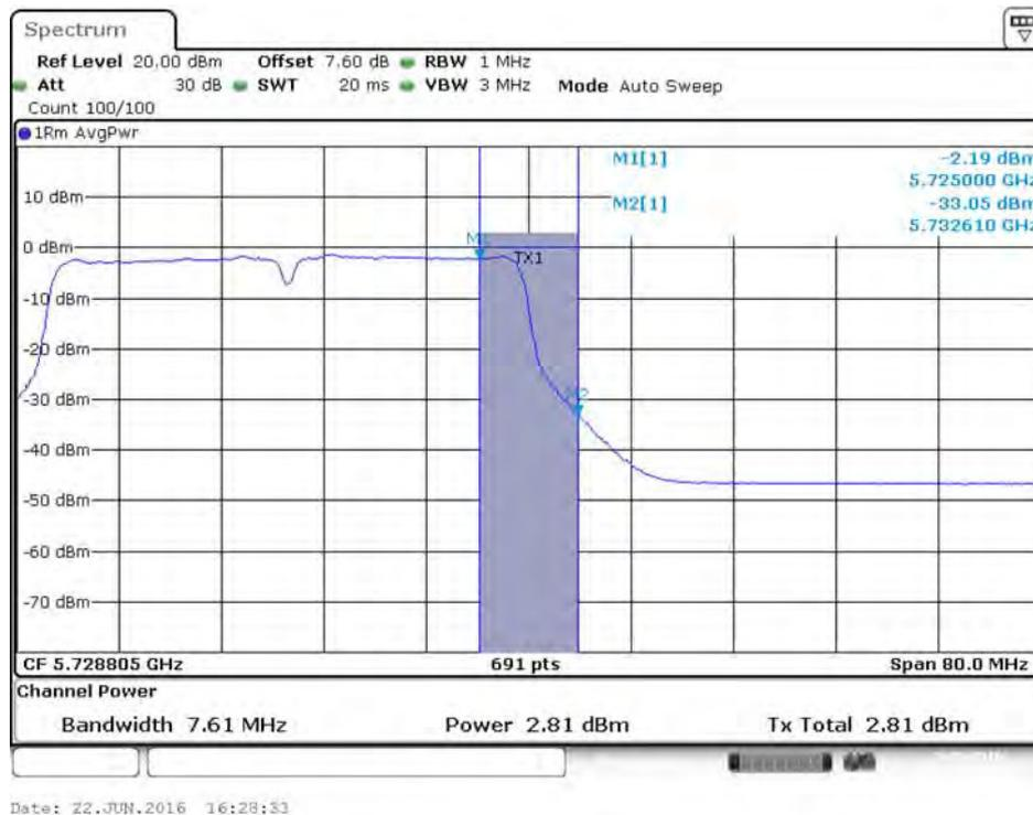
**Conducted Output Power Plot on Configuration IEEE 802.11ac MCS0/Nss3 VHT40 / Chain 3 / 5710 MHz (UNII 3)**
