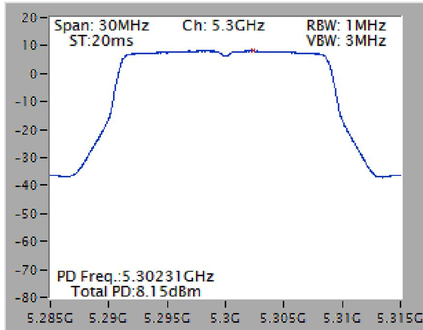
Power Density Plot on Configuration IEEE 802.11ac MCS0/Nss2 VHT20 / Chain 1 + Chain 2 + Chain 3 + Chain 4 / 5580 MHz
