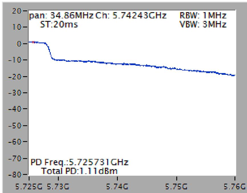
Power Density Plot on Configuration IEEE 802.11ac MCS0/Nss1 VHT80 / Chain 5 / 5690 MHz (UNII 2C)
