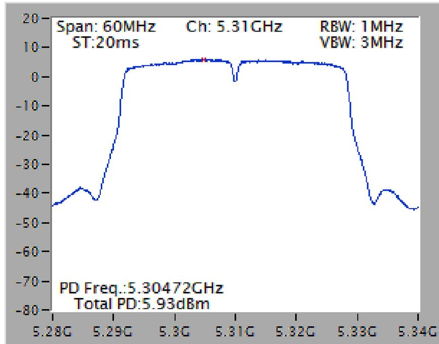
Power Density Plot on Configuration IEEE 802.11ac MCS0/Nss1 VHT40 / Chain 1 + Chain 2 + Chain 3 + Chain 4 / 5510 MHz
