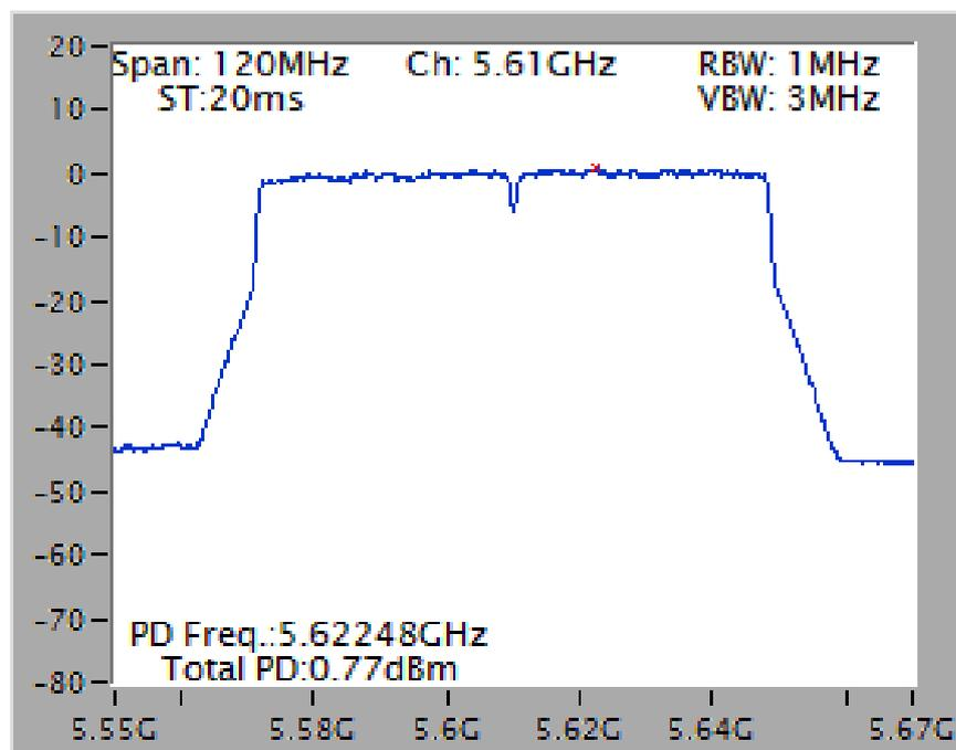
Power Density Plot on Configuration IEEE 802.11ac MCS0/Nss4 VHT20 / Chain 1 + Chain 2 + Chain 3 + Chain 4 / 5260 MHz
