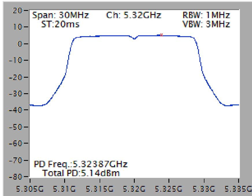
Power Density Plot on Configuration IEEE 802.11ac MCS0/Nss1 VHT20 / Chain 1 + Chain 2 + Chain 3 + Chain 4 / 5700 MHz
