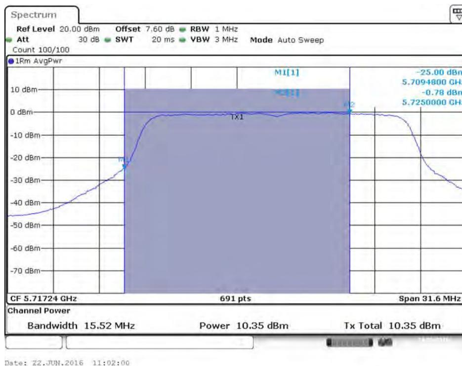
**Conducted Output Power Plot on Configuration IEEE 802.11ac MCS0/Nss3 VHT20 / Chain 1 / 5720 MHz (UNII 3)**
