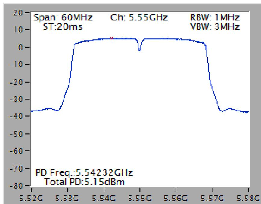
Power Density Plot on Configuration IEEE 802.11ac MCS0/Nss2 VHT80 / Chain 1 + Chain 2 + Chain 3 + Chain 4 / 5290 MHz
