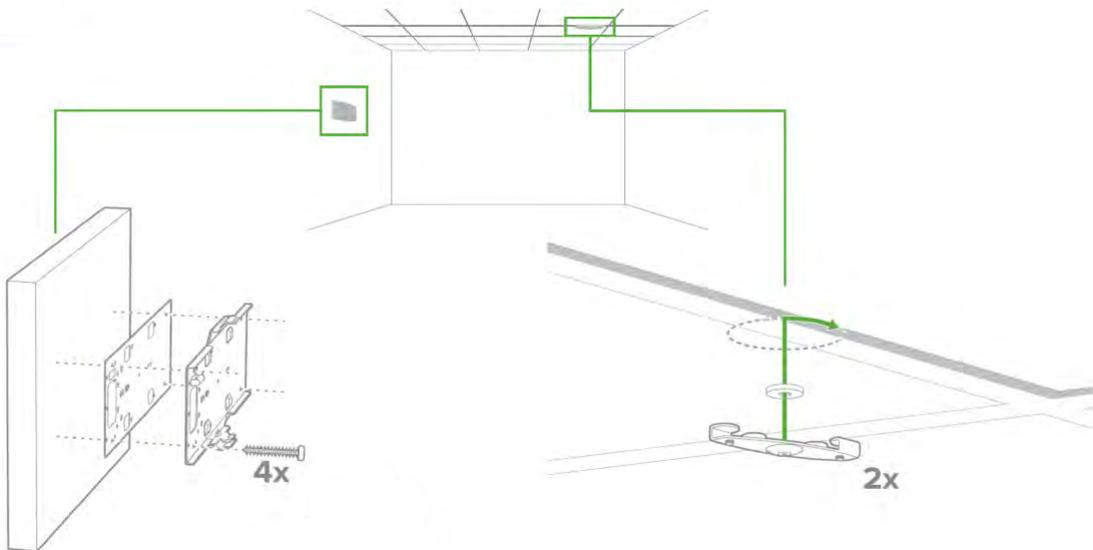
1. Attach the T-rail clips to the T-rail by rotating them and snapping them into place as shown. The black foam pads should be compressed slightly after installation.
