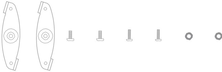
Dropped ceiling mounting clips with set screws
