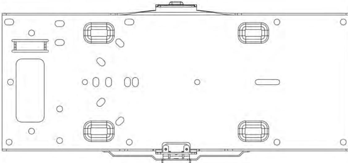
It is recommended that the MR46E-HW be mounted to a wall or solid ceiling using the mount plate for physical security reasons.
