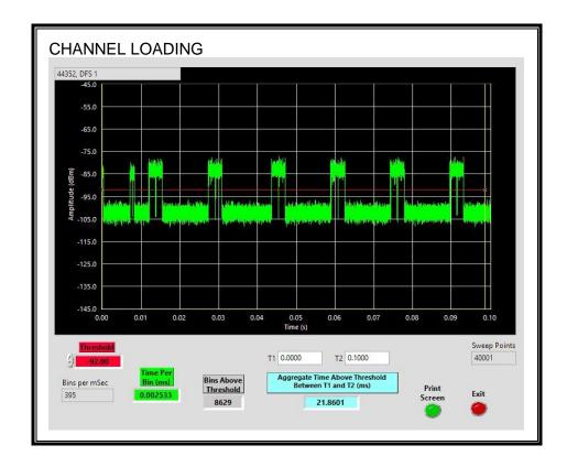
The level of traffic loading on the channel by the EUT is 21.8601%.
