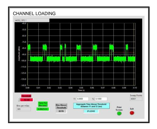
The level of traffic loading on the channel by the EUT is 21.2243%.
