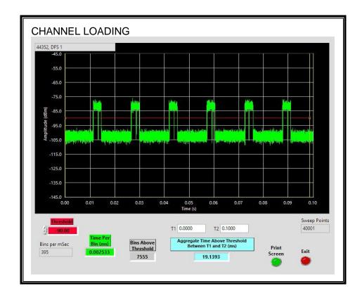
The level of traffic loading on the channel by the EUT is 19.1393%.
