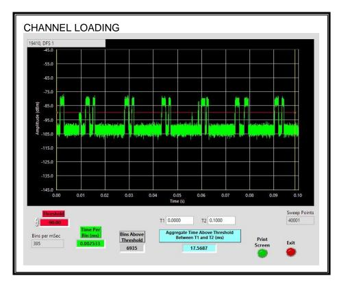
The level of traffic loading on the channel by the EUT is 17.57%
