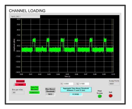
The level of traffic loading on the channel by the EUT is 17.91%
