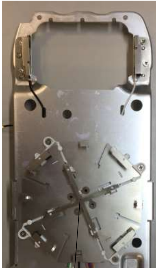
4x4 Modularized WiFi Antenna
