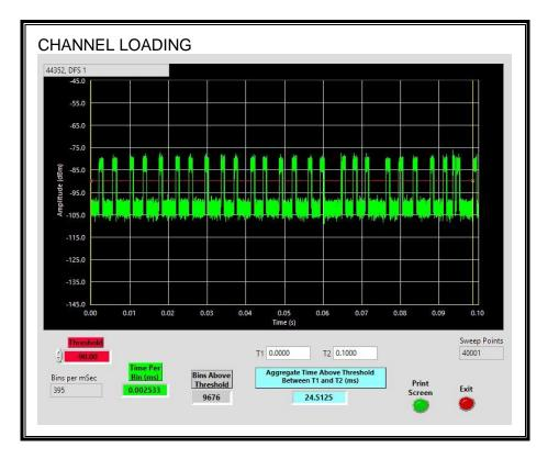
The level of traffic loading on the channel by the EUT is 24.5125%.
