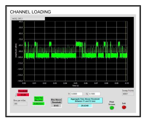
The level of traffic loading on the channel by the EUT is 20.634%.
