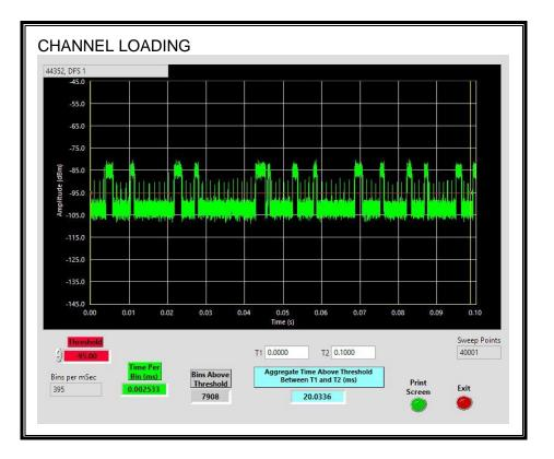
The level of traffic loading on the channel by the EUT is 20.0336%.
