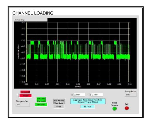
The level of traffic loading on the channel by the EUT is 22.11%.
