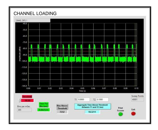
The level of traffic loading on the channel by the EUT is 18.32%.
