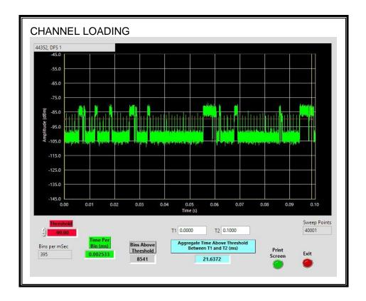
The level of traffic loading on the channel by the EUT is 21.6372%.
