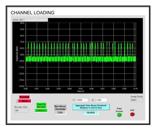
The level of traffic loading on the channel by the EUT is 18.6428%.
