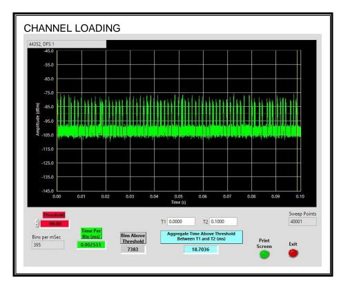
The level of traffic loading on the channel by the EUT is 18.7036%
