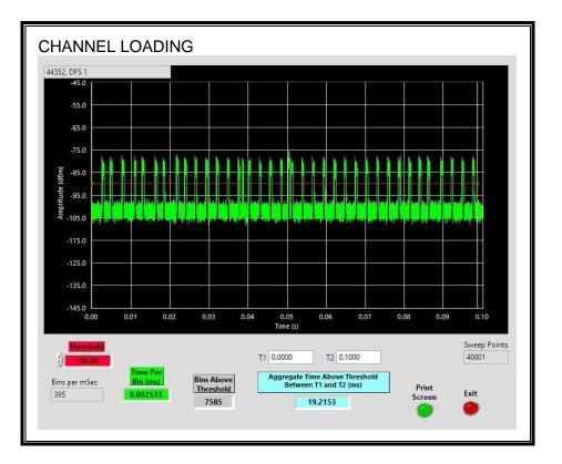
The level of traffic loading on the channel by the EUT is 19.2153%
