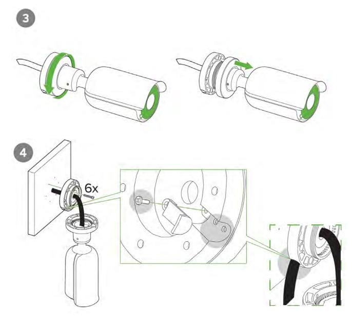
Note: The fixed power cable will not be exposed to the outdoor environment after successful installation of the MV52 on a wall using the provided mount.
