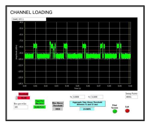
The level of traffic loading on the channel by the EUT is 19.9%
