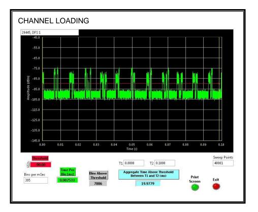
The level of traffic loading on the channel by the EUT is 19.97%
