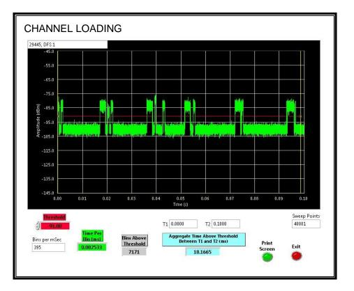
The level of traffic loading on the channel by the EUT is 18.16%
