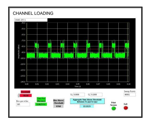
The level of traffic loading on the channel by the EUT is 22.21%
