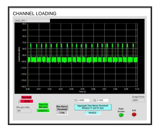
The level of traffic loading on the channel by the EUT is 19.6232%.
