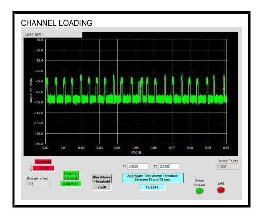
The level of traffic loading on the channel by the EUT is 19.3243%.
