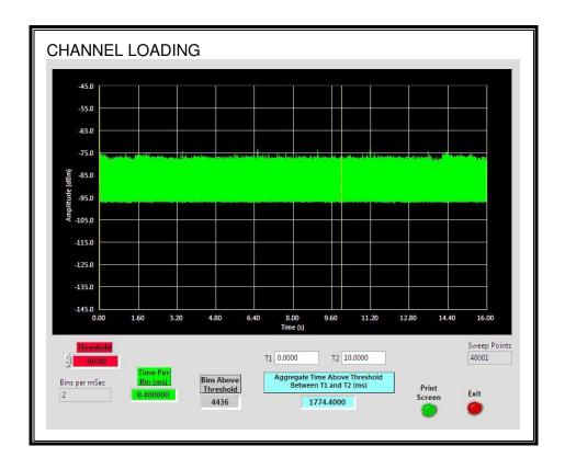
The level of traffic loading on the channel by the EUT is 17.744%
