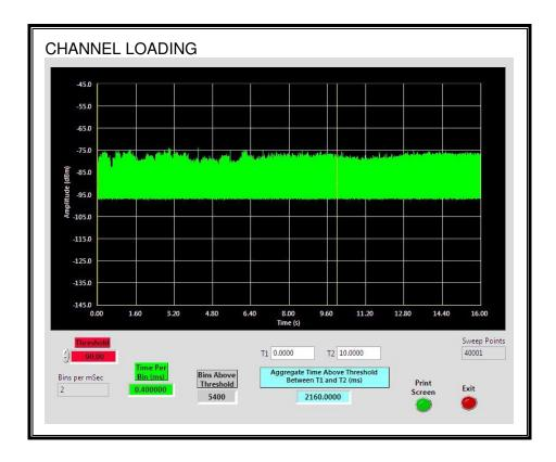
The level of traffic loading on the channel by the EUT is 21.6%
