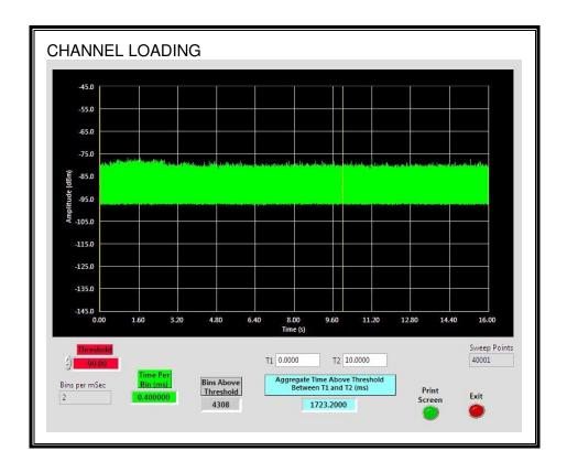
The level of traffic loading on the channel by the EUT is 17.232%
