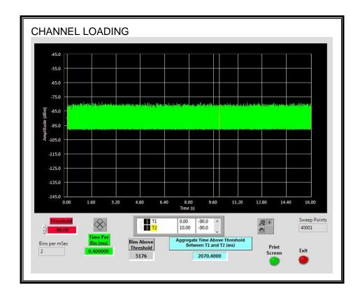
The level of traffic loading on the channel by the EUT is 20.704%
