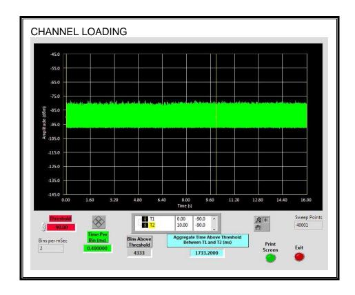
The level of traffic loading on the channel by the EUT is 17.332%
