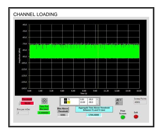
The level of traffic loading on the channel by the EUT is 17.044%
