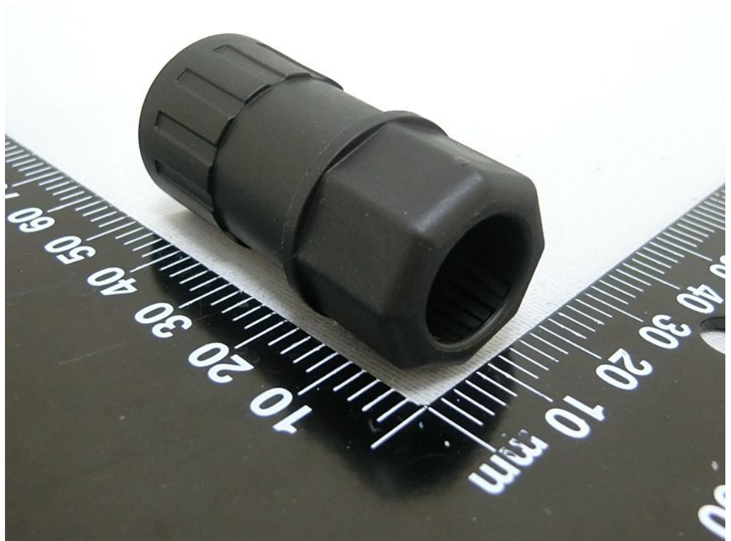
Waterproof Covering (Cable Gland) 1 used for EUT 1
