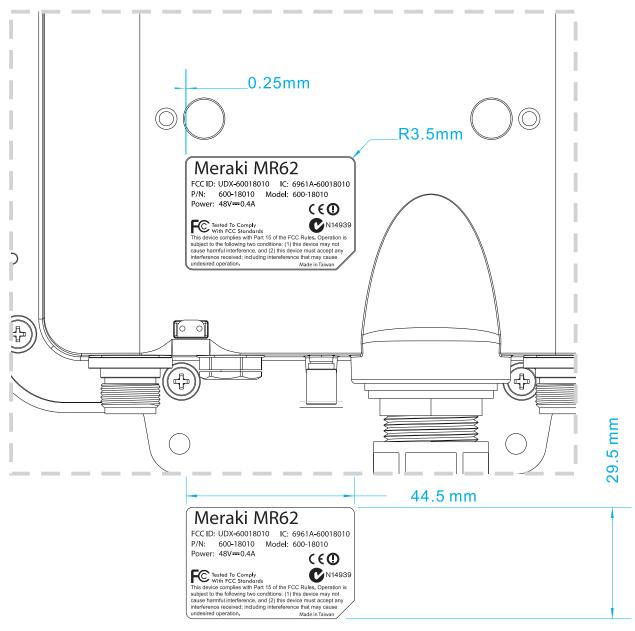
New dimensions: 44.5\*29.5mm Tolerance: -0.1mm
