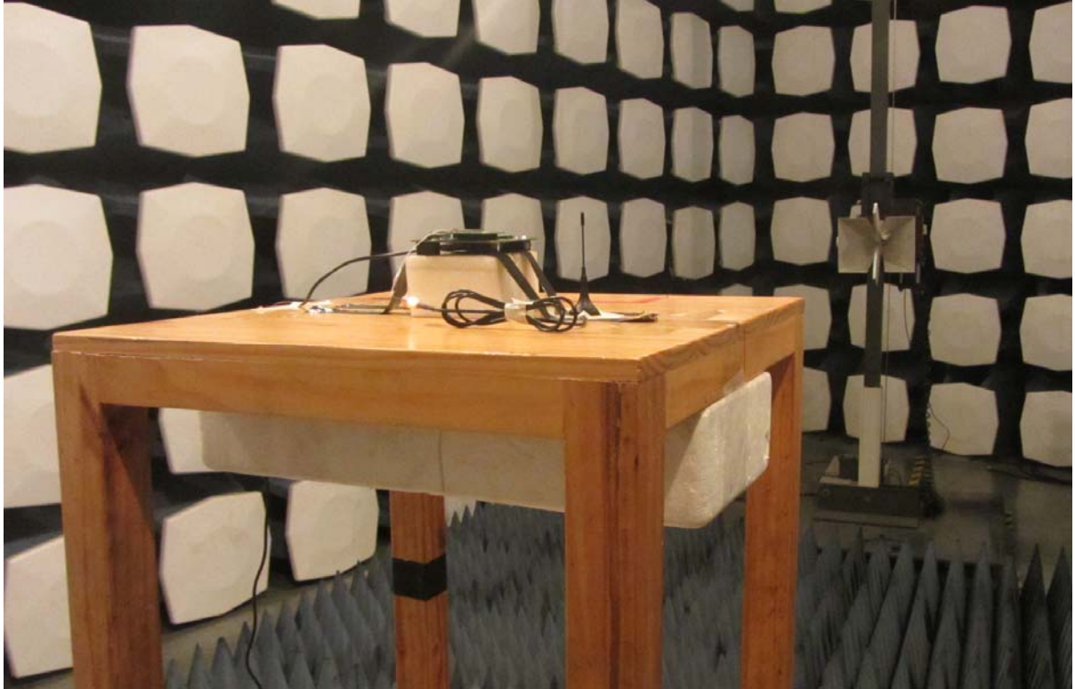
Picture 2: Radiated Spurious Emissions Test setup
