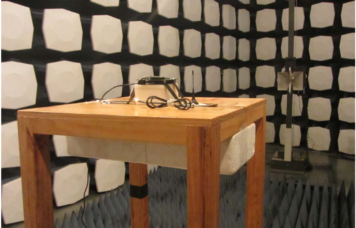
Picture 2: Radiated Spurious Emissions Test setup
