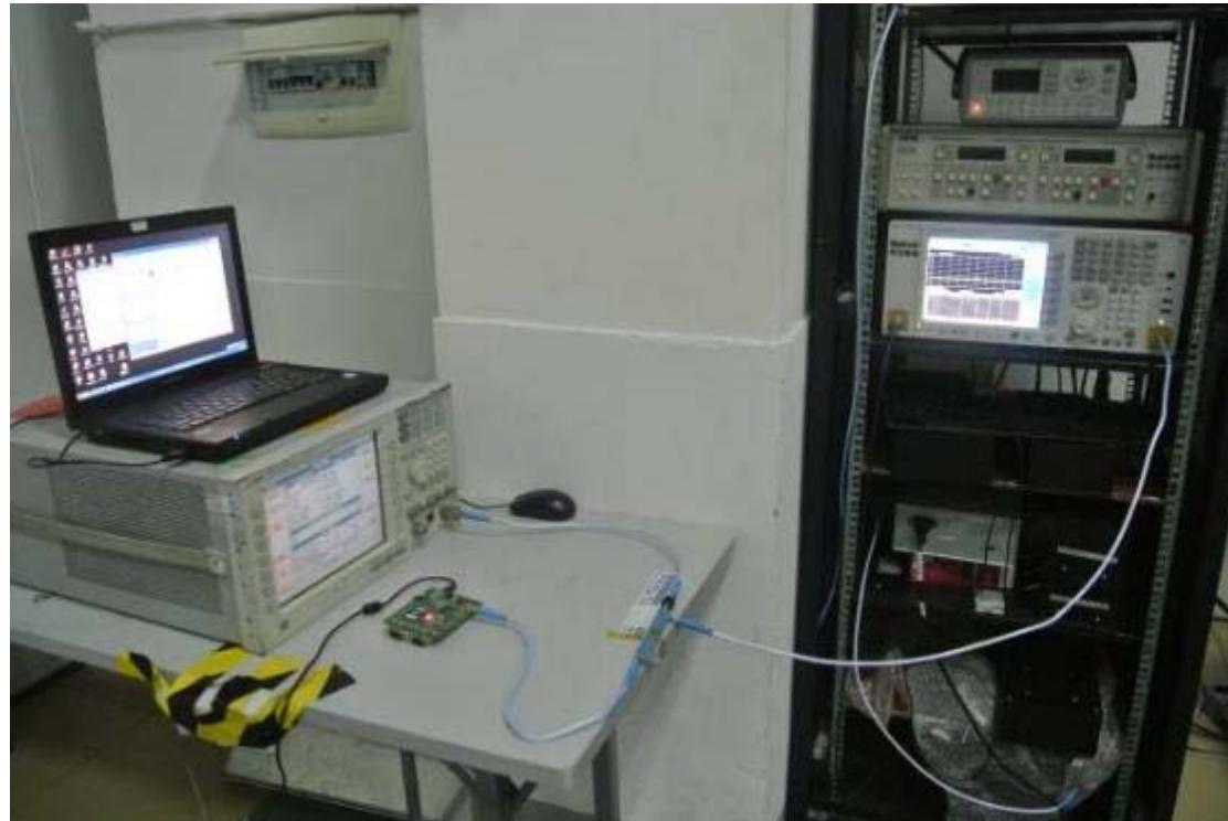
Description: Frequency Stability Under Temperature & Voltage Variations Test Setup
