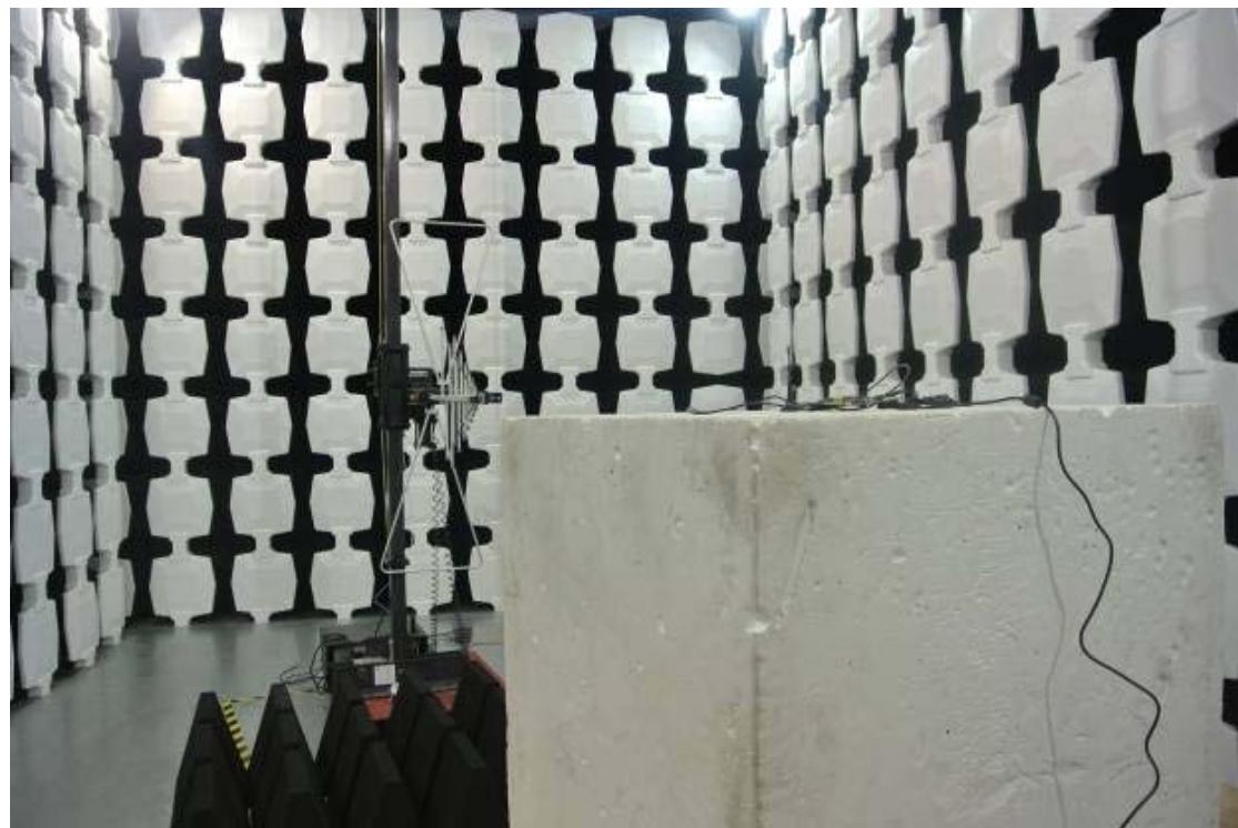
Description: EIRP / Radiated Spurious Measurement (Above 1GHz) Test Setup
