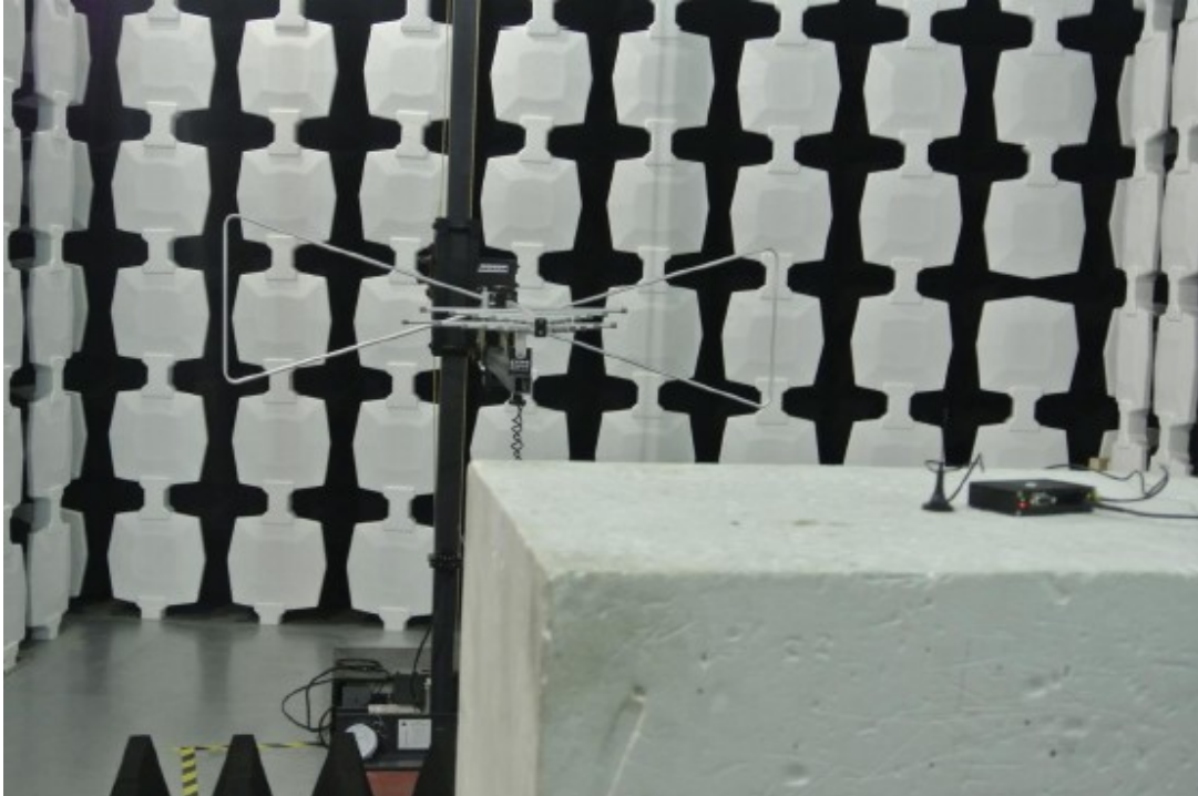
Spurious Emission/ERP Test:
