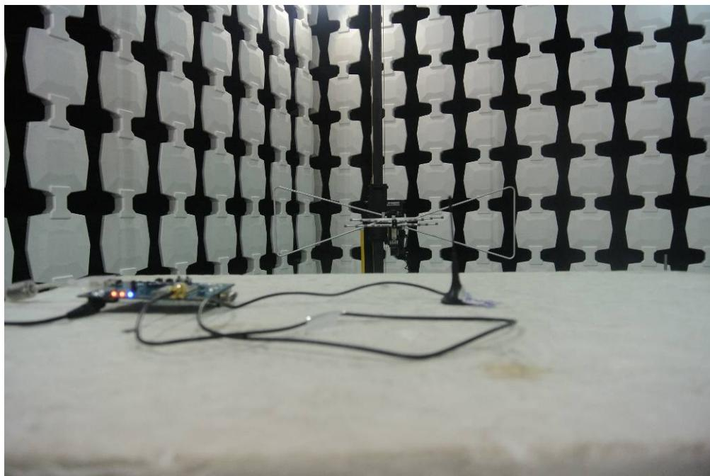
EIRP Test, Radiated Spurious Measurement (Above 1GHz) Setup
