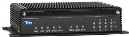
Figure 7.1A : AVL750MXB Front Panel
