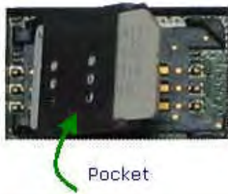
Figure 8.6 : SIM card holder pocket
