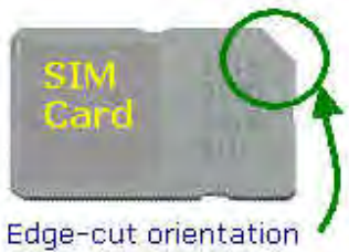
Figure 8.4 : SIM card orientation
