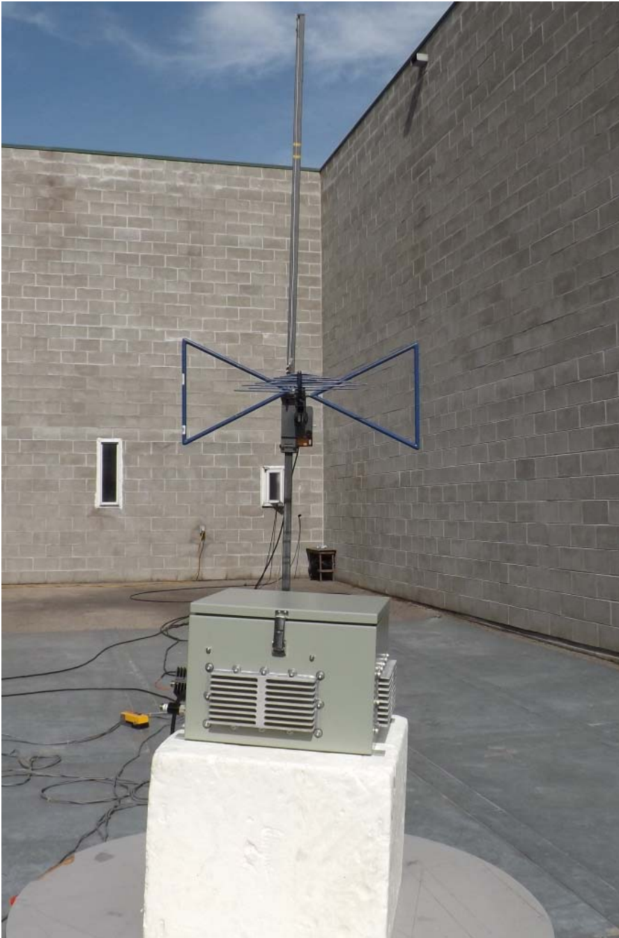
Figure E24.2 – Setup – Radiated Measurements – Below 1GHz
