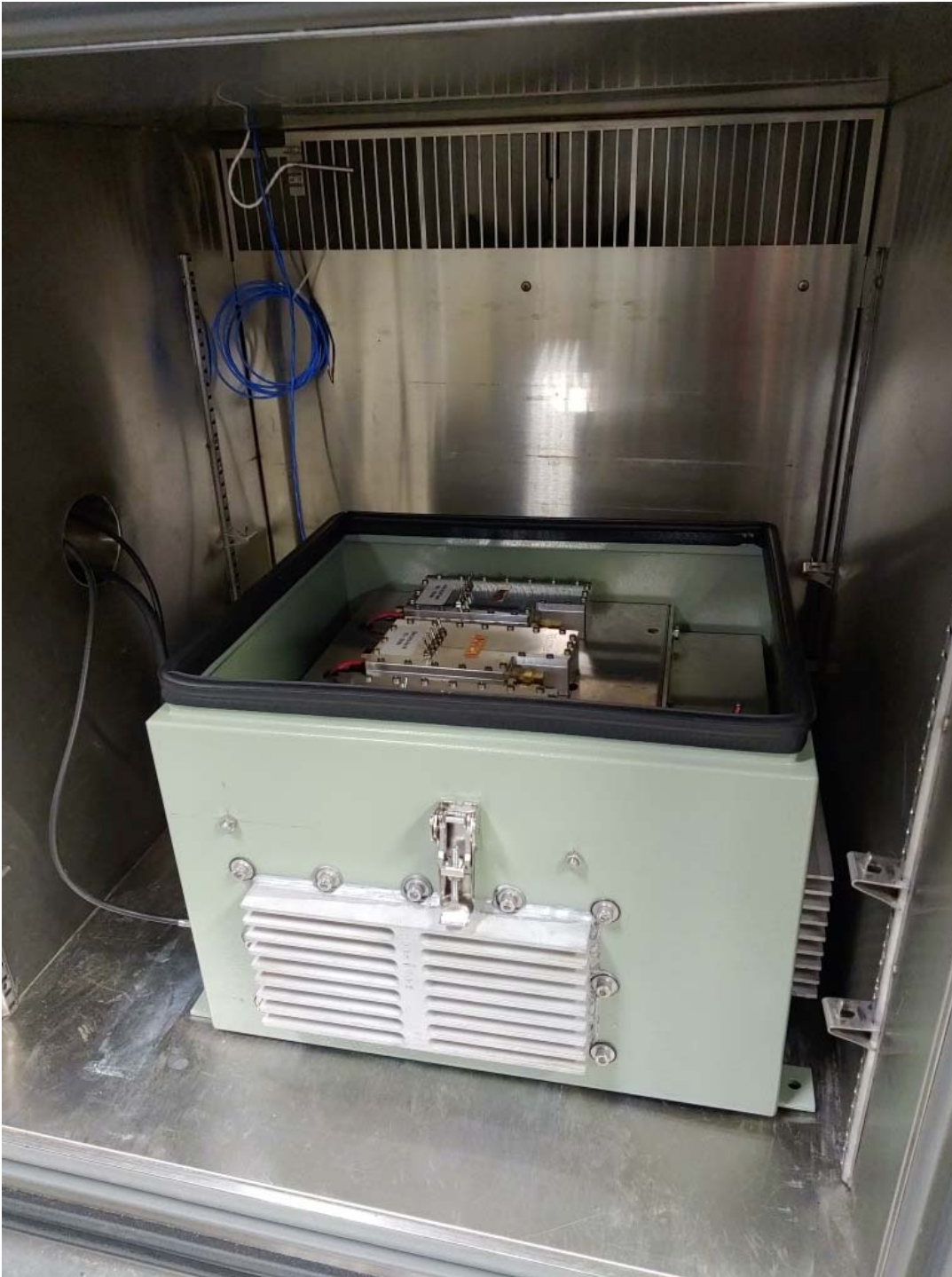
Figure E24.7 – Setup – Frequency Stability Measurements
