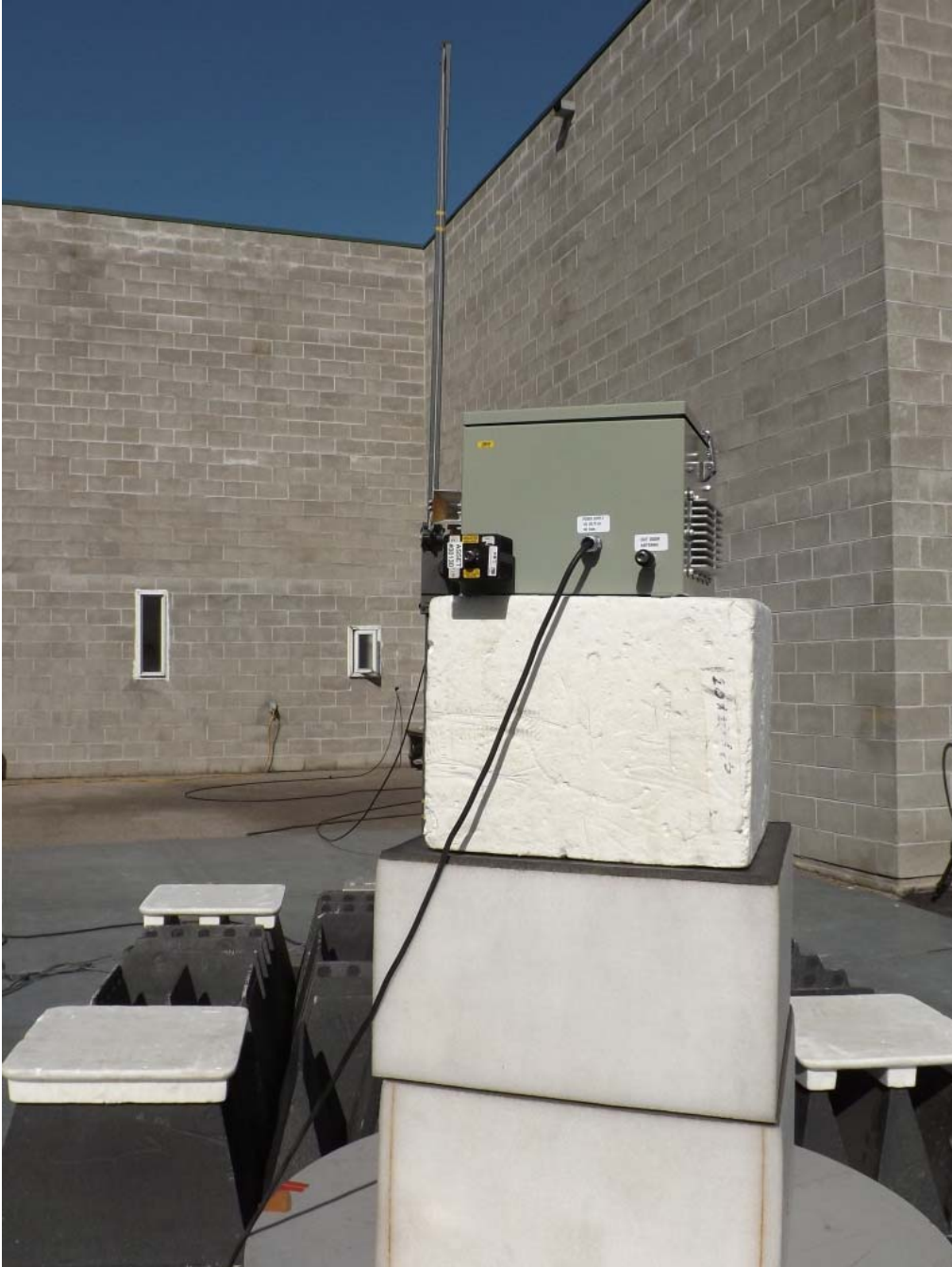
Figure E24.3 – Setup – Radiated Measurements – Above 1GHz
