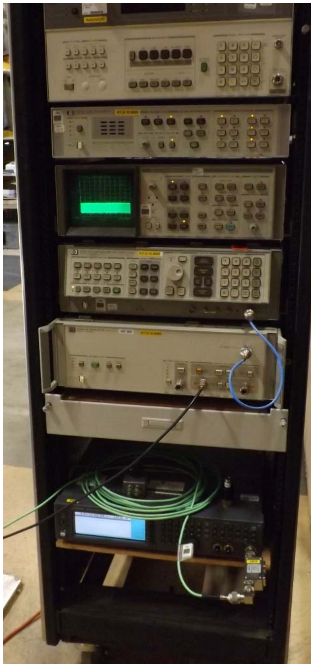
Figure E24.5 – Setup – Power Line Conducted Measurements
