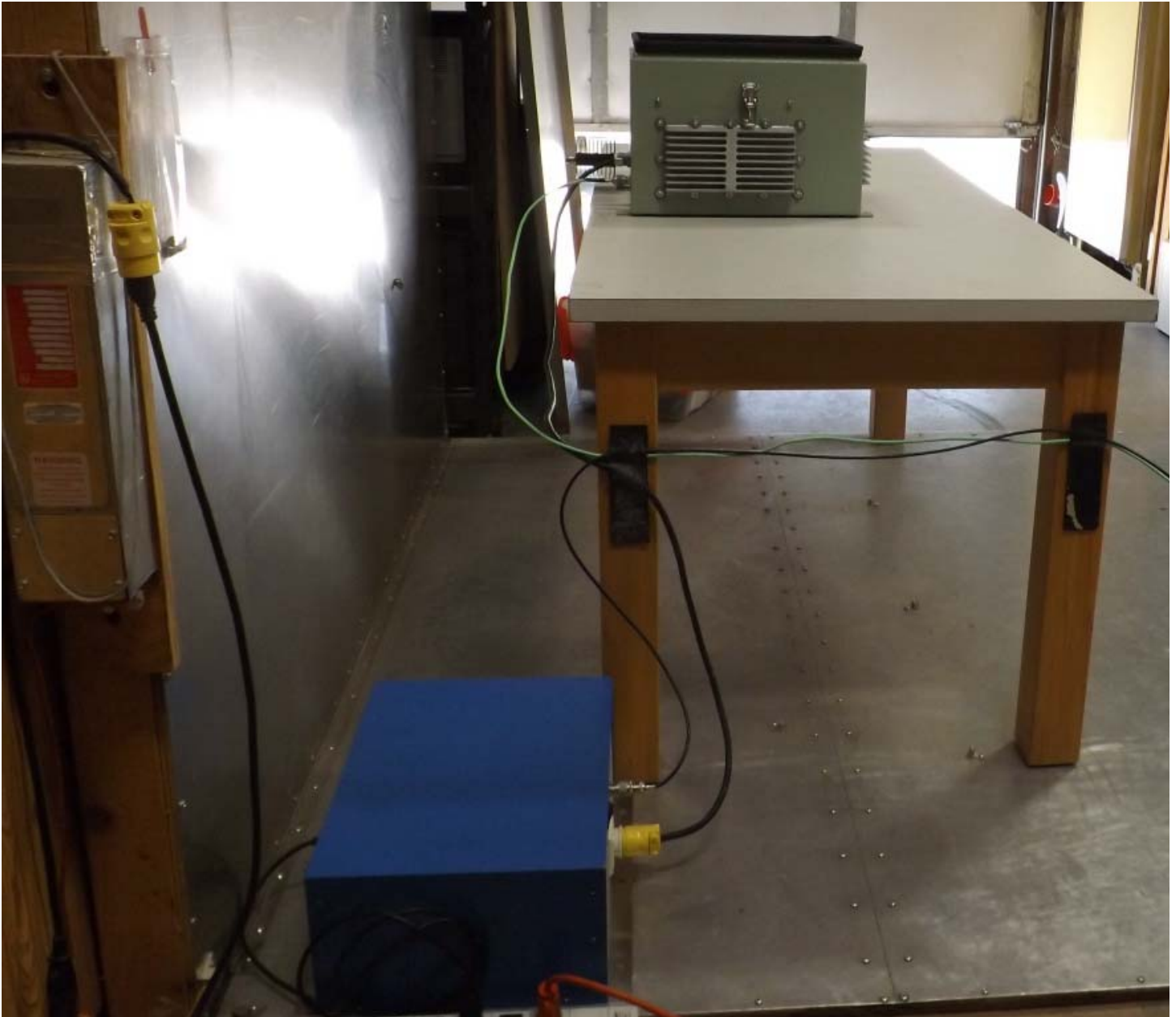
Figure E24.4 – Setup – Power Line Conducted Measurements
