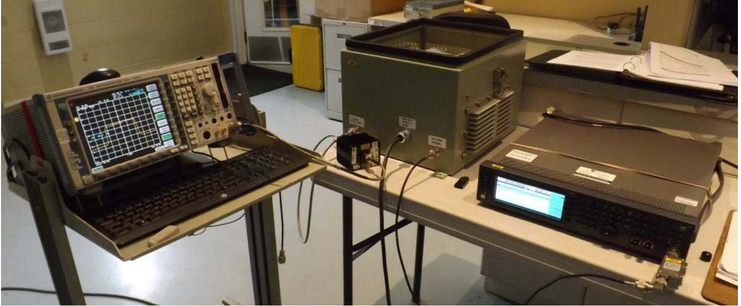
Figure E24.1 – Setup – Conducted Measurements
