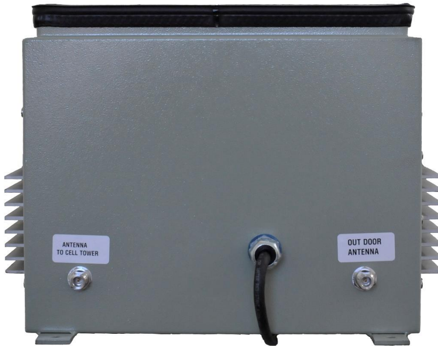
Figure 2 Location of the N Type Connectors for the Antennas
