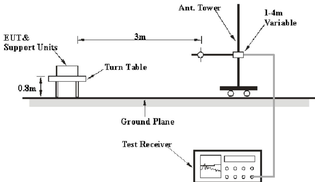
The radiated emission and out of band emission tests were performed in the 3 meters chamber A&B, using the setup accordance with the ANSI C63.4-2003. The specification used was the FCC 15.209 and FCC 15.249 limits.
