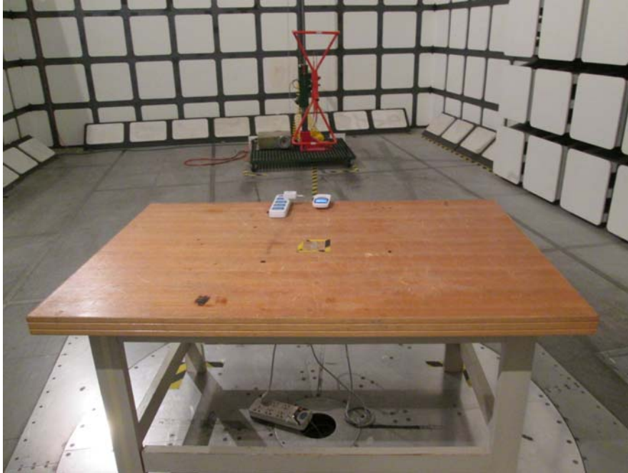
Radiated Emissions – Front View (Below 1 GHz, Charging by G.Credit adapter)
