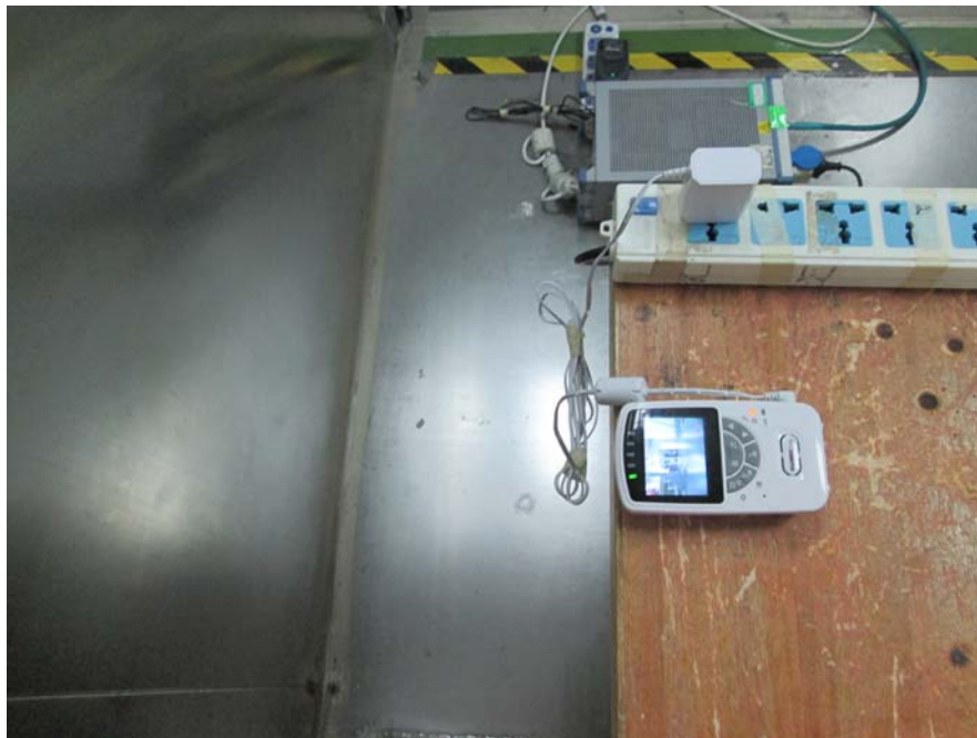
Conduction Emissions - Side View (Charging by G.Credit adapter)
