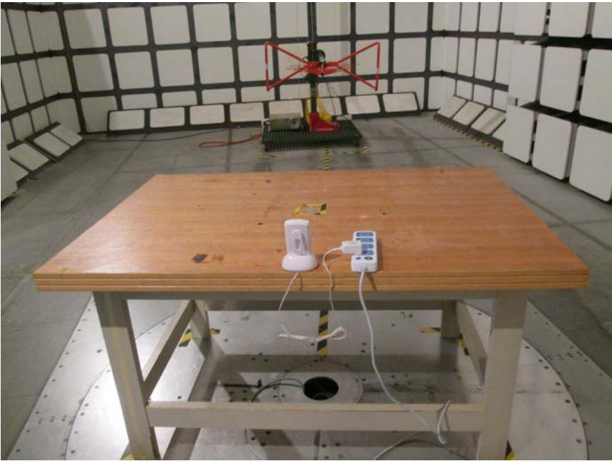
Radiated Emissions –Rear View (Below 1 GHz, Charging by KINGS charger)
