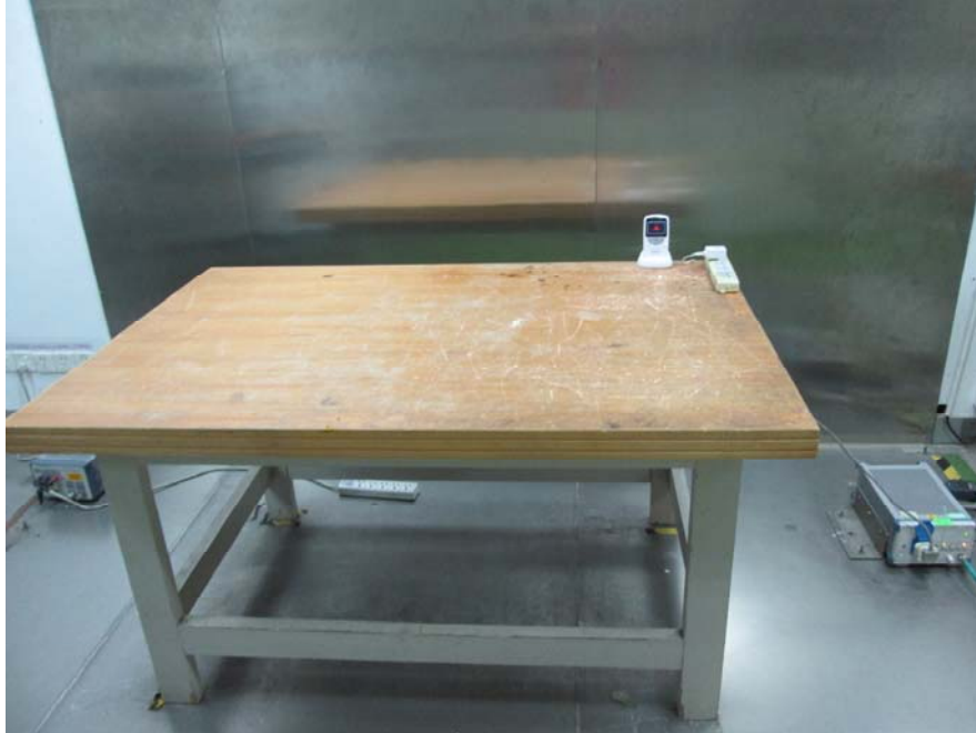
Conduction Emissions - Front View (Charging by KINGS charger)
