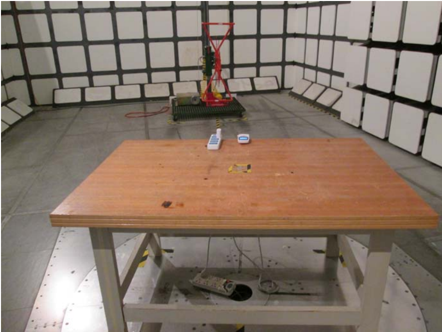
Radiated Emissions – Front View (Below 1 GHz, Charging by KINGS adapter))
