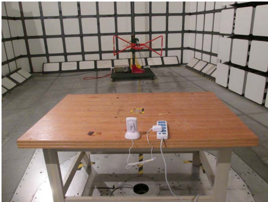
Radiated Emissions –Rear View (Below 1 GHz, Charging by 5ESP charger)
