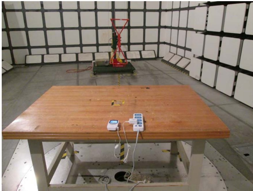
Radiated Emissions - Ride View (Below 1 GHz, Charging by G.Credit adapter)
