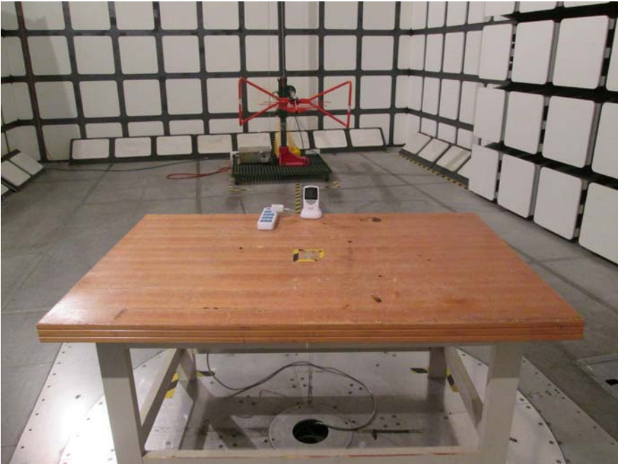
Radiated Emissions –Front View (Below 1 GHz, Charging by KINGS charger)
