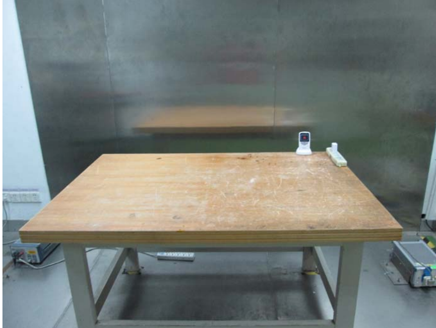
Conduction Emissions - Front View (Charging by G.Credit charger)
