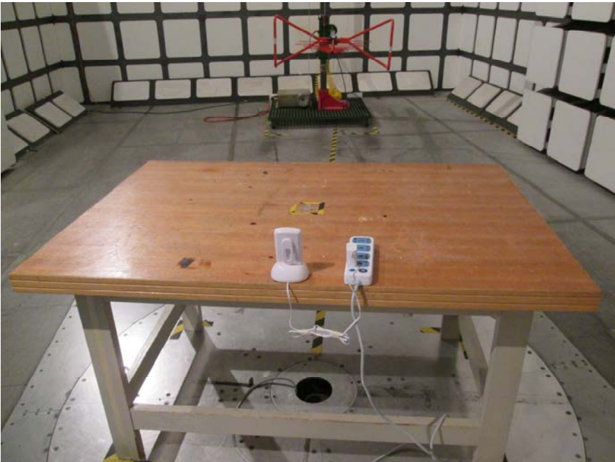
Radiated Emissions –Rear View (Below 1 GHz, Charging by G.Credit charger)
