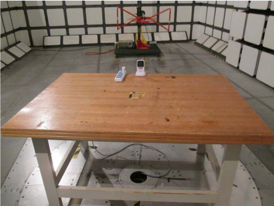
Radiated Emissions –Front View (Below 1 GHz, Charging by G.Credit charger)
