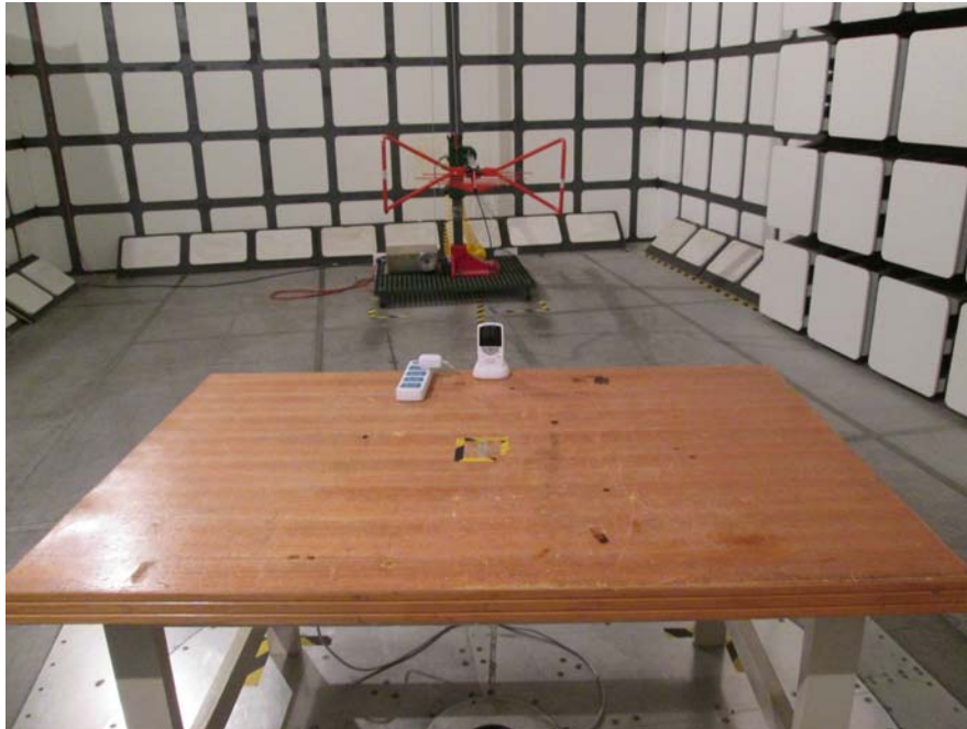
Radiated Emissions –Front View (Below 1 GHz, Charging by 5ESP charger)
