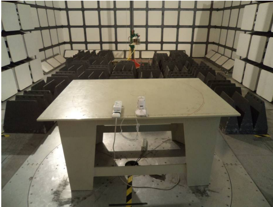
Radiated Emissions –Front View (Above 1 GHz)
