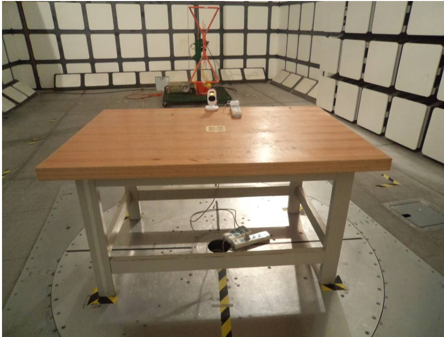
Radiated Emissions – Front View (Below 1 GHz)
