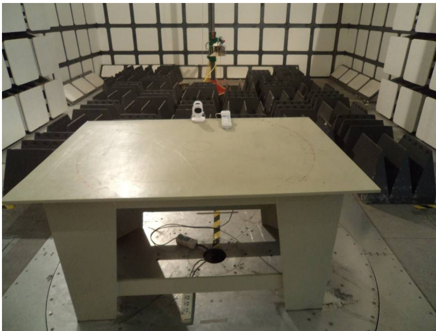
Radiated Emissions –Rear View (Above 1 GHz)
