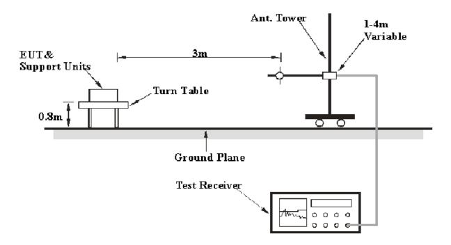
The radiated emission tests were performed in the 3 meters, using the setup accordance with the ANSI C63.4-2009. The specification used was the FCC 15.209 and FCC 15.247 limits.
