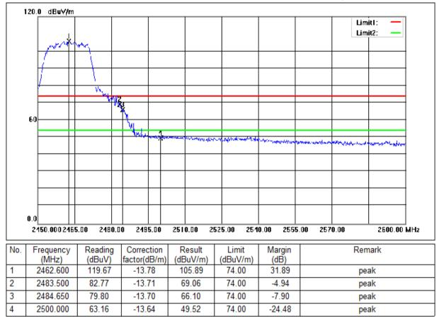
Mode:a; Polarization:Horizontal; Modulation:n; bandwidth:20MHz; Channel:High
