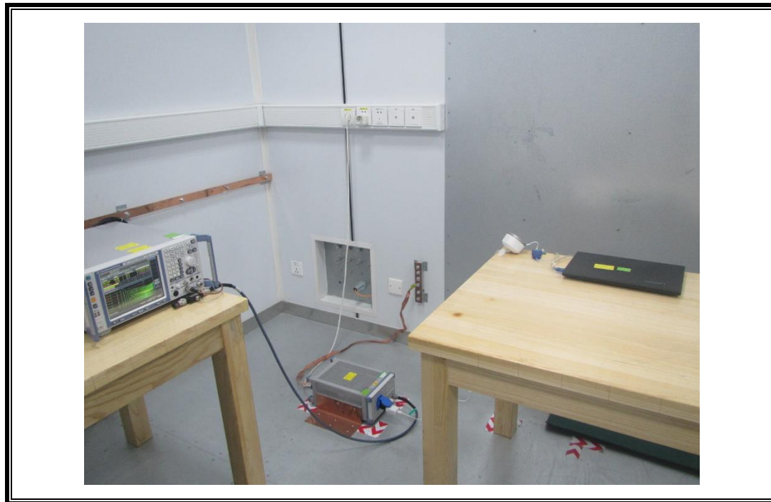
POWERLINE CONDUCTED EMISSIONS MEASUREMENT SETUP
