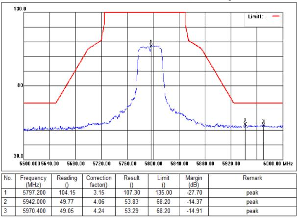
Mode:d; Polarization:Vertical; Modulation:ac; bandwidth:40MHz; Channel:High
