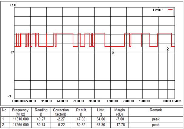
Mode:d; Polarization:Horizontal; Modulation:ac; bandwidth:40MHz; Channel:Low
