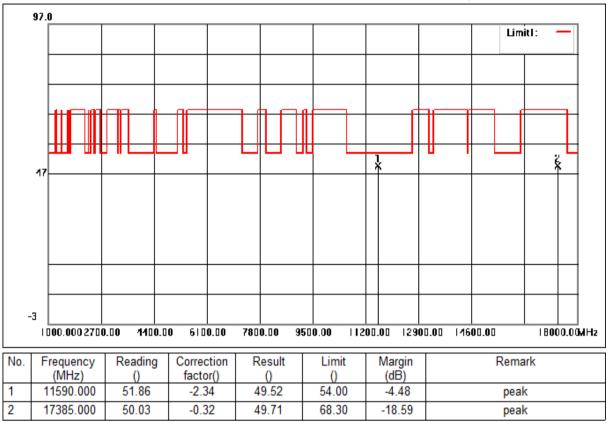
Mode:d; Polarization:Vertical; Modulation:ac; bandwidth:40MHz; Channel:High
