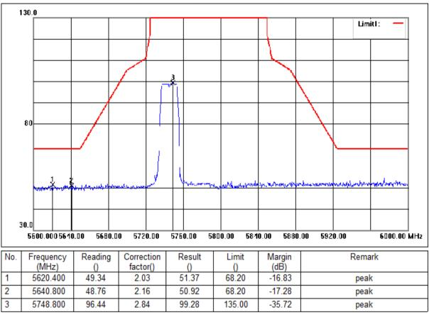
Mode:d; Polarization:Horizontal; Modulation:n; bandwidth:20MHz; Channel:Low
