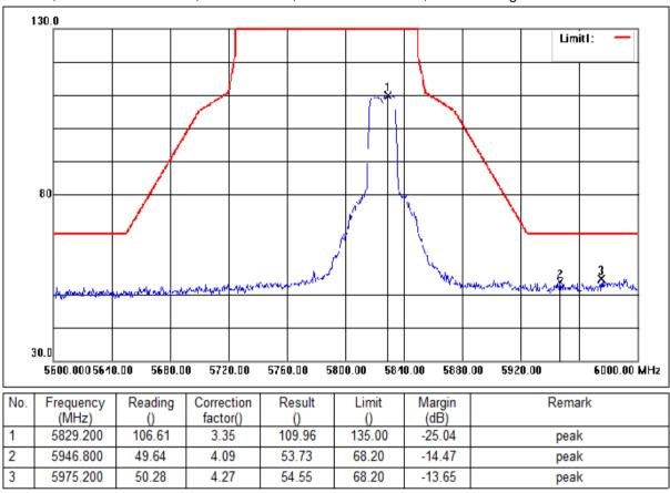
Mode:d; Polarization:Vertical; Modulation:n; bandwidth:20MHz; Channel:High
