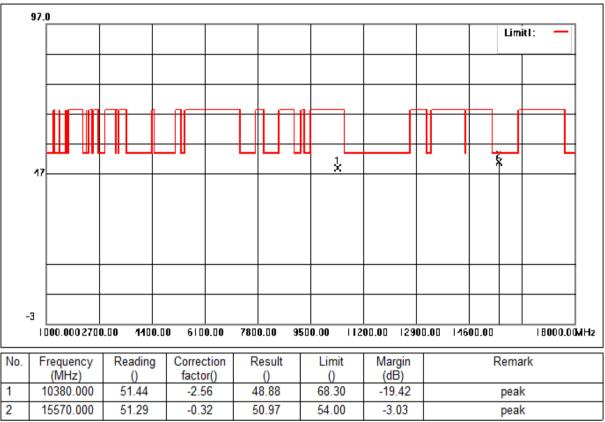
Mode:c; Polarization:Vertical; Modulation:ac; bandwidth:40MHz; Channel:Low
