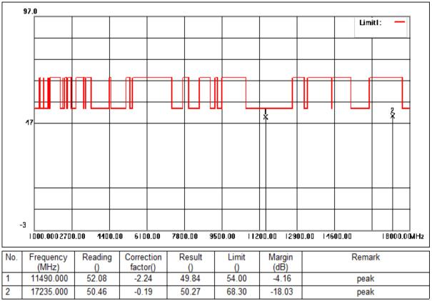
Mode:d; Polarization:Horizontal; Modulation:ac; bandwidth:20MHz; Channel:Low
