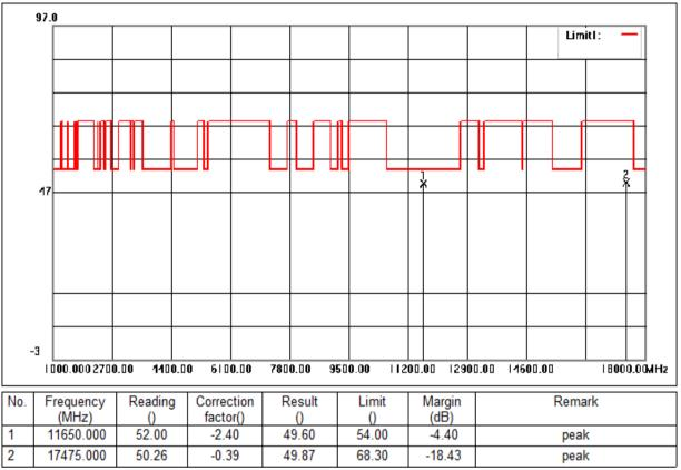
Mode:d; Polarization:Horizontal; Modulation:a; bandwidth:20MHz; Channel:High
