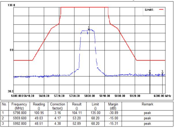
Mode:d; Polarization:Vertical; Modulation:n; bandwidth:40MHz; Channel:High
