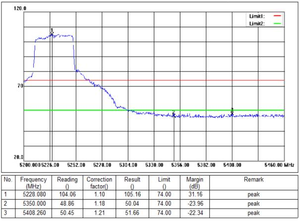
Mode:c; Polarization:Vertical; Modulation:c; bandwidth:40MHz; Channel:High
