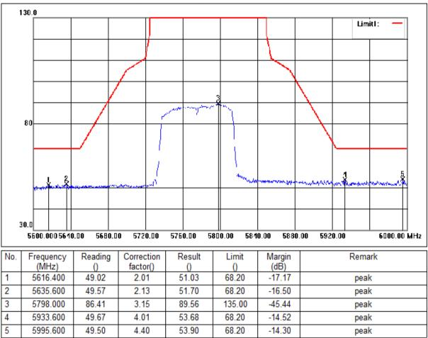
Mode:d; Polarization:Horizontal; Modulation:ac; bandwidth:80MHz; Channel:Low
