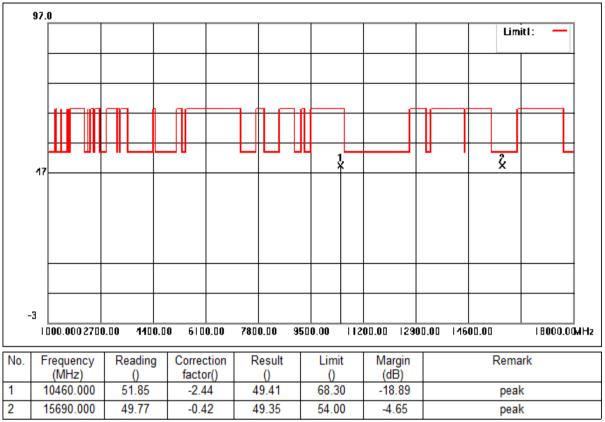
Mode:c; Polarization:Horizontal; Modulation:ac; bandwidth:40MHz; Channel:High
