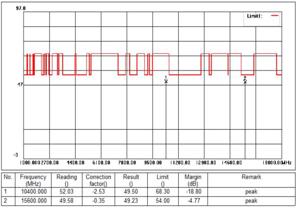
Mode:c; Polarization:Vertical; Modulation:a; bandwidth:20MHz; Channel:middle
