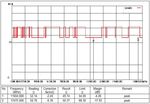
Mode:d; Polarization:Vertical; Modulation:a; bandwidth:20MHz; Channel:High
