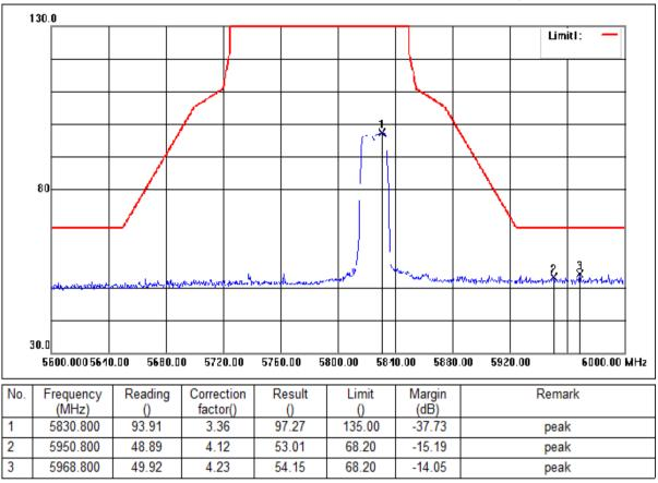
Mode:d; Polarization:Horizontal; Modulation:n; bandwidth:20MHz; Channel:High
