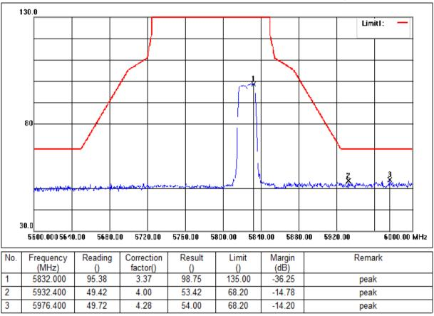
Mode:d; Polarization:Horizontal; Modulation:ac; bandwidth:20MHz; Channel:High
