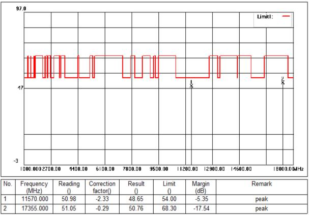
Mode:d; Polarization:Horizontal; Modulation:n; bandwidth:20MHz; Channel:middle
