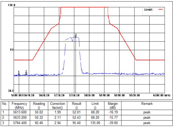
Mode:d; Polarization:Horizontal; Modulation:n; bandwidth:40MHz; Channel:Low
