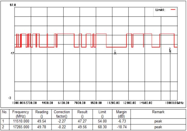
Mode:d; Polarization:Horizontal; Modulation:n; bandwidth:40MHz; Channel:Low
