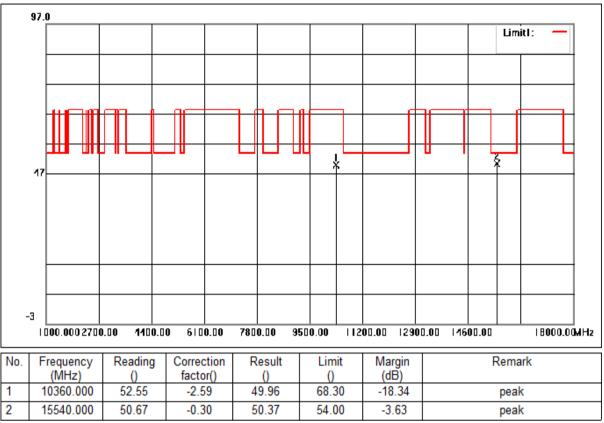
Mode:c; Polarization:Horizontal; Modulation:ac; bandwidth:20MHz; Channel:Low
