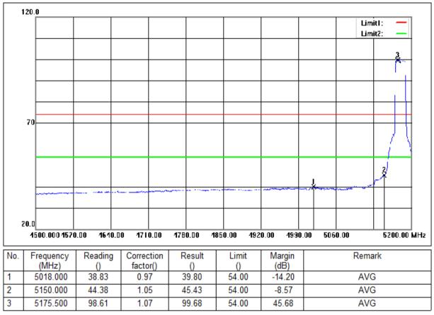
Mode:c; Polarization:Vertical; Modulation:c; bandwidth:20MHz; Channel:Low
