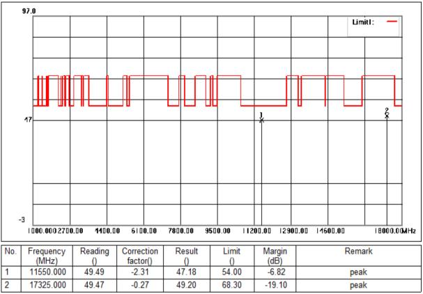
Mode:d; Polarization:Horizontal; Modulation:ac; bandwidth:80MHz; Channel:Low
