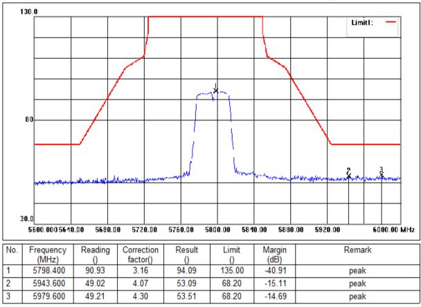
Mode:d; Polarization:Horizontal; Modulation:n; bandwidth:40MHz; Channel:High
