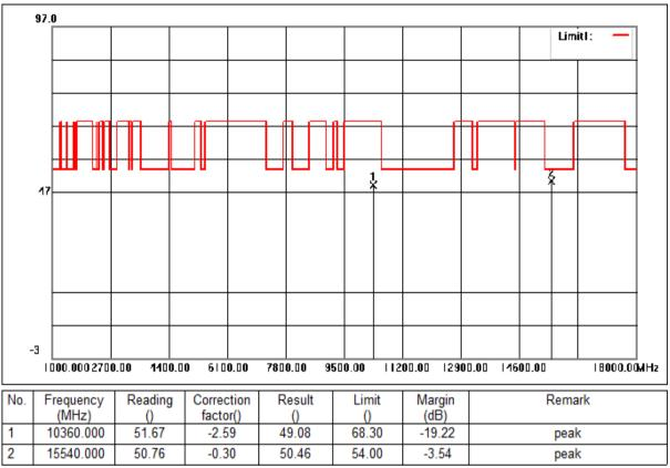
Mode:c; Polarization:Vertical; Modulation:n; bandwidth:20MHz; Channel:Low
