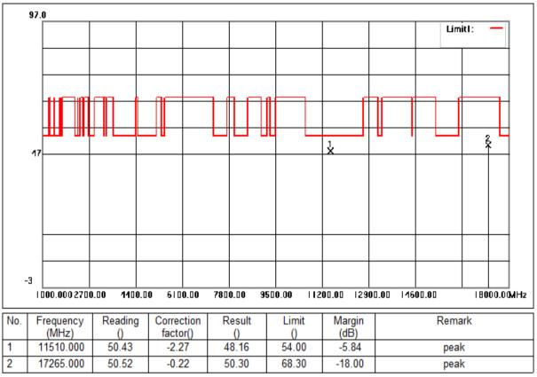
Mode:d; Polarization:Vertical; Modulation:n; bandwidth:40MHz; Channel:Low
