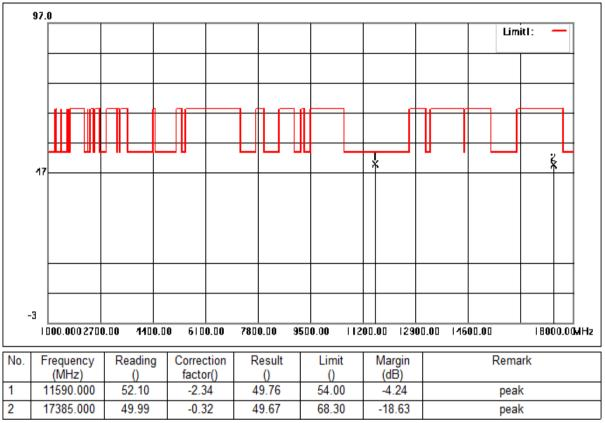
Mode:d; Polarization:Horizontal; Modulation:n; bandwidth:40MHz; Channel:High
