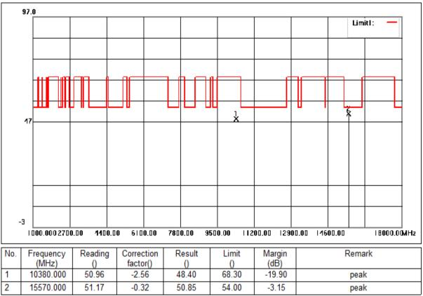
Mode:c; Polarization:Vertical; Modulation:n; bandwidth:40MHz; Channel:Low
