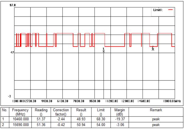
Mode:c; Polarization:Vertical; Modulation:ac; bandwidth:40MHz; Channel:High
