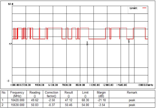
Mode:c; Polarization:Horizontal; Modulation:ac; bandwidth:80MHz; Channel:Low
