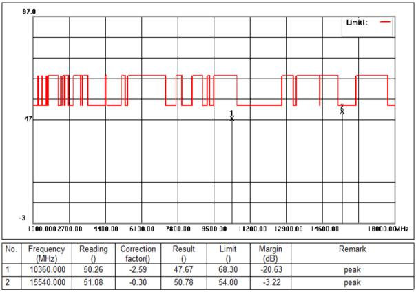
Mode:c; Polarization:Vertical; Modulation:a; bandwidth:20MHz; Channel:Low
