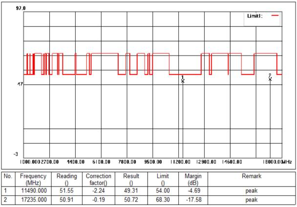
Mode:d; Polarization:Vertical; Modulation:a; bandwidth:20MHz; Channel:Low
