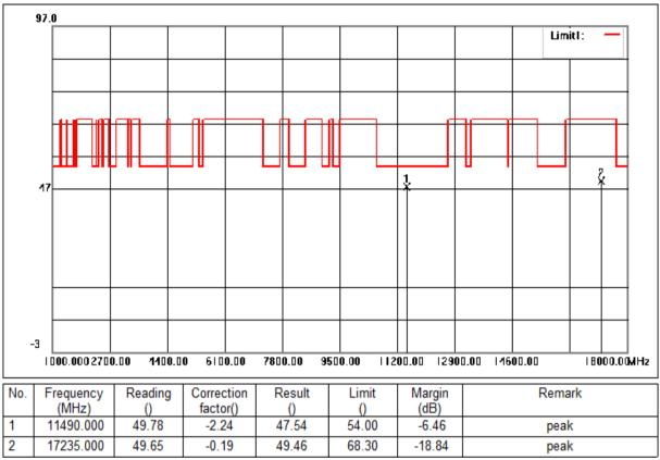
Mode:d; Polarization:Vertical; Modulation:ac; bandwidth:20MHz; Channel:Low
