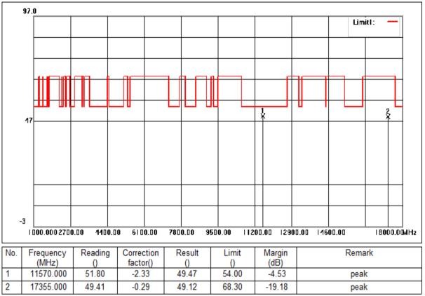
Mode:d; Polarization:Horizontal; Modulation:ac; bandwidth:20MHz; Channel:middle
