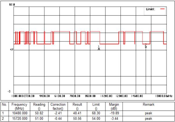
Mode:c; Polarization:Horizontal; Modulation:n; bandwidth:20MHz; Channel:High
