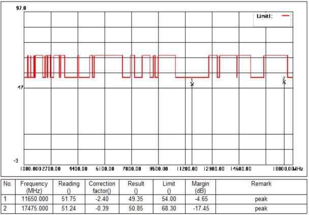
Mode:d; Polarization:Horizontal; Modulation:n; bandwidth:20MHz; Channel:High
