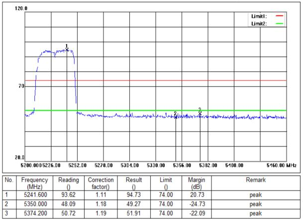
Mode:c; Polarization:Horizontal; Modulation:n; bandwidth:40MHz; Channel:High
