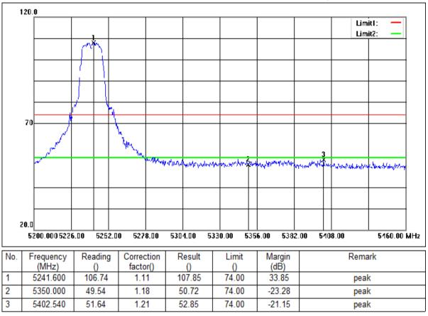
Mode:c; Polarization:Vertical; Modulation:n; bandwidth:20MHz; Channel:High
