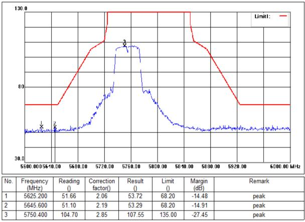
Mode:d; Polarization:Vertical; Modulation:ac; bandwidth:40MHz; Channel:Low
