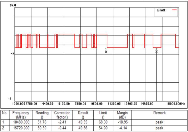
Mode:c; Polarization:Vertical; Modulation:a; bandwidth:20MHz; Channel:High
