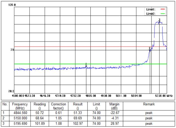
Mode:c; Polarization:Vertical; Modulation:n; bandwidth:40MHz; Channel:Low
