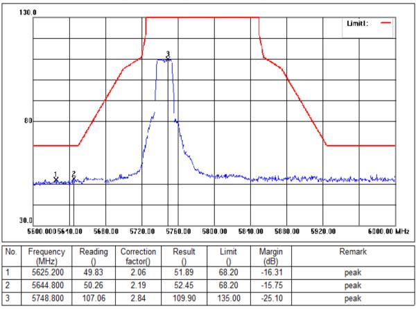
Mode:d; Polarization:Vertical; Modulation:n; bandwidth:20MHz; Channel:Low
