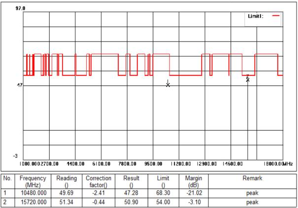
Mode:c; Polarization:Vertical; Modulation:ac; bandwidth:20MHz; Channel:High
