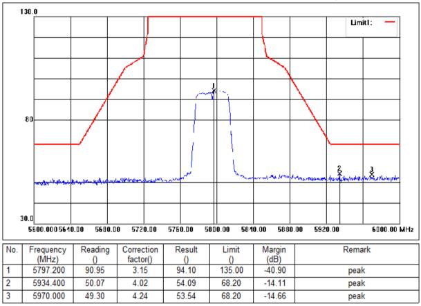
Mode:d; Polarization:Horizontal; Modulation:ac; bandwidth:40MHz; Channel:High
