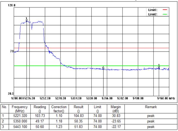
Mode:c; Polarization:Vertical; Modulation:n; bandwidth:40MHz; Channel:High
