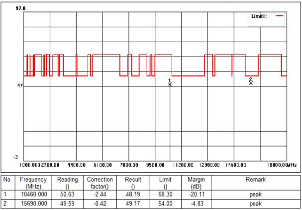
Mode:c; Polarization:Vertical; Modulation:n; bandwidth:40MHz; Channel:High
