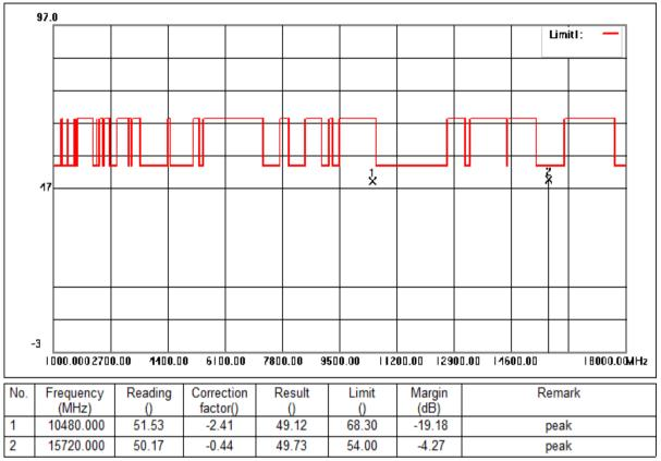
Mode:c; Polarization:Horizontal; Modulation:ac; bandwidth:20MHz; Channel:High
