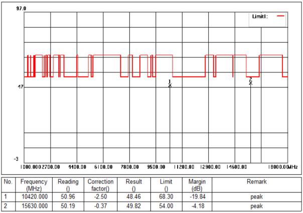
Mode:c; Polarization:Vertical; Modulation:ac; bandwidth:80MHz; Channel:Low
