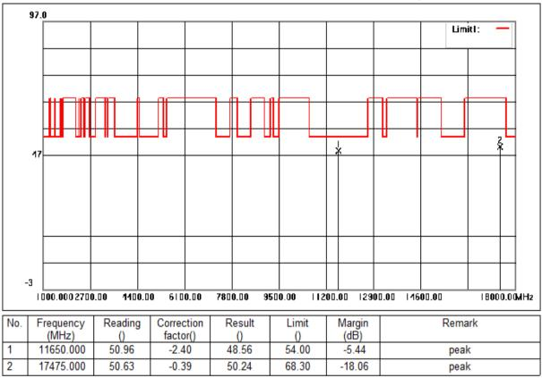
Mode:d; Polarization:Vertical; Modulation:ac; bandwidth:20MHz; Channel:High
