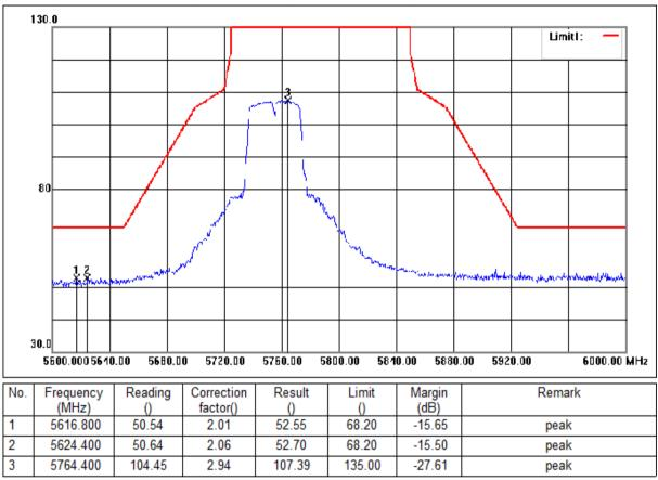
Mode:d; Polarization:Vertical; Modulation:n; bandwidth:40MHz; Channel:Low
