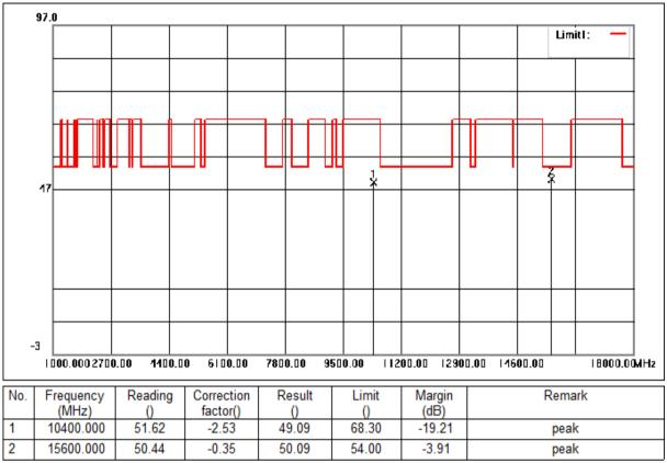
Mode:c; Polarization:Horizontal; Modulation:a; bandwidth:20MHz; Channel:middle
