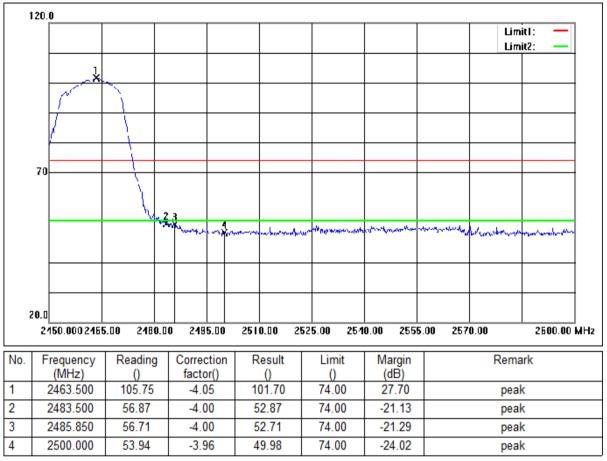
Mode:b; Polarization:Vertical; Modulation:n; bandwidth:20MHz; Channel:High
