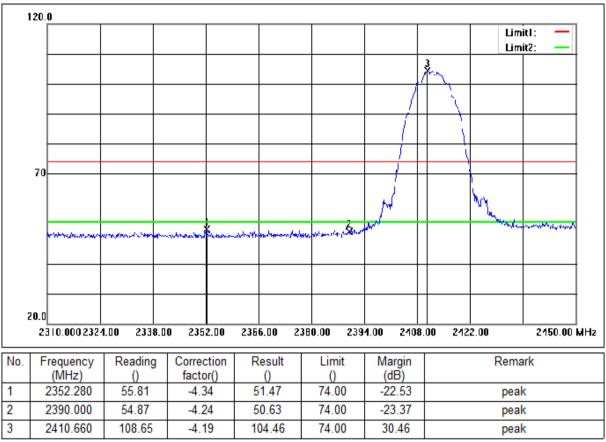
Mode:b; Polarization:Vertical; Modulation:b; bandwidth:20MHz; Channel:Low
