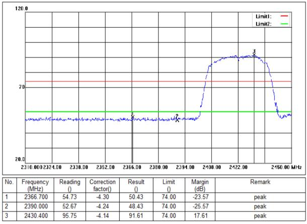
Mode:b; Polarization:Horizontal; Modulation:n; bandwidth:40MHz; Channel:Low
