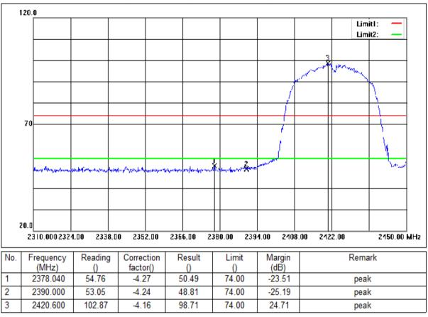
Mode:b; Polarization:Vertical; Modulation:n; bandwidth:40MHz; Channel:Low
