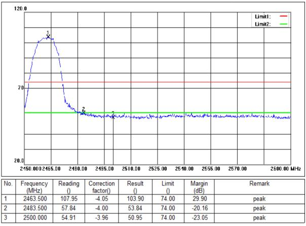
Mode:b; Polarization:Vertical; Modulation:b; bandwidth:20MHz; Channel:High
