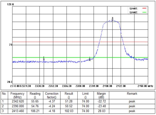
Mode:b; Polarization:Vertical; Modulation:n; bandwidth:20MHz; Channel:Low
