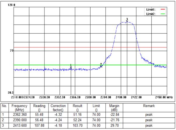
Mode:b; Polarization:Vertical; Modulation:g; bandwidth:20MHz; Channel:Low
