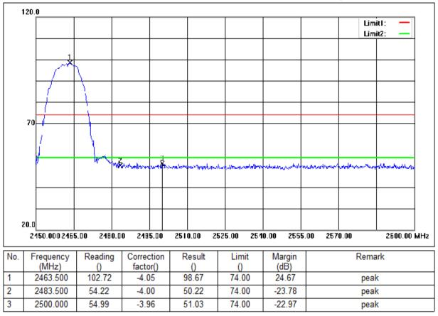
Mode:b; Polarization:Horizontal; Modulation:b; bandwidth:20MHz; Channel:High
