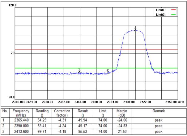
Mode:b; Polarization:Horizontal; Modulation:n; bandwidth:20MHz; Channel:Low
