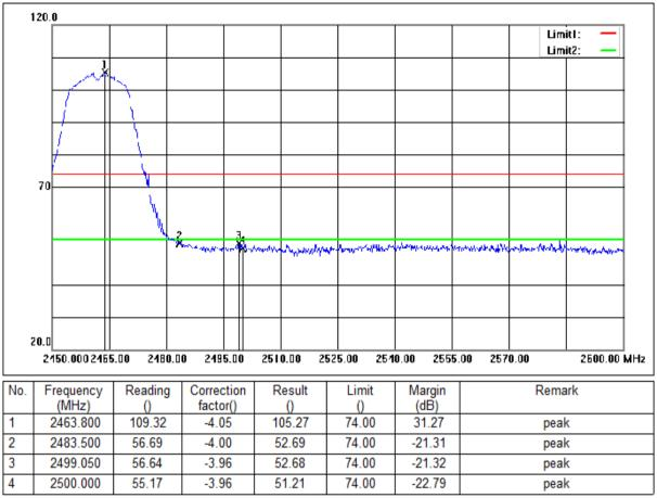
Mode:b; Polarization:Vertical; Modulation:g; bandwidth:20MHz; Channel:High
