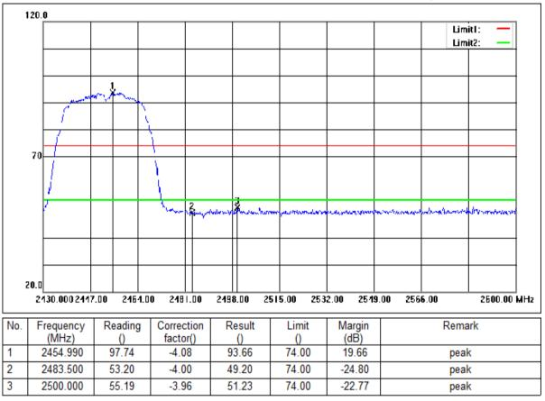
Mode:b; Polarization:Horizontal; Modulation:n; bandwidth:40MHz; Channel:High
