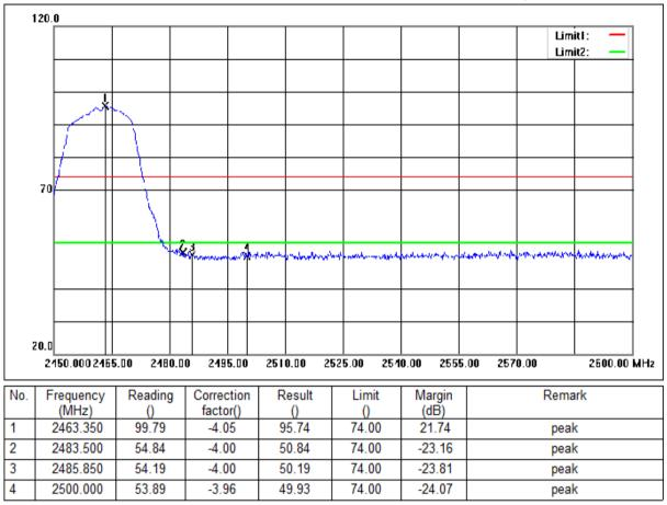
Mode:b; Polarization:Horizontal; Modulation:n; bandwidth:20MHz; Channel:High
