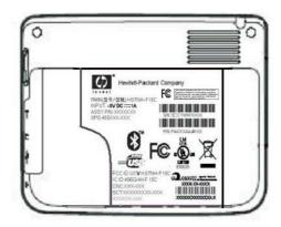
The FCC ID and DoC Label will be placed on the equipment as shown in the photograph below.
