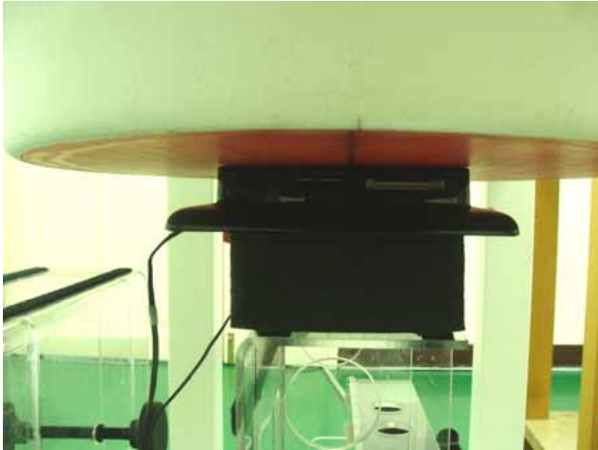
Bottom of the DUT with 0 cm gap to flat phantom (DUT with Earphone)
