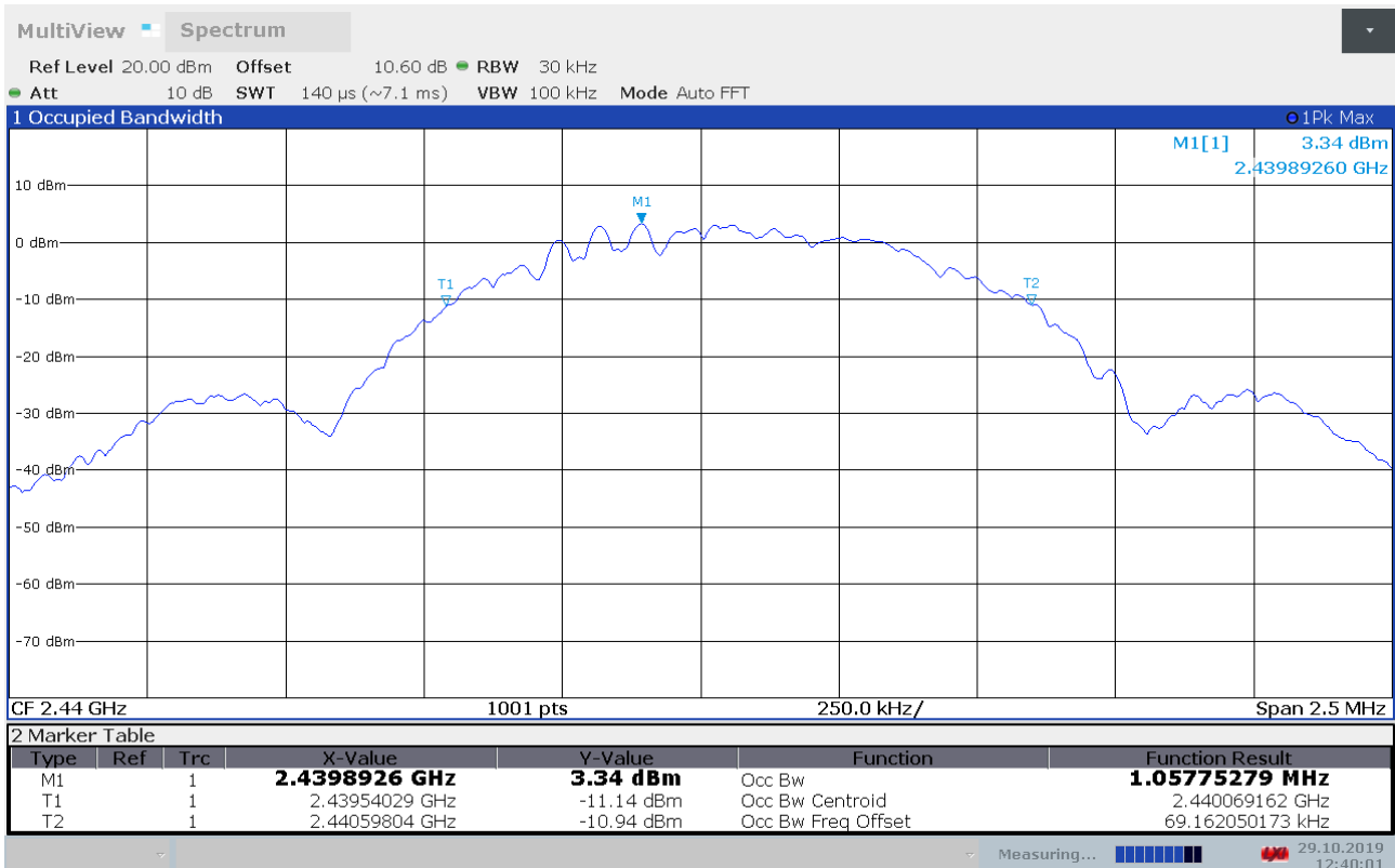
Occupied Bandwidth, 99%, 2440 MHz
