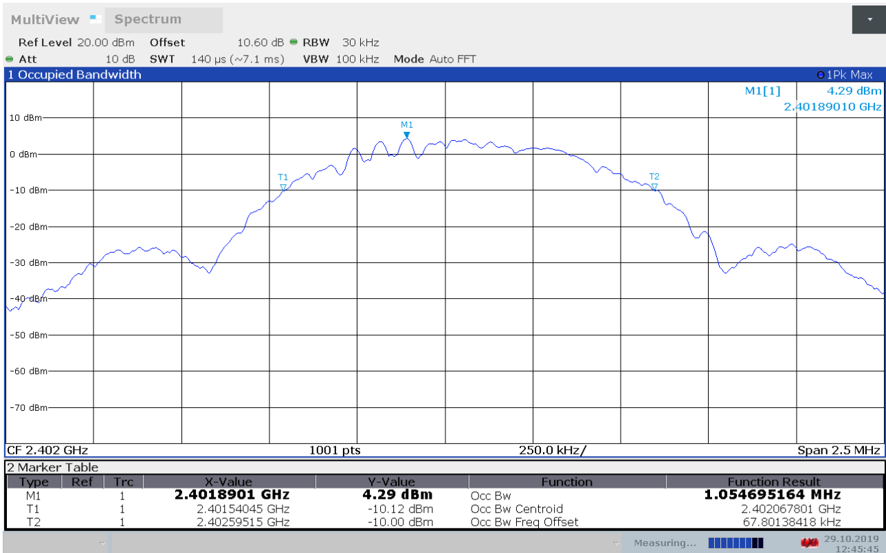
Occupied Bandwidth, 99%, 2402 MHz
