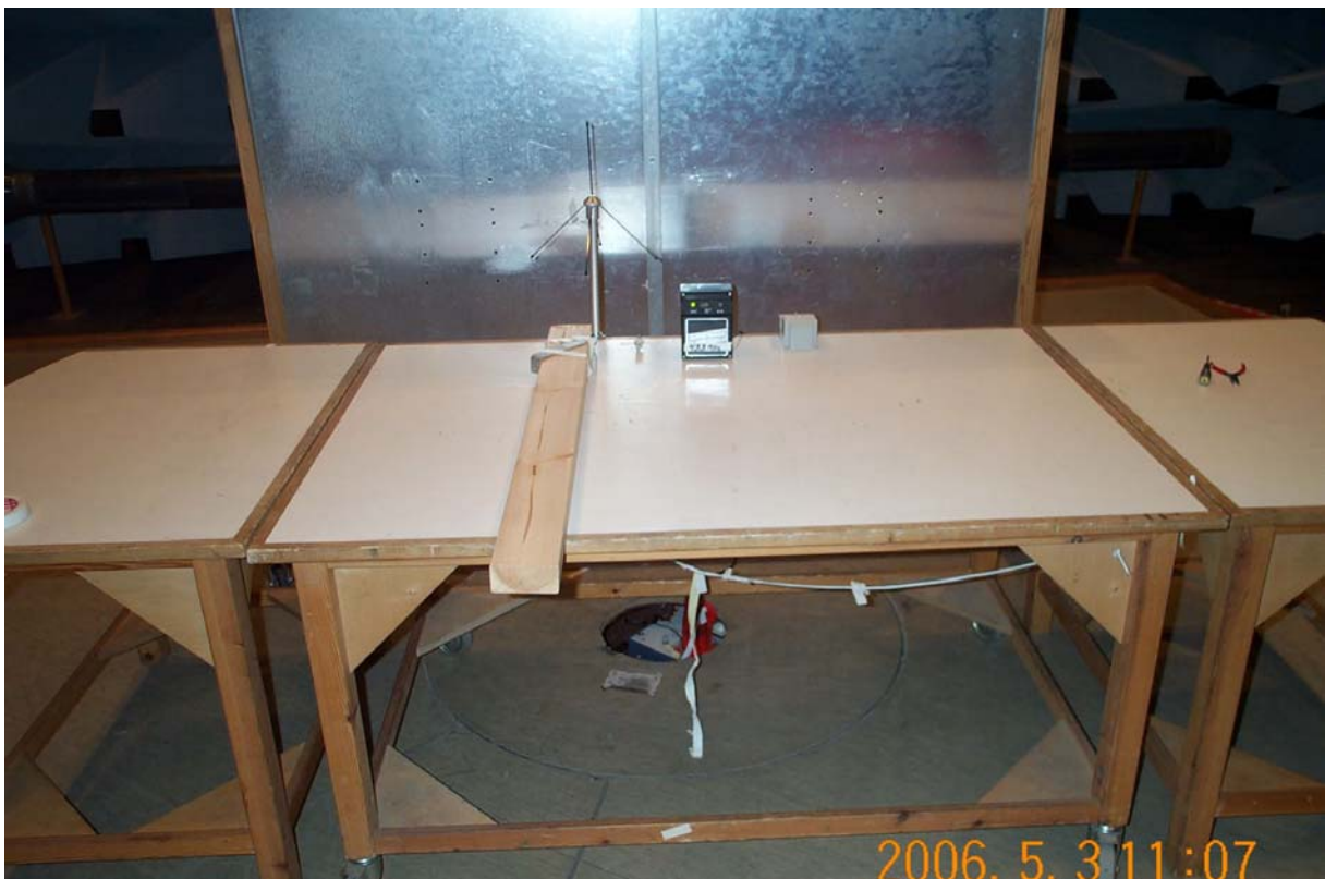
Photo A2.4 Test setup for conducted emission.
