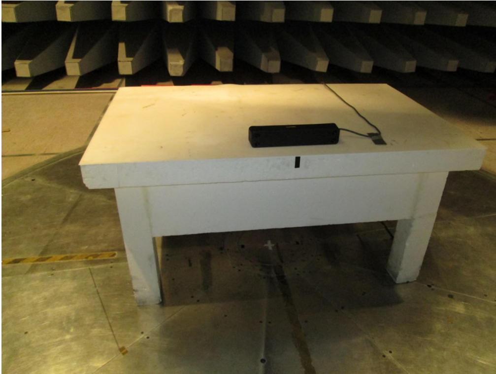
Photo 4.1.1 Test setup regarding measurement of radio frequency electromagnetic field. Preview measurement in shielded room
