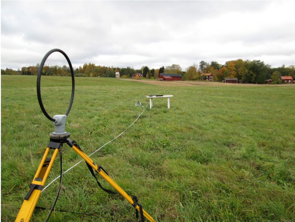
Photo 4.1.3 Test setup regarding measurement of radio frequency electromagnetic field. Verification measurement outdoors. 10 m measurement distance.
