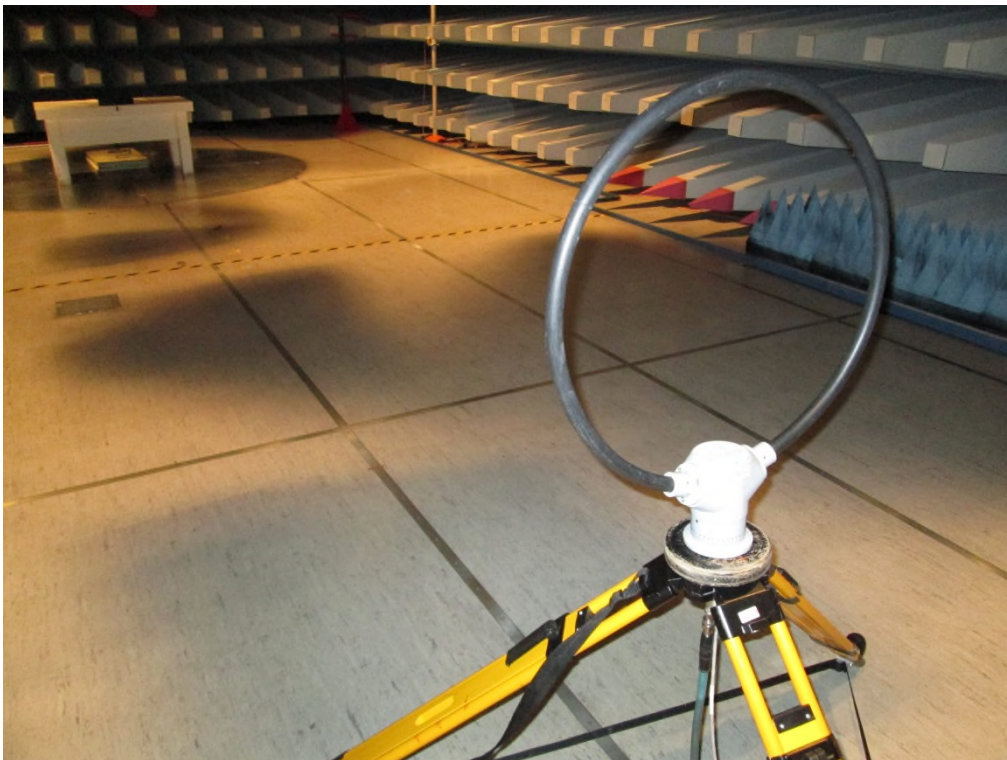
Photo 4.1.2 Test setup regarding measurement of radio frequency electromagnetic field. Preview measurement in shielded room
