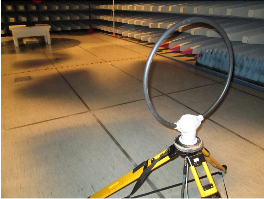
Photo 4.4.1 Test setup regarding measurement of occupied bandwidth.
