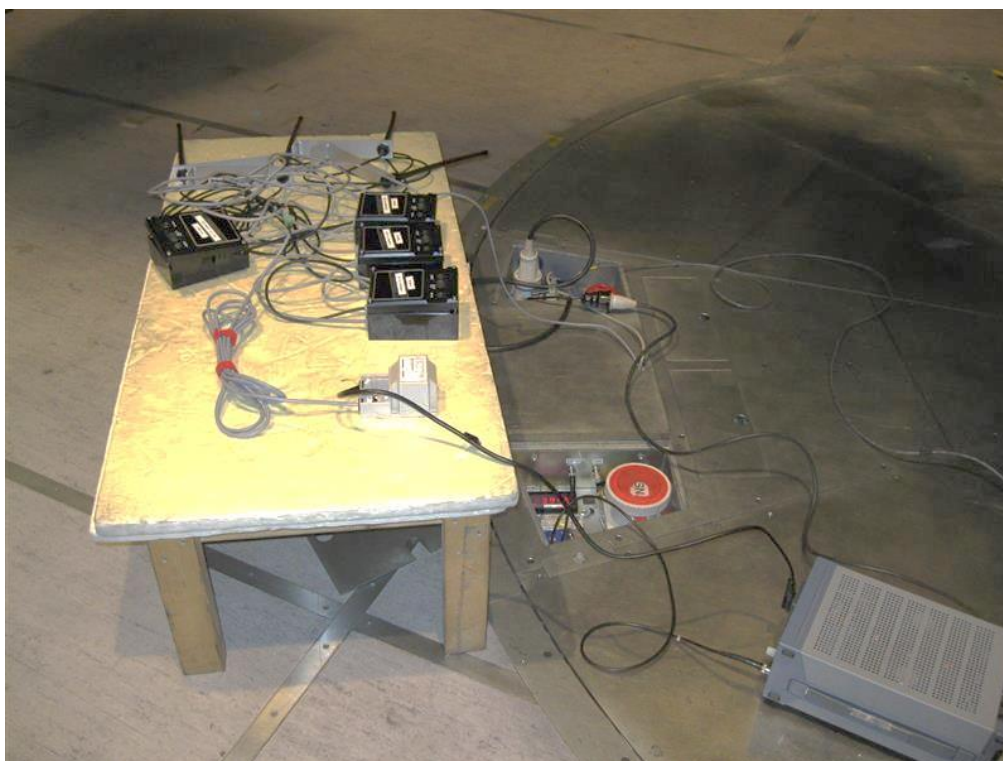
Test setup regarding measurement of radio frequency voltage on mains.
