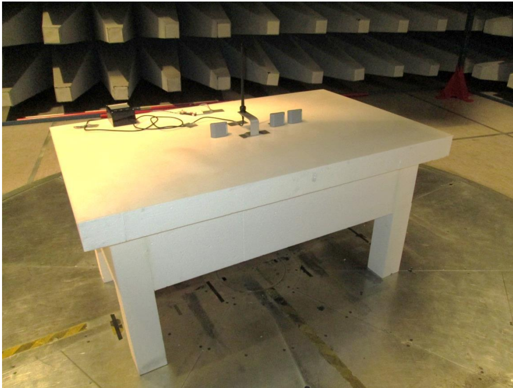
Test setup regarding measurement of peak output field strength of fundamental.
