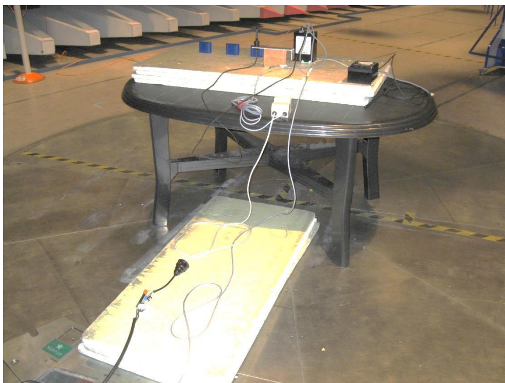
Test setup regarding measurement of radio frequency electromagnetic field < 1 GHz..
