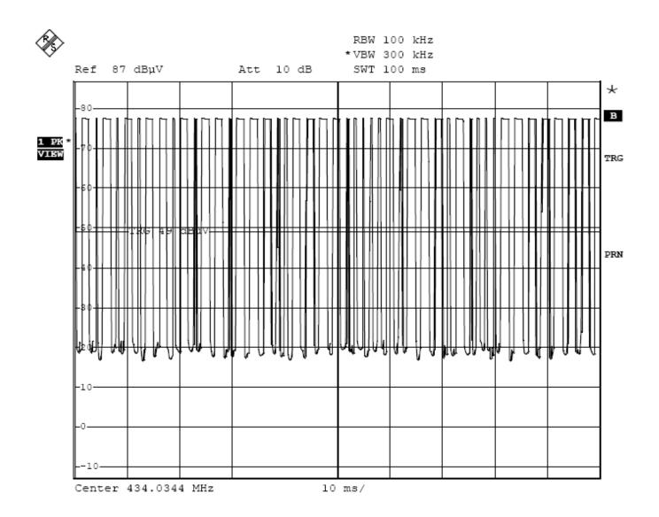
The graph shows the pattern of coding during the signal transmission. Hence the total time of one period is 100ms.
