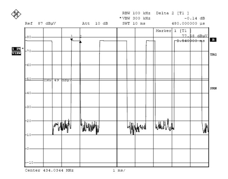
The graph show the duration of short 'on' signal. From marker 1 to marker 2, duration is 0.48ms.
