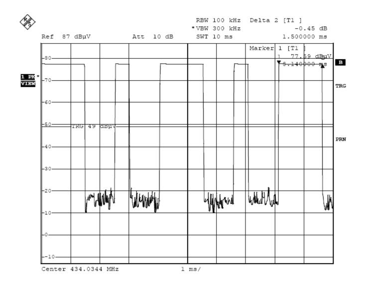
The graph show the duration of long 'on' signal. From marker 1 to marker 2, duration is 1.5ms.
