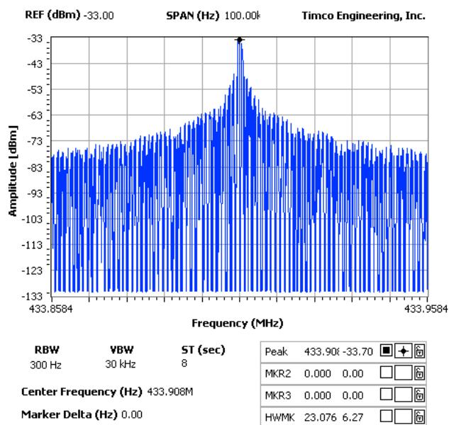
**METHOD OF MEASUREMENT:** A small sample of the transmitter output was fed into the spectrum analyzer and the following plot was generated. The vertical scale is set to 10 dB per division: the horizontal scale is set to 100 kHz per division.
