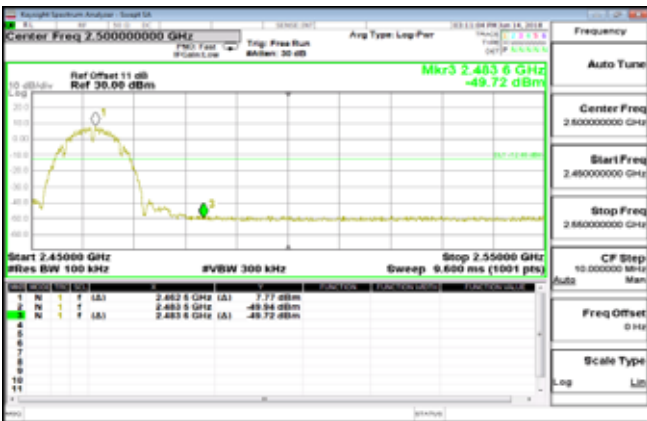
802.11b: Band Edges Test Data CH-High
