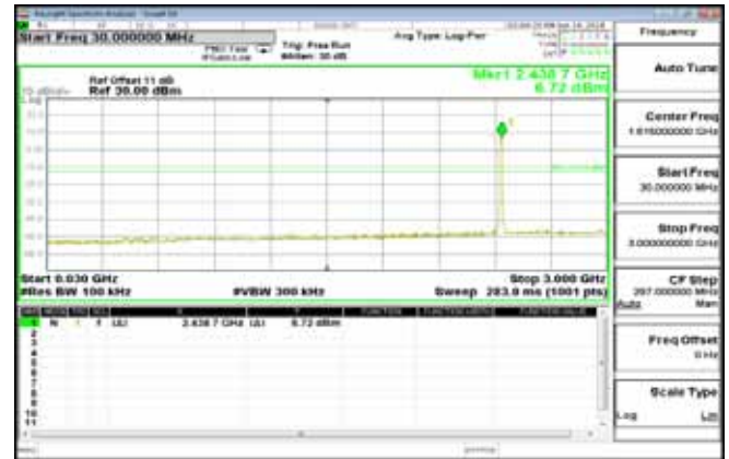
802.11b: Spurious Emission Test Data CH-Mid
