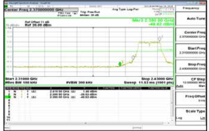
802.11g: Band Edges Test Data CH-High
