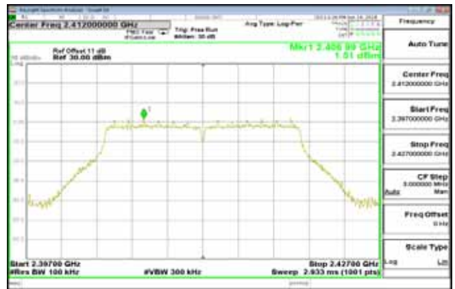
802.11g Reference Level of Emission Limit(CH-Mid)
