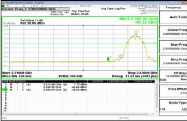
802.11b: Band Edges Test Data CH-High
