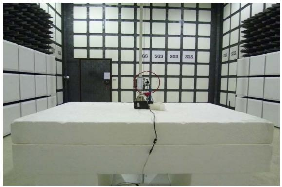
Radiated Emission Set up Photos (Below 1GHz)
