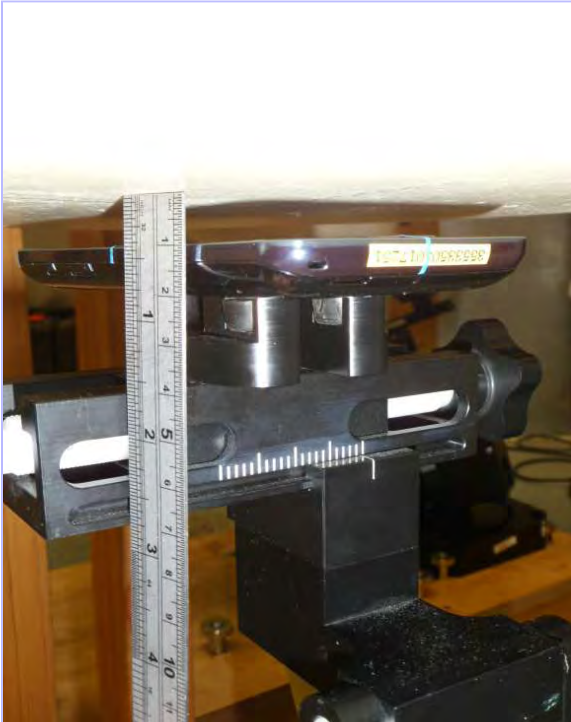
PHT/92315JD03A/010: Front of EUT Antenna Retracted Facing Phantom at 10mm
