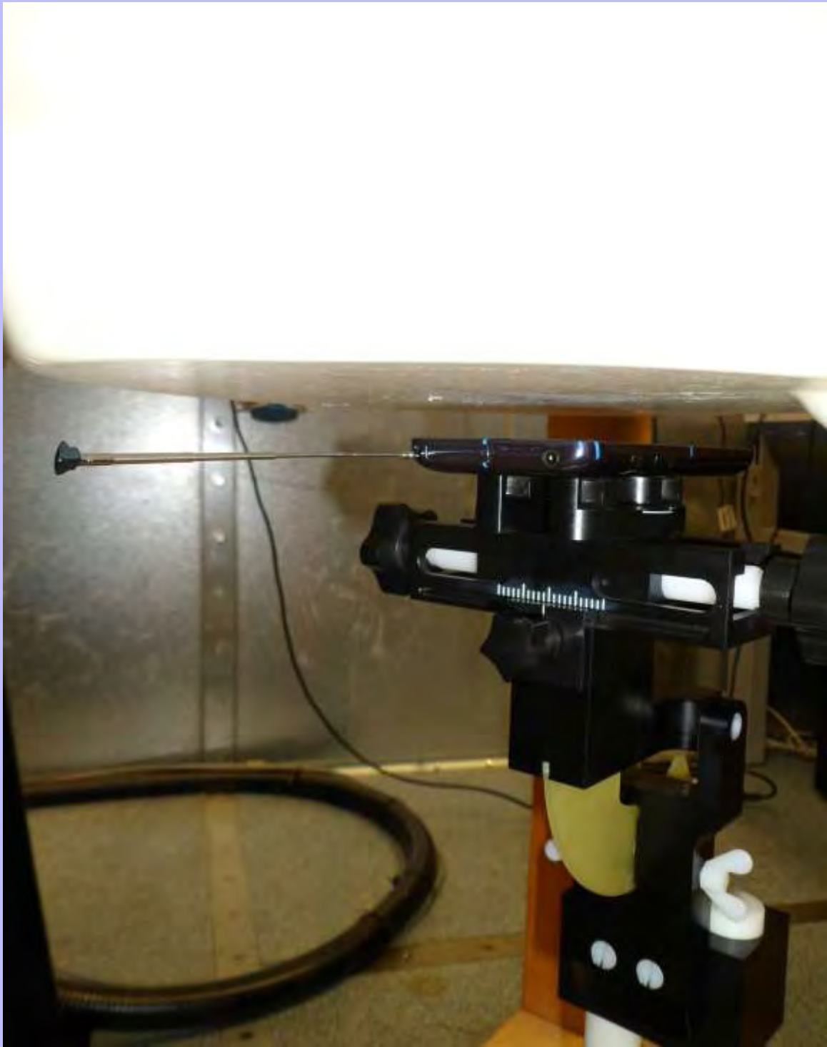
PHT/92315JD03A/013: Front of EUT Antenna Extended Facing Phantom at 15mm
