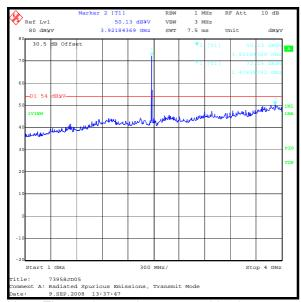
Note: The carrier can be seen on this plot at 2480MHz
