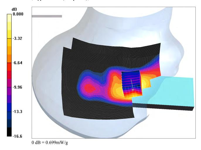
Communication System: PCS 1900; Frequency: 1879.8 MHz; Duty Cycle: 1:8.3
