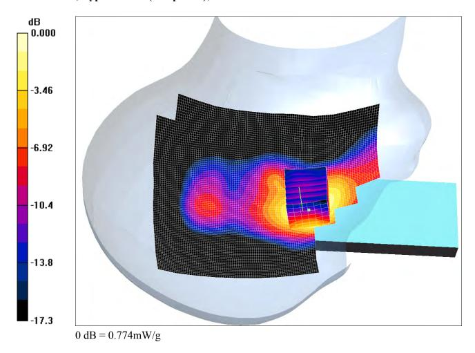
Communication System: PCS 1900; Frequency: 1909.8 MHz; Duty Cycle: 1:8.3
