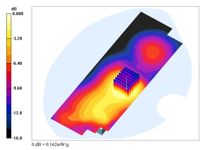
Communication System: GPRS 1900; Frequency: 1879.8 MHz; Duty Cycle: 1:4
