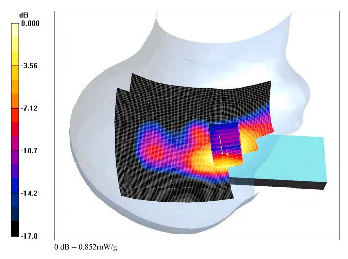
Communication System: PCS 1900; Frequency: 1850.2 MHz; Duty Cycle: 1:8.3
