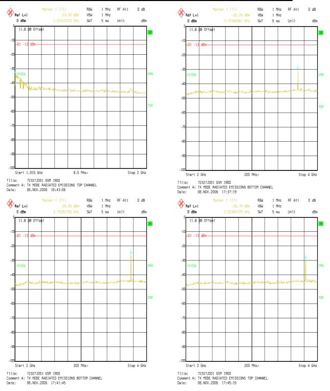
Note: These plots are pre-scans and for indication purposes only. For final measurements, see accompanying tables. The Plot with the emission at 3.7635 GHz incorrectly states Bottom Channel, when it was tested on the Top Channel.
