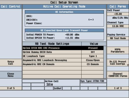
Figure 7: RB Test Mode Settings
