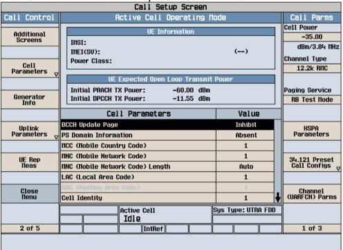
**Figure 5: Cell Parameters**
