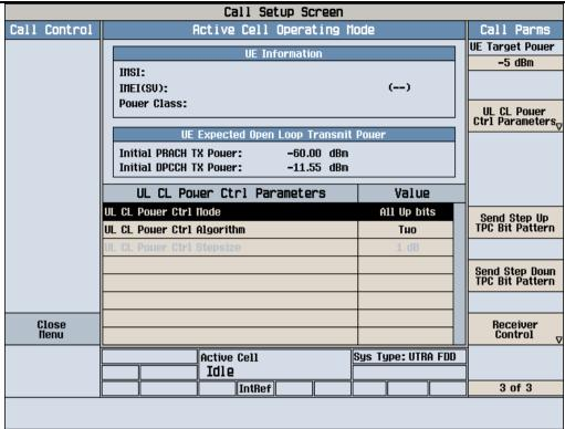
Figure 4: UL CL Power Ctrl Parameters
